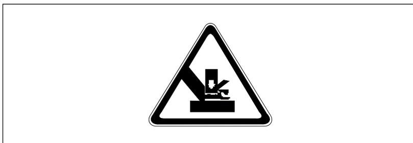
Figure 2-6. The pinching hazard label.
