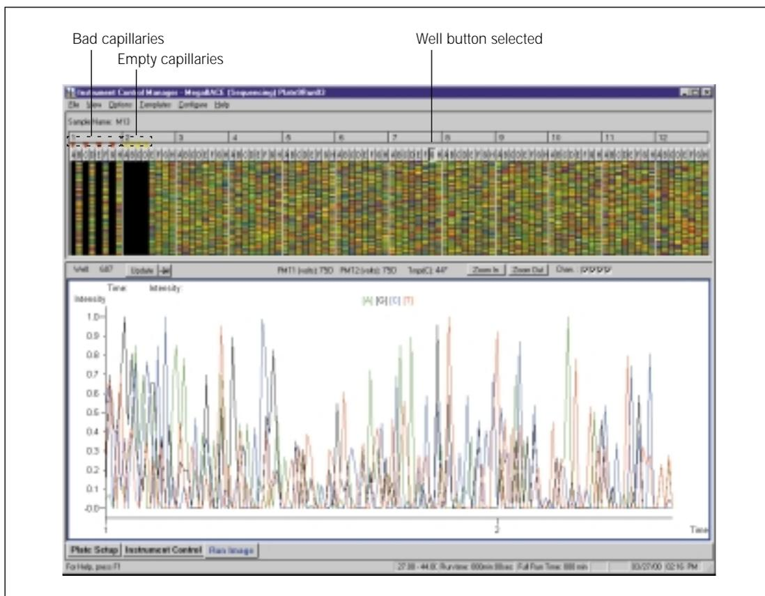
**Figure 5-6.** The Run Image window for a sequencing run. Empty capillaries are indicated by yellow arrows above the well buttons, and bad capillaries are indicated by red arrows above the well buttons.
