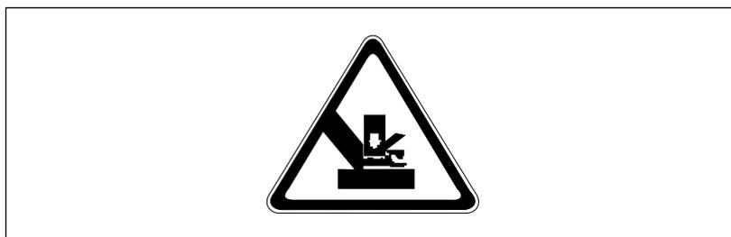
Figure 2-6. The pinching hazard label.
