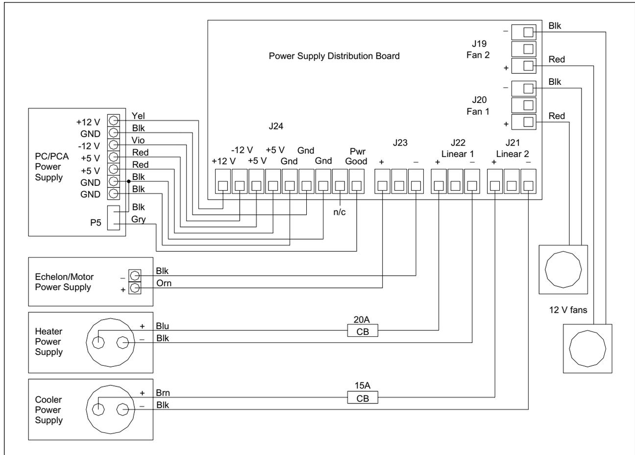
Figure 5-7. Power Supply Box DC Distribution Block Diagram (Four-Supply Model).
