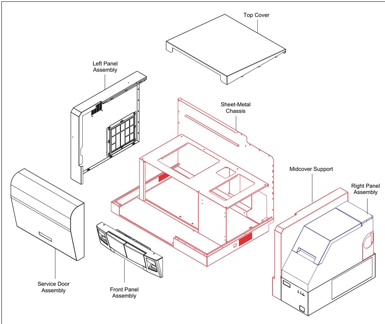
Figure 4-2. Enclosure Assembly.
