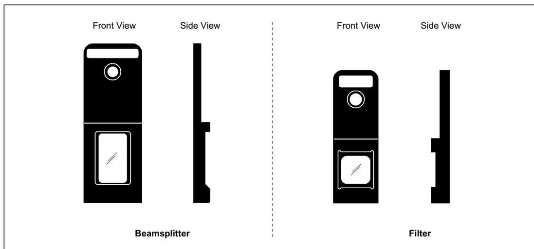
Figure 3-1. Emission Beamsplitter and Filter.
