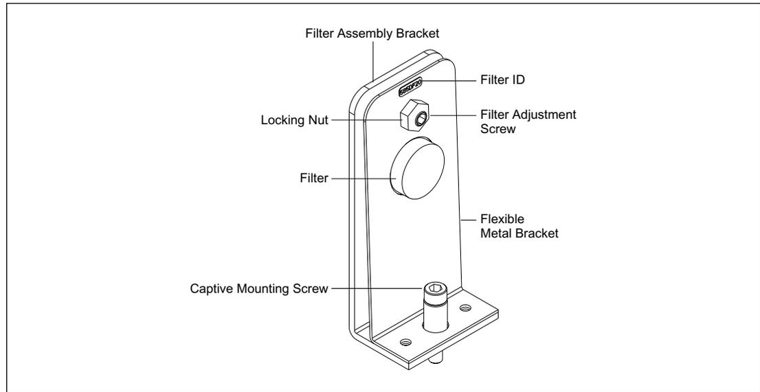
Figure 4-21. Laser Line Filter Assembly.
