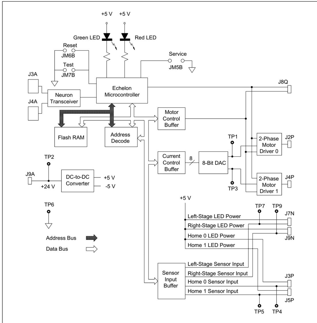
Figure 5-31. SCAN Board Block Diagram.
