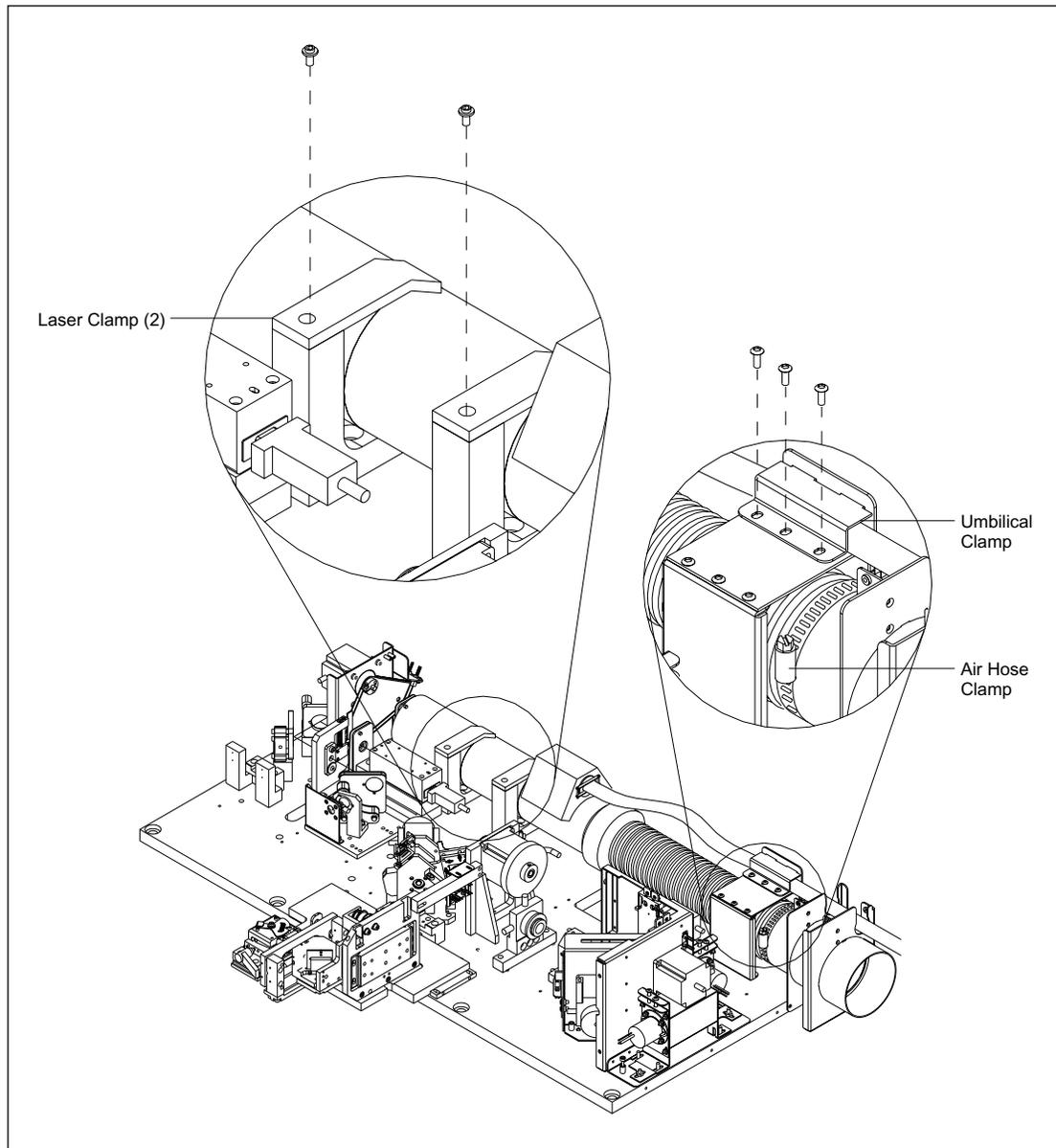
Figure 9-43. Blue Laser Mounting.
