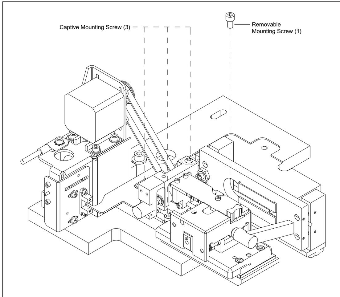
Figure 9-55. Focus Assembly Mounting.
