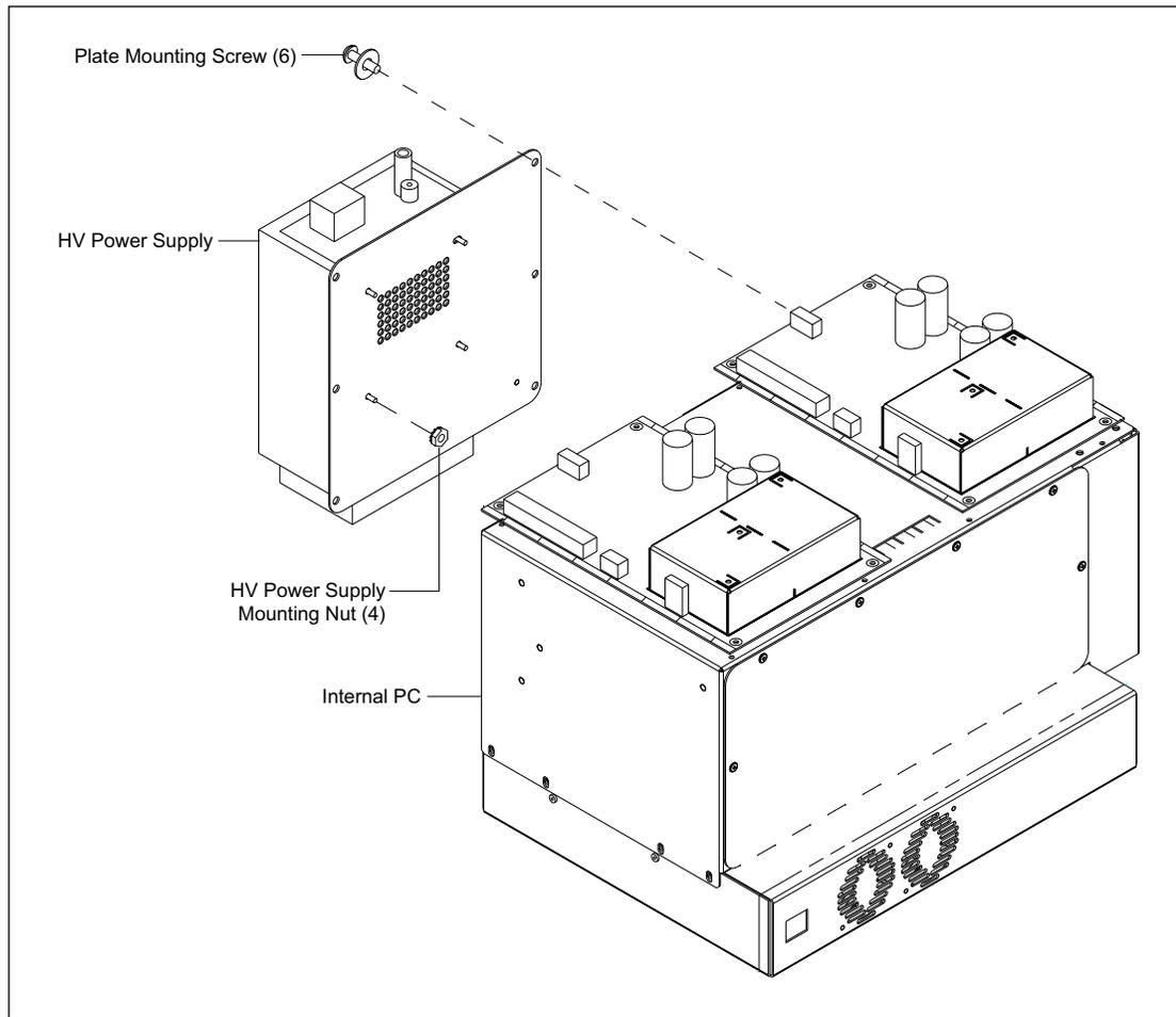
Figure 9-30. HV Power Supply Mounting.
