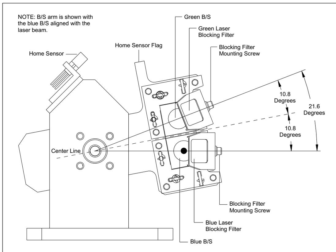
Figure 4-28. Primary Beamsplitter Arm Assembly.
