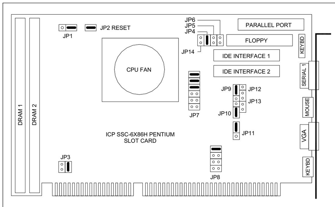
Figure 5-20. CPU Component Layout Diagram.
