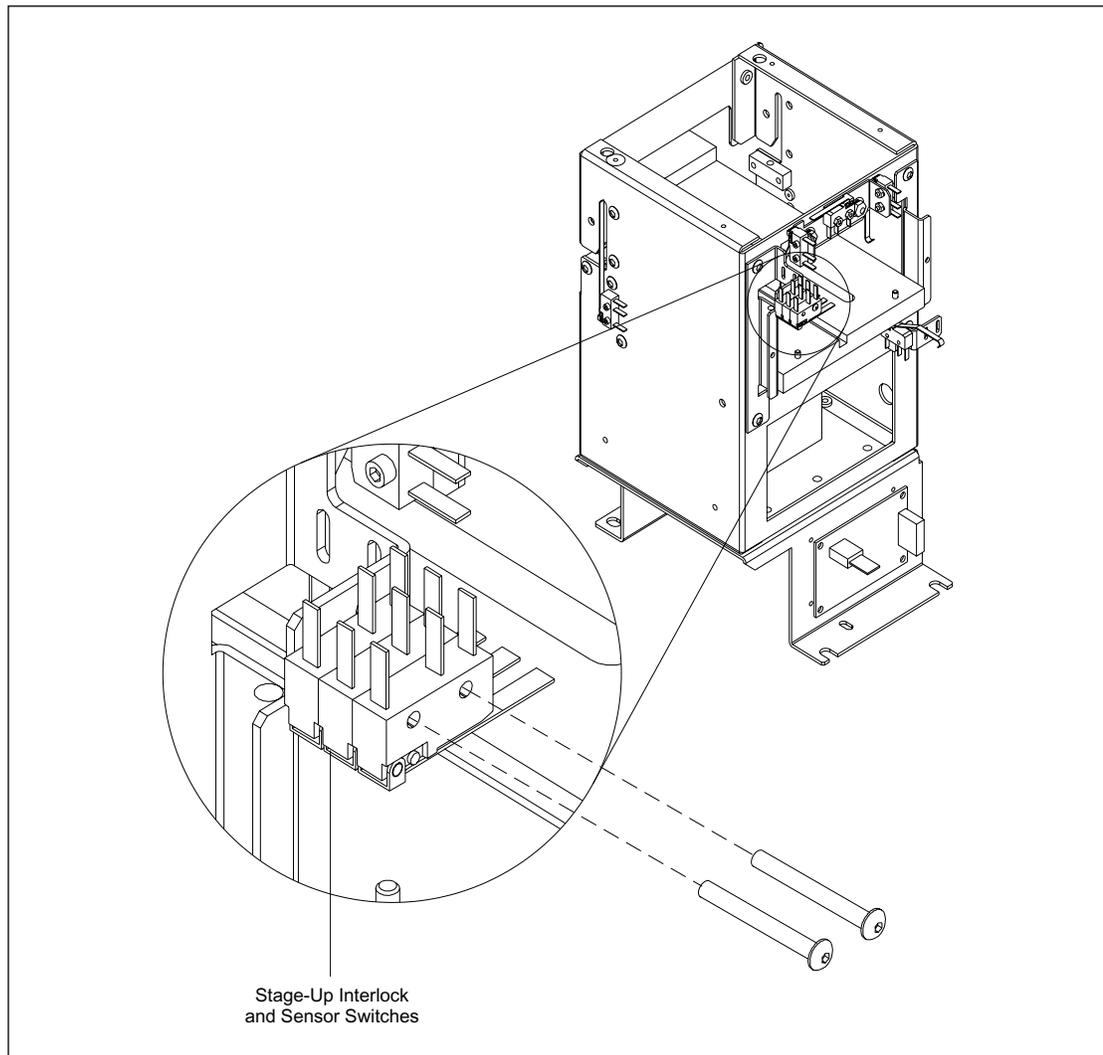
Figure 9-70. Cathode Stage-Up Interlock and Sensor Switch Mounting.
