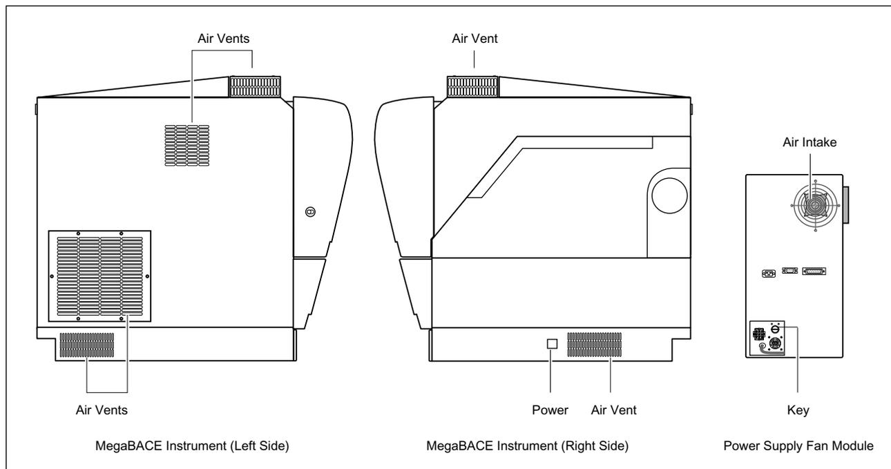
Figure 6-15. Instrument Airflow Openings.
