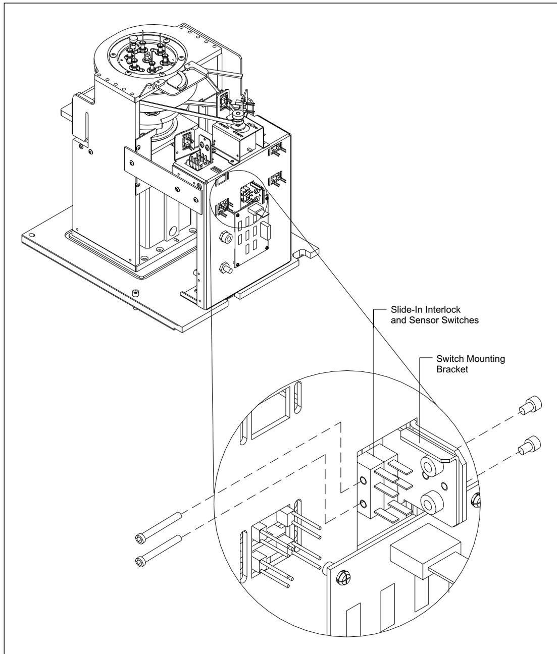
Figure 9-89. Anode Slide-In Interlock and Sensor Switch Mounting.
