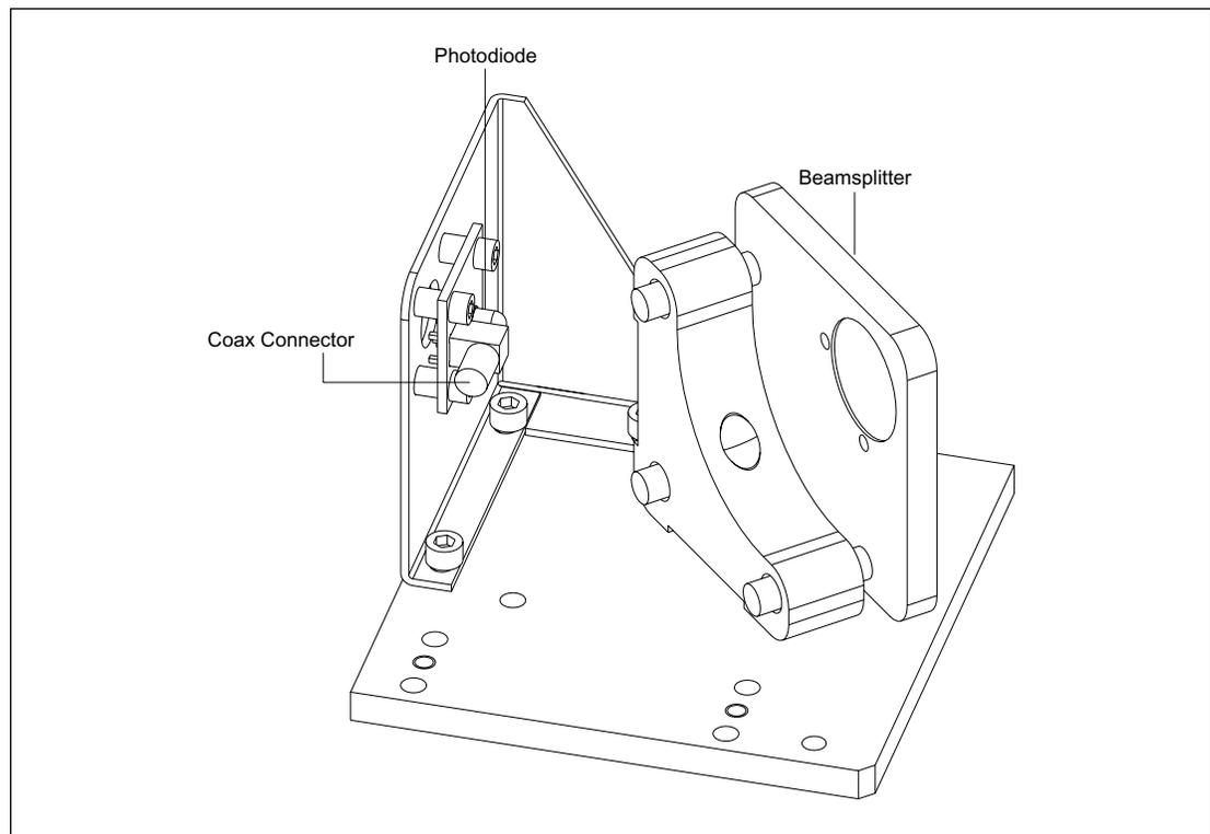
Figure 3-15. Capillary Detection Optics.
