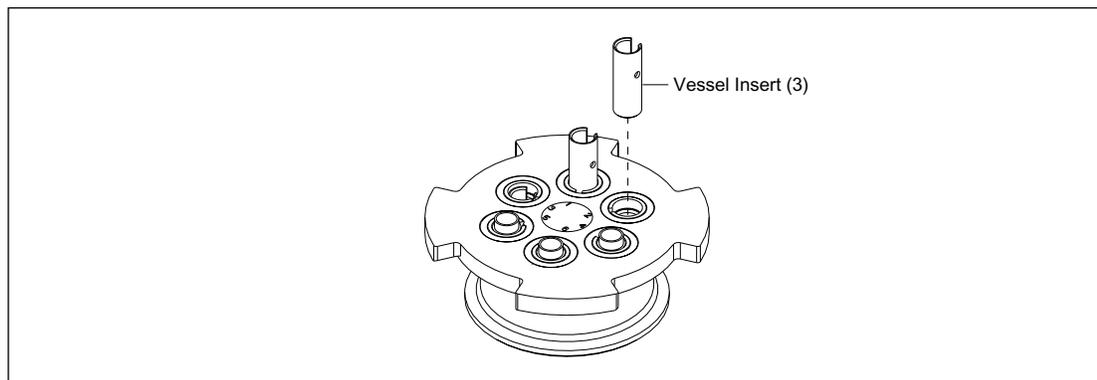
Figure 8-11. Anode Reservoir Holder.
