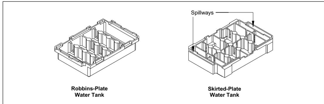
Figure 8-14. The Robbins Plate and the Skirted Plate.
