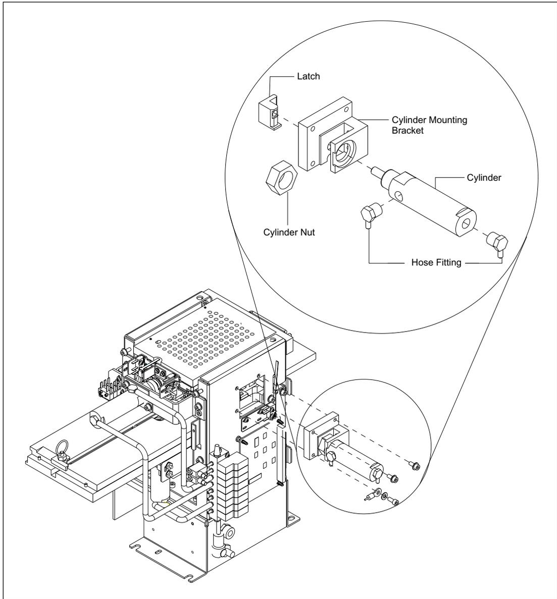
Figure 9-79. Indexer X-Position Actuator Mounting (MB 2000).
