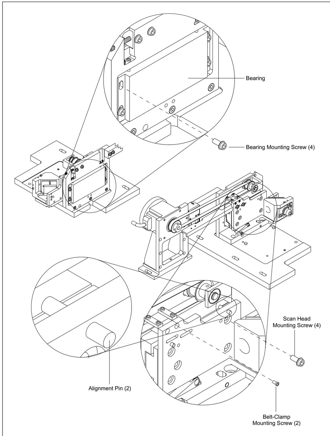
Figure 9-54. Scan Head Bearing Mounting.
