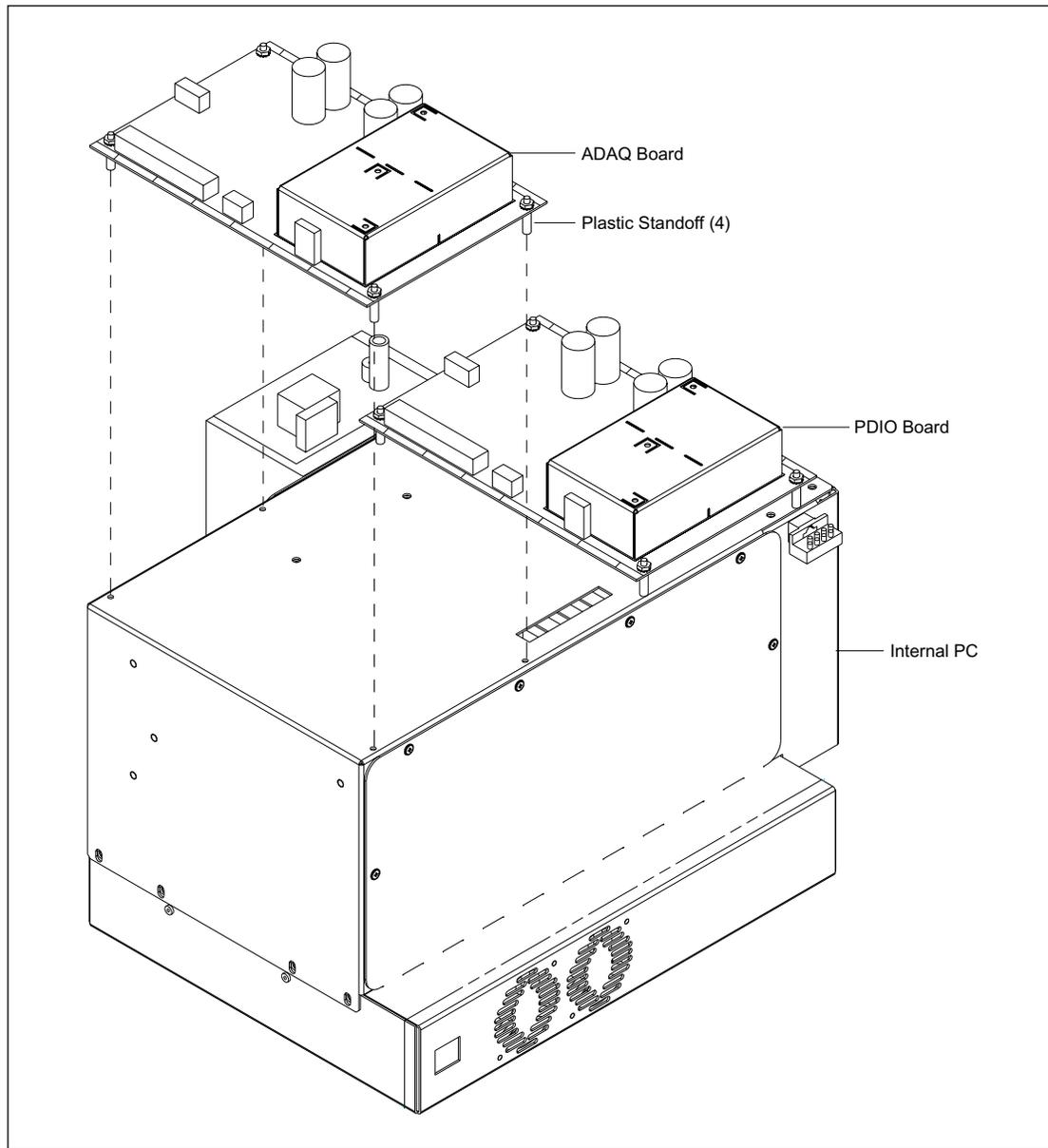
Figure 9-27. ADAQ Board Mounting.
