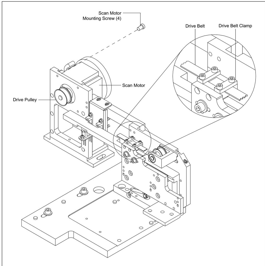
Figure 9-52. Scan Head Drive Motor Mounting.
