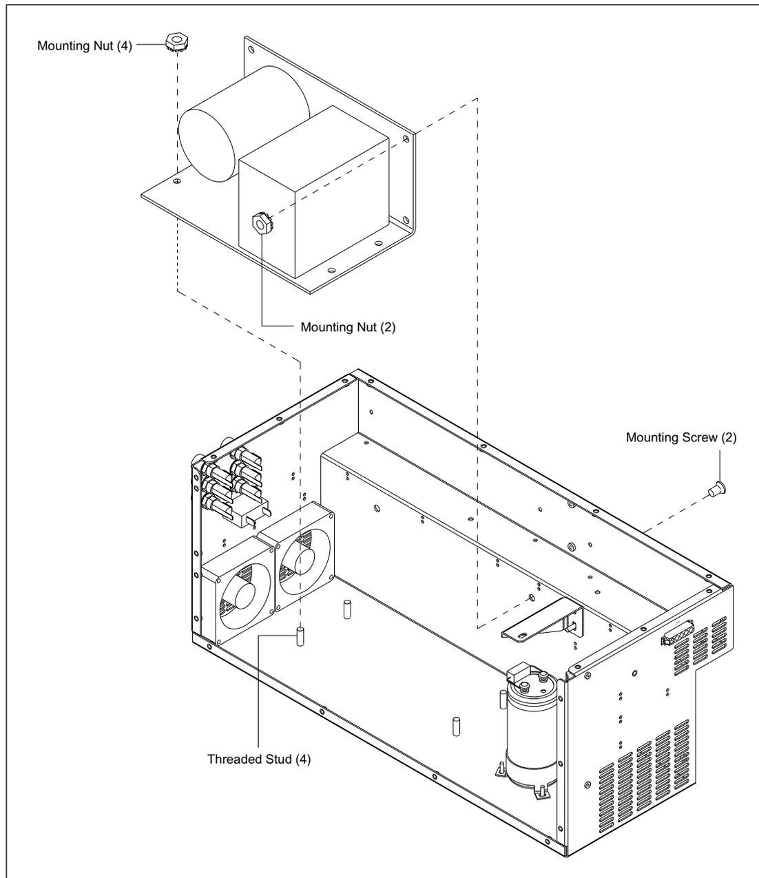
Figure 9-18. Heater Power Supply Mounting (Two-Supply Model).
