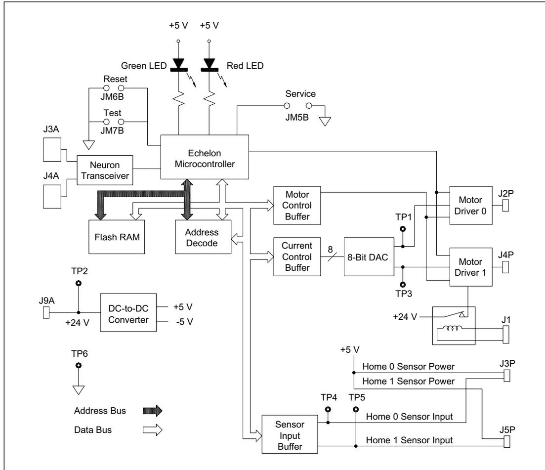
Figure 5-34. BEAM Board Block Diagram.
