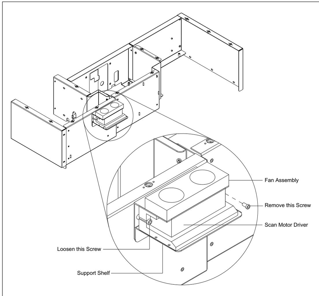
Figure 9-41. Scan Motor Driver Mounting.
