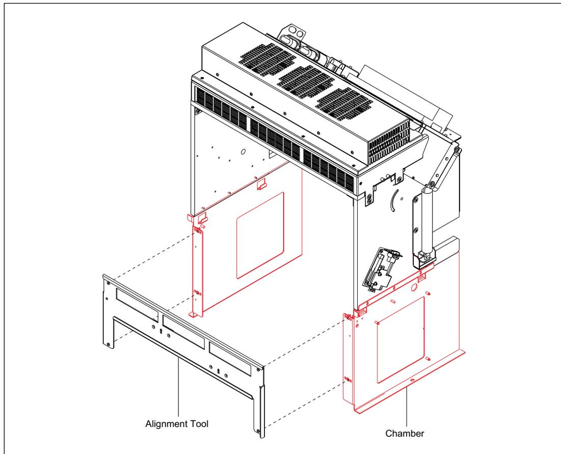
Figure 8-8. Alignment Tool Location.
