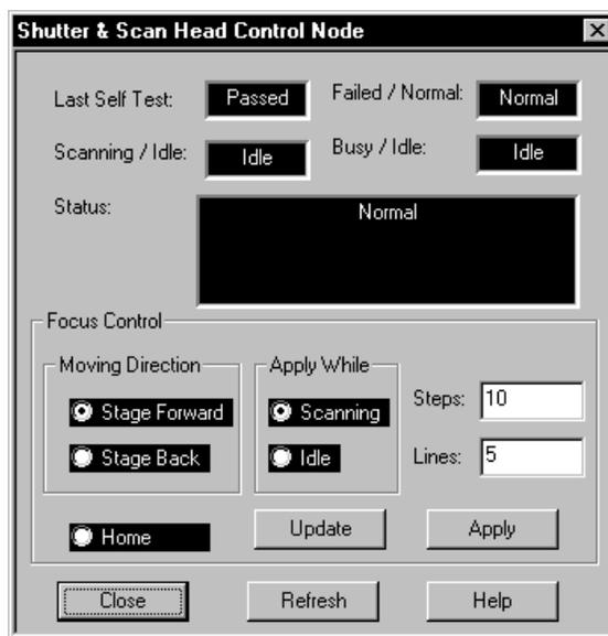
Figure 7-14. Shutter and Scan Head Control Node.
