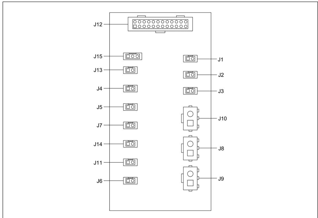
Figure 5-64. Pressure Connector Board Component Layout Diagram.
