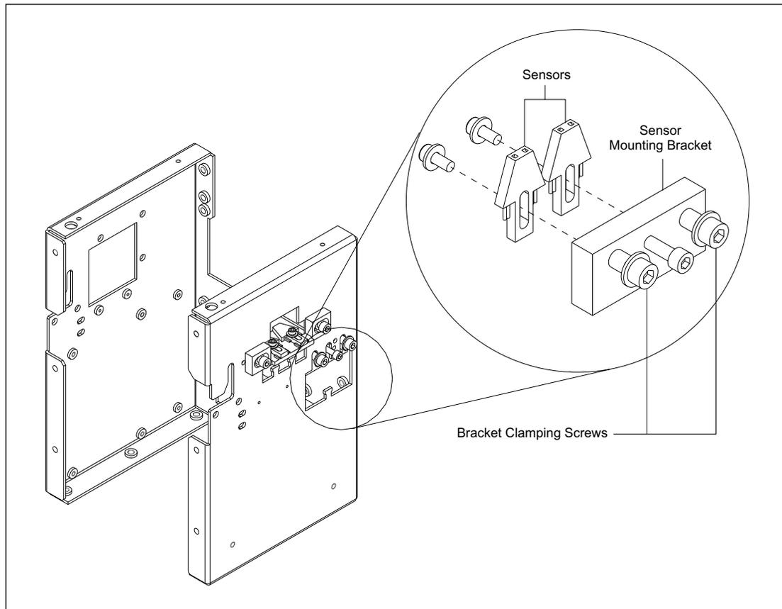
Figure 9-76. Indexer X-Position Sensor Mounting (MB 2000).
