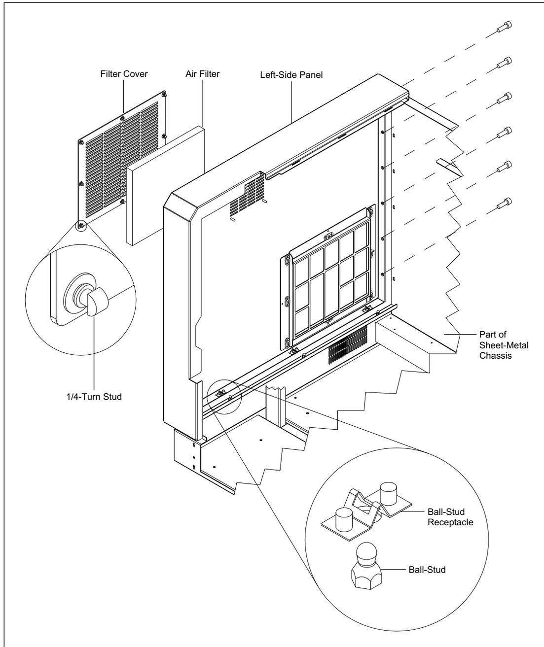
Figure 9-2. Left Panel and Air Filter Assembly Mounting.
