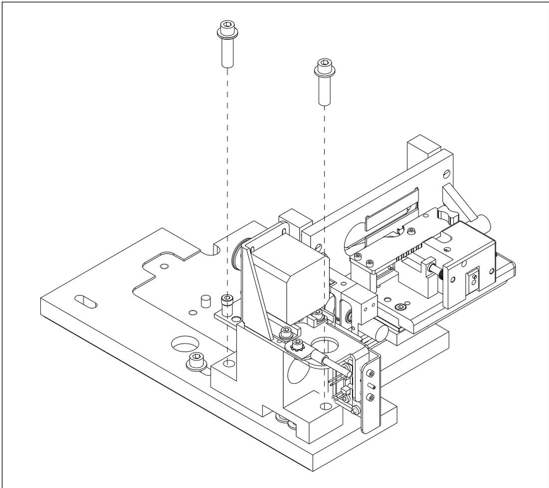
Figure 9-56. Focus Drive Assembly Mounting.
