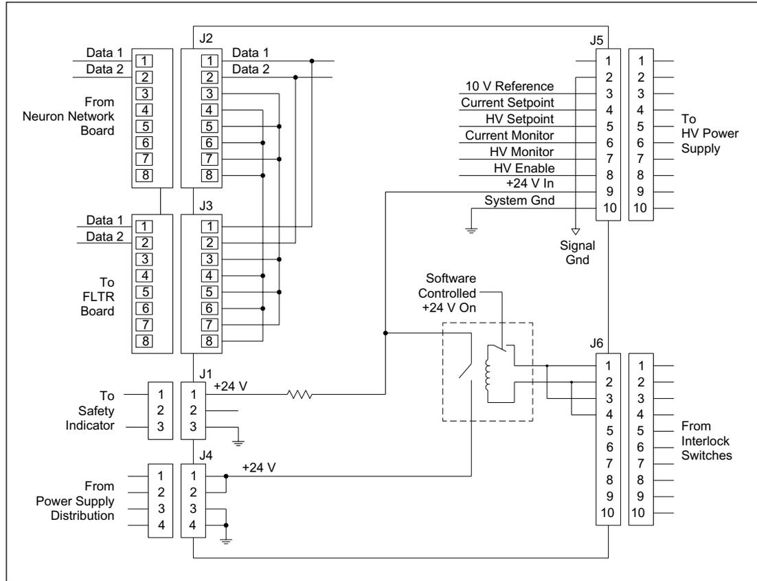
Figure 5-27. EPHV Board Connector Detail Diagram.
