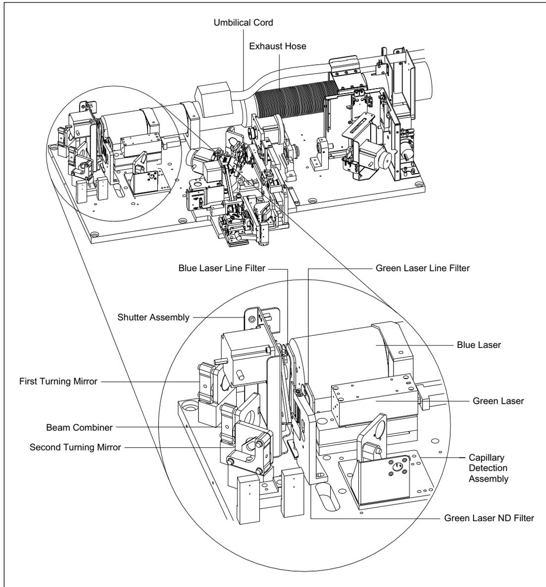
Figure 4-16. Optical Components Assembly (Sheet 1 of 3).
