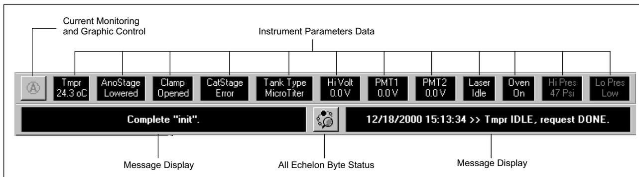
Figure 7-2. Instrument Parameter Data and Message Displays.
