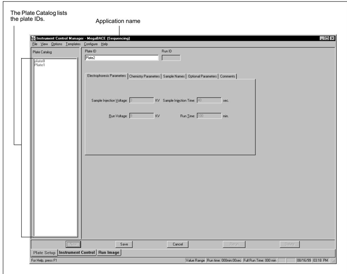
Figure 6-17. The Instrument Control Manager software displaying the Plate Setup window and the Plate Catalog. Note that sequencing is selected as the application and displayed in the title bar.
