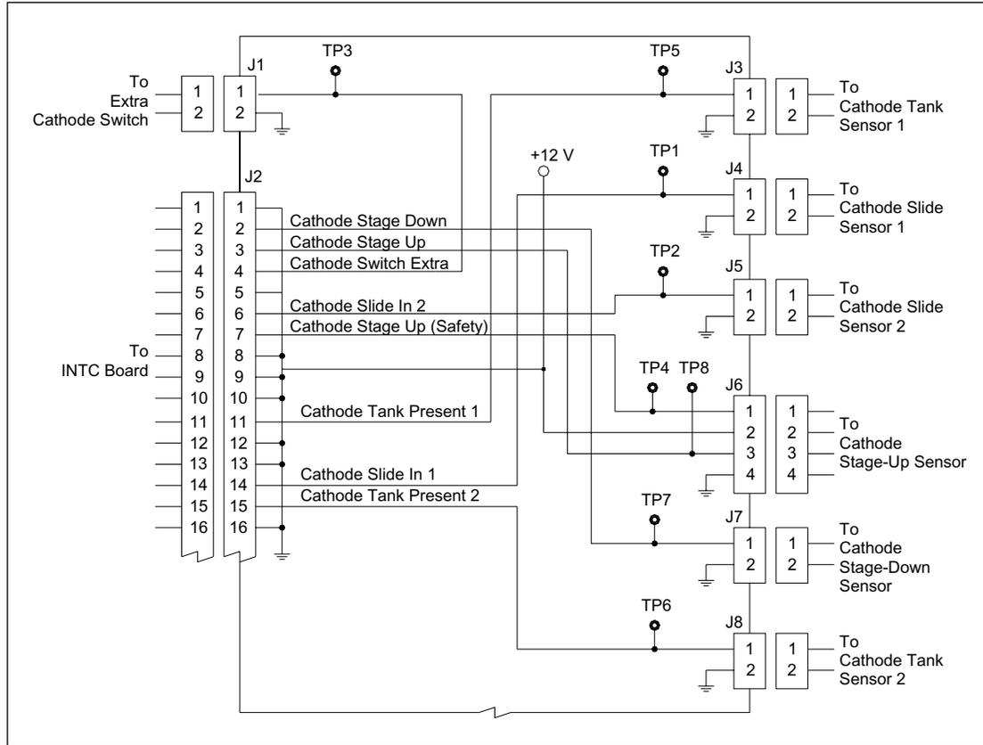
Figure 5-60. Cathode Connector Board Connector Detail Diagram (MB 2000) (Sheet 1 of 2).
