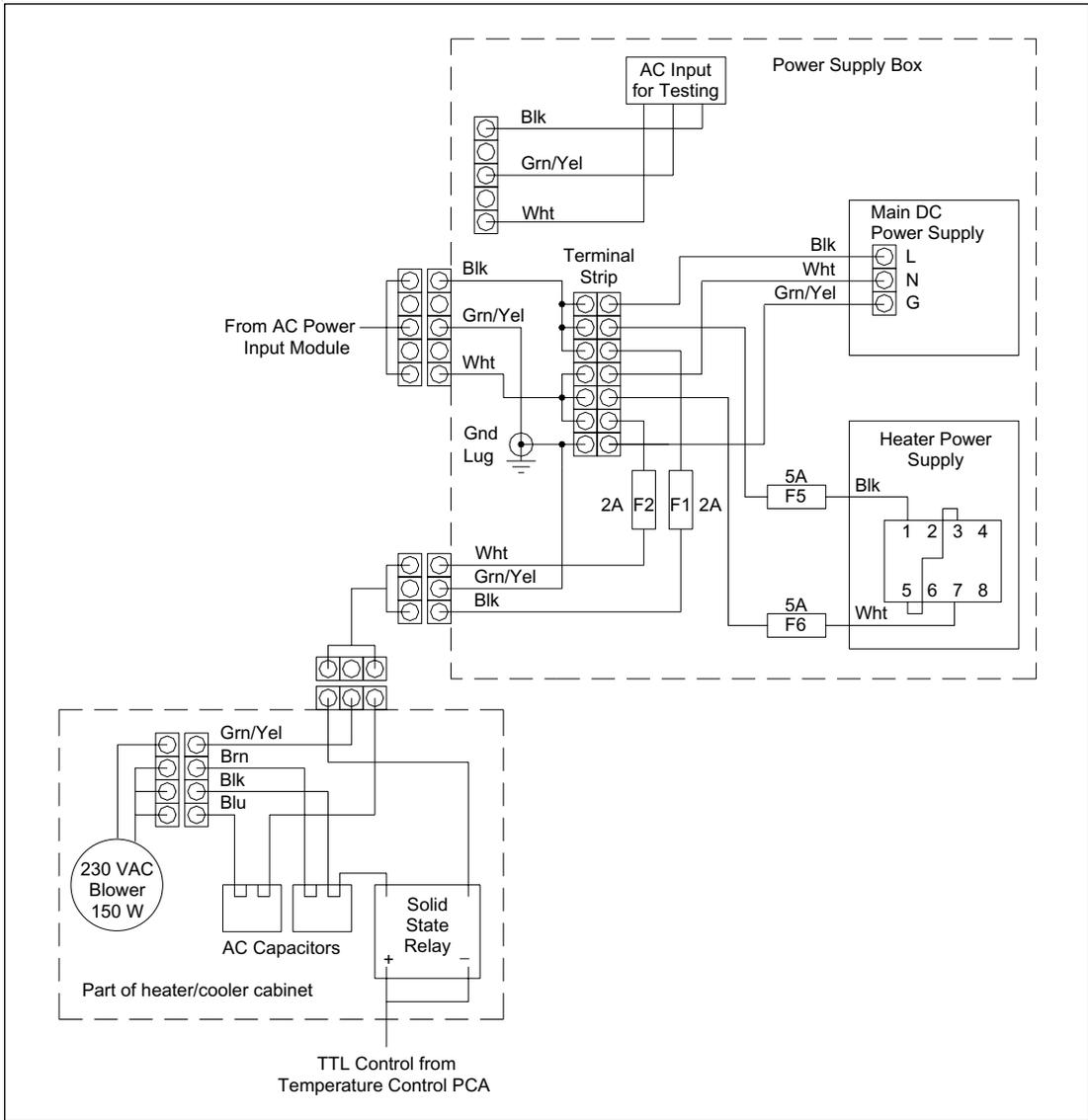
Figure 5-3. Main AC Distribution Block Diagram (Two-Supply Model).
