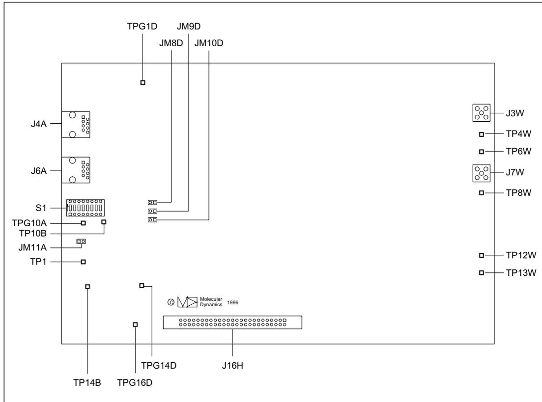
Figure 5-55. PDIO Board Component Layout Diagram.
