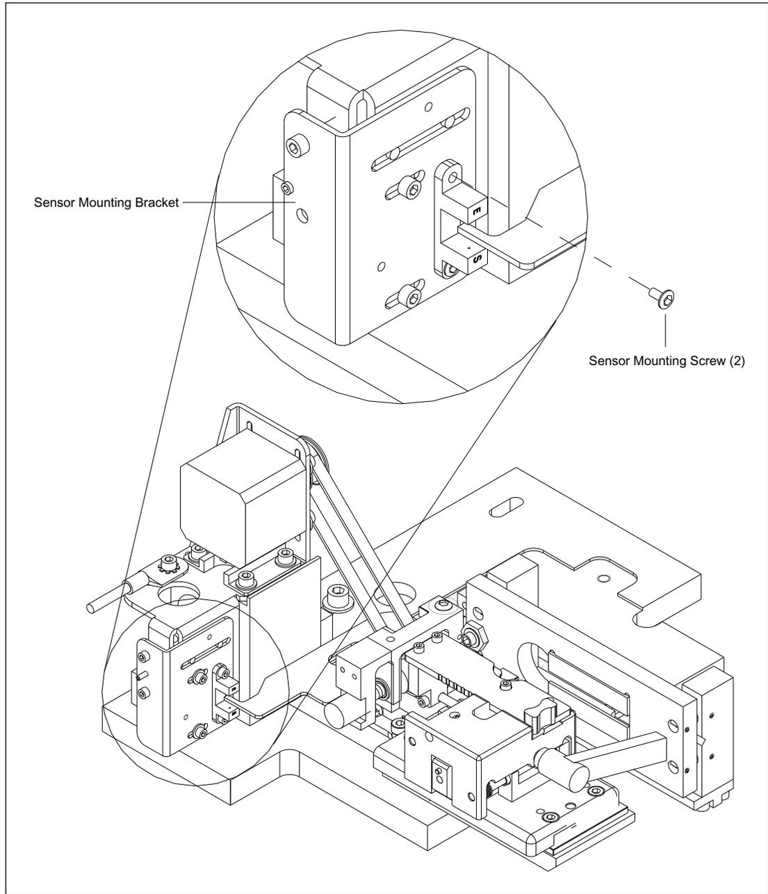
Figure 9-58. Focus Assembly Position Sensor Mounting.
