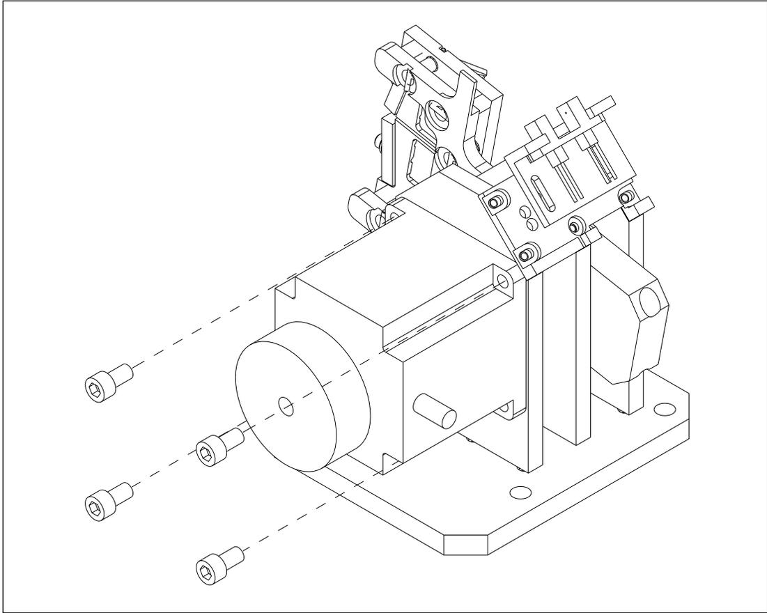
Figure 9-49. Primary Beamsplitter Changer Drive Motor Mounting.
