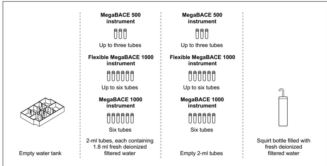
Figure 6-23. The Materials for the Flush and Dry Capillaries Protocol. **Note:** You use one tube of water for each capillary array installed in the instrument.
