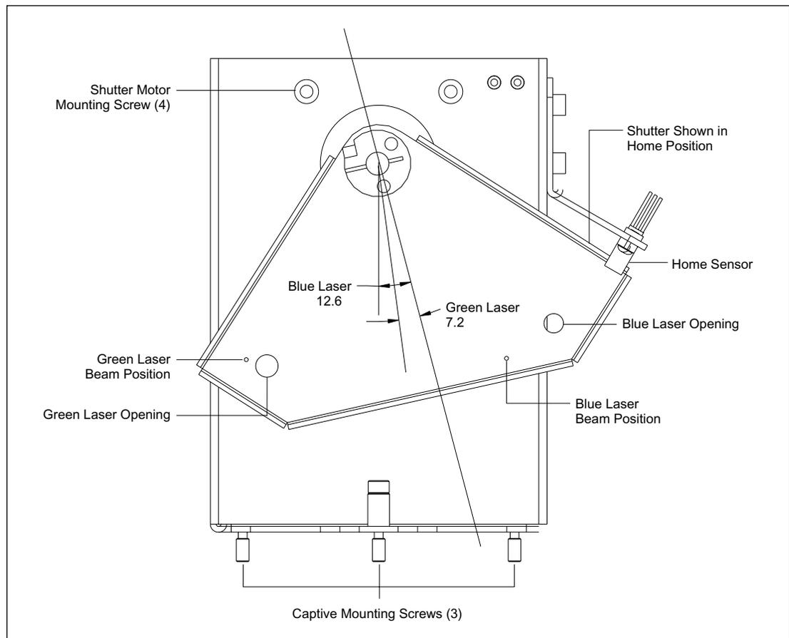
Figure 4-24. Three-Position Shutter Assembly (Sheet 2 of 2).
