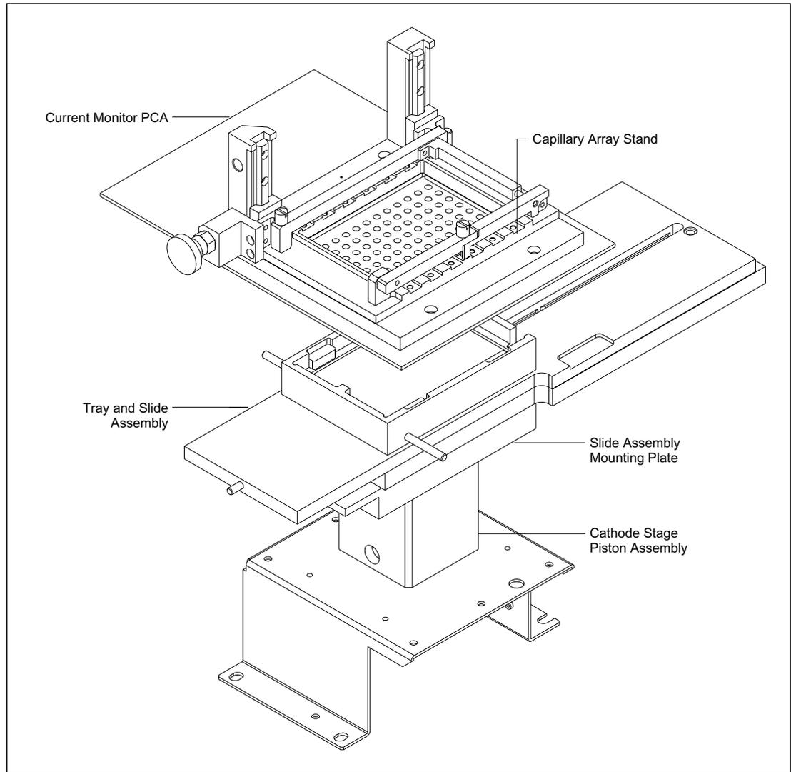
Figure 4-42. Cathode Assembly, Simplified View.
