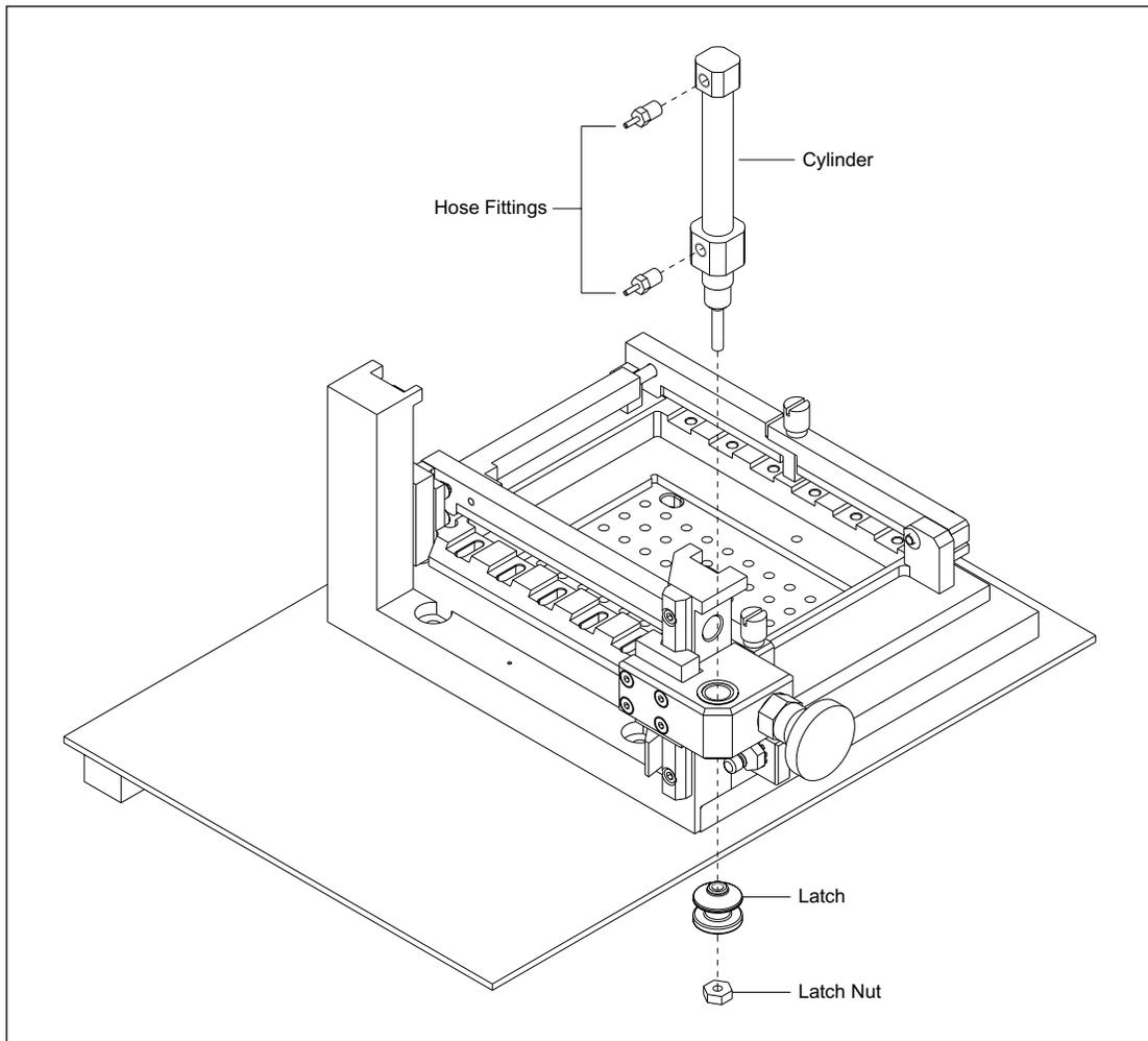
Figure 9-74. Capillary Array Stage Actuator Mounting (MB 2000).
