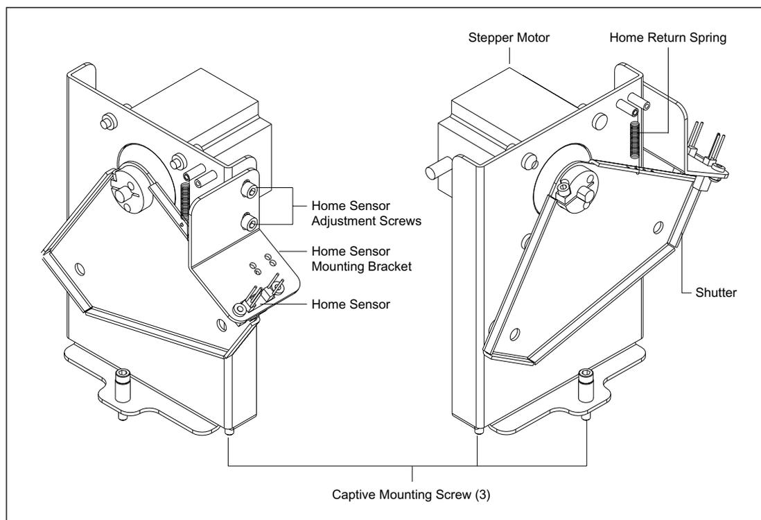
Figure 4-23. Three-Position Shutter Assembly (Sheet 1 of 2).
