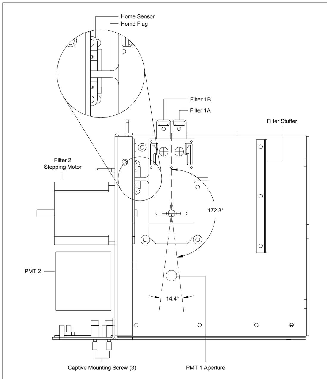
Figure 4-38. Filter Changer Arm Assembly.
