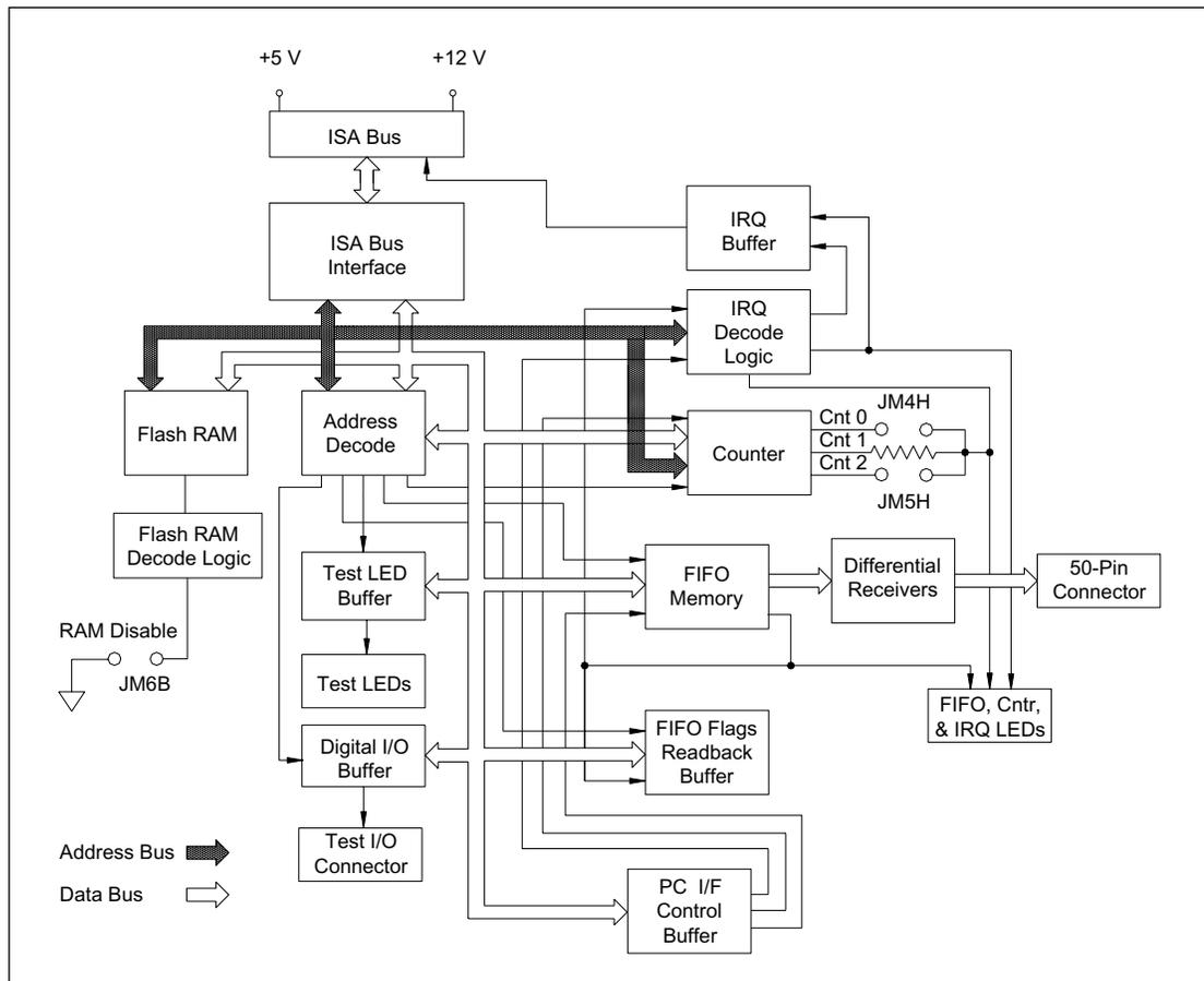
Figure 5-22. PC Interface Board Block Diagram.
