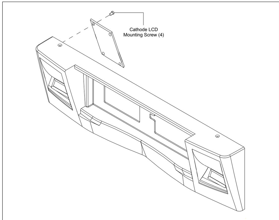
Figure 9-9. Cathode LCD Board Mounting.
