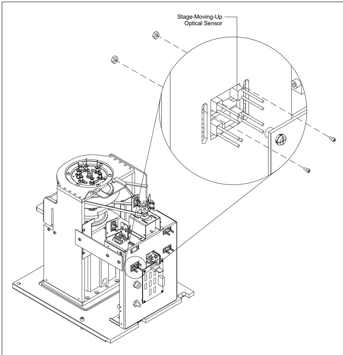
Figure 9-90. Anode Stage-Moving-Up Optical Sensor Mounting.
