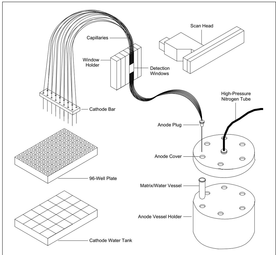
Figure 2-2. Capillary Array.
