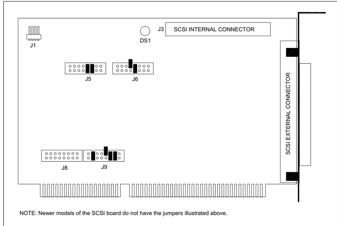
Figure 9-32. SCSI Interface Board Jumper Configuration.
