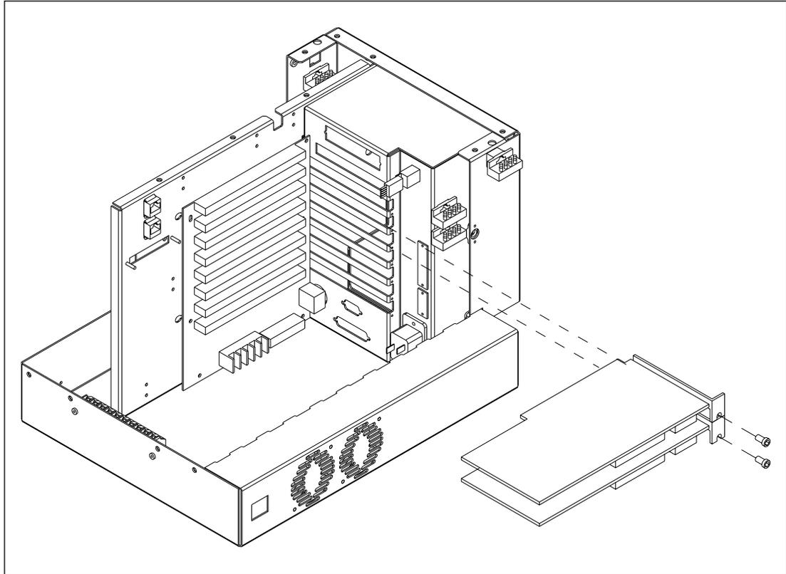
Figure 9-33. Analog Interface Board Mounting.
