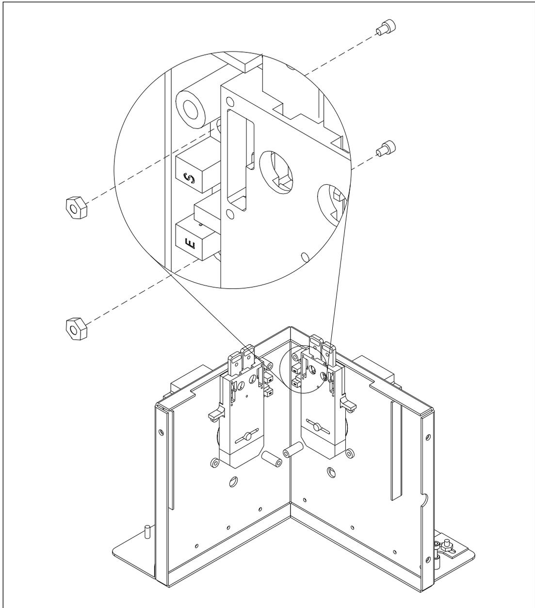
Figure 9-65. Filter Changer Home Sensor Mounting.
