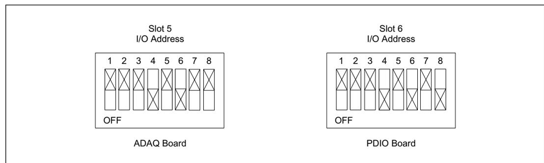
Figure 9-34. Analog Interface Board Address Programming.
