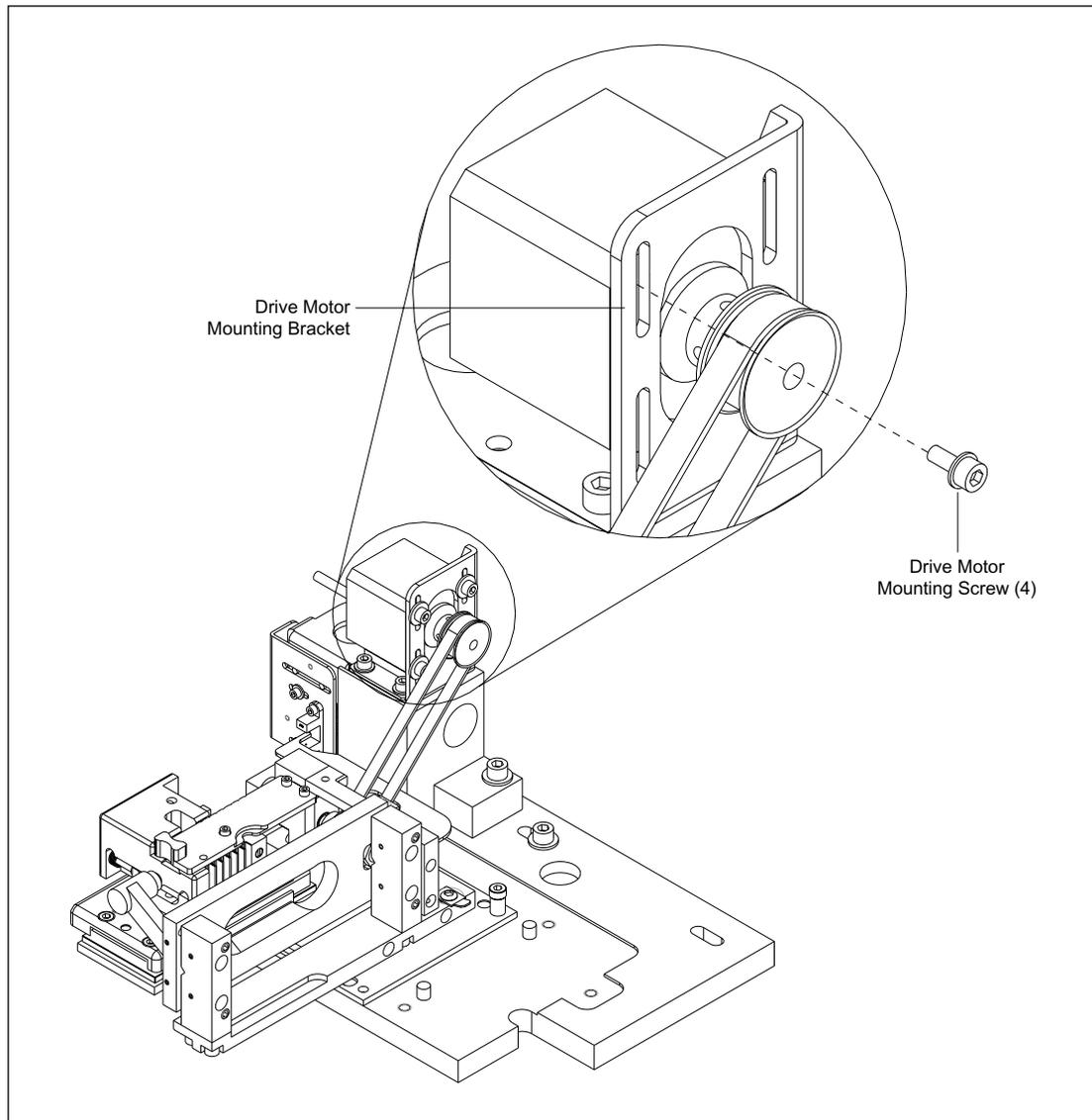
Figure 9-57. Focus Assembly Drive Motor Mounting.
