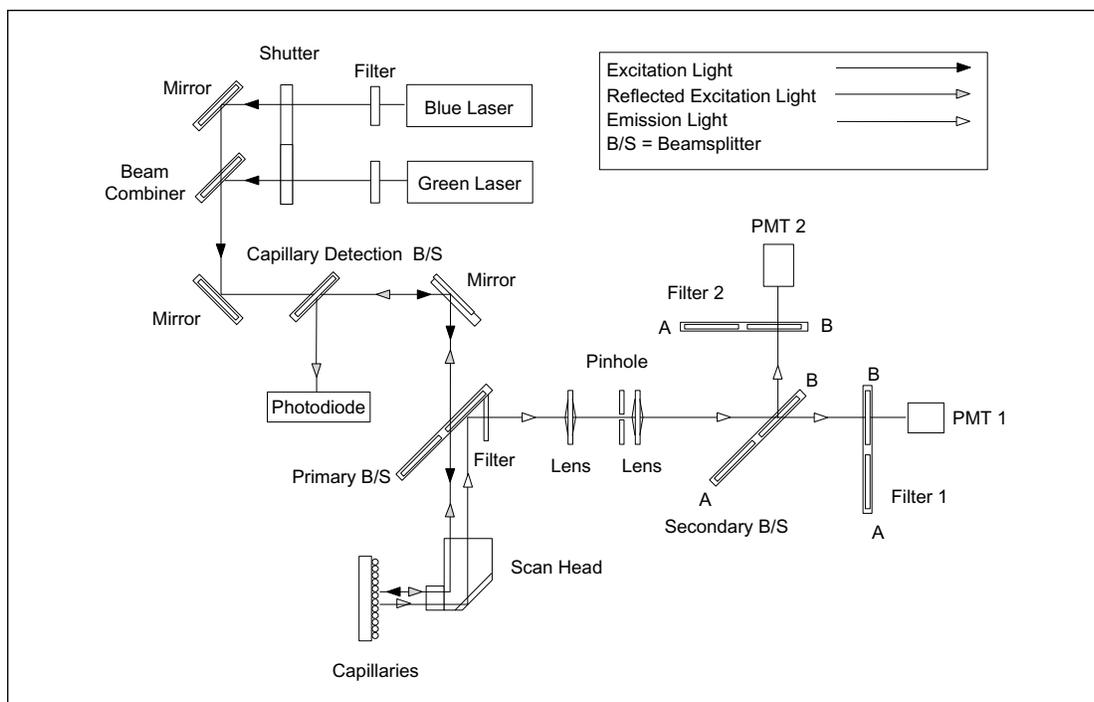
Figure 2-4. Optics, Simplified Block Diagram.
