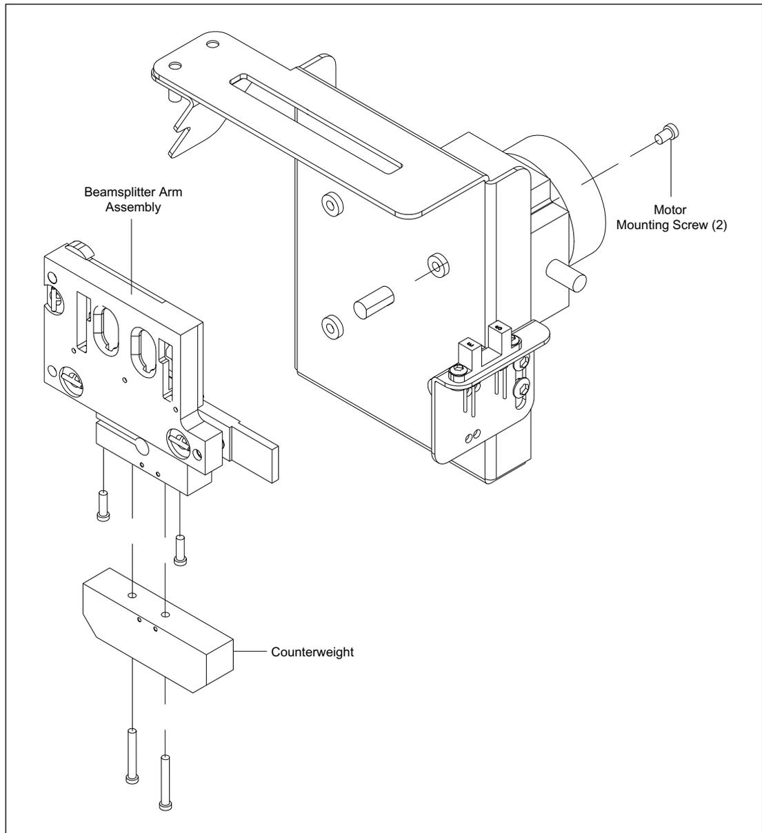
Figure 9-61. Secondary Beamsplitter Arm Assembly Mounting.
