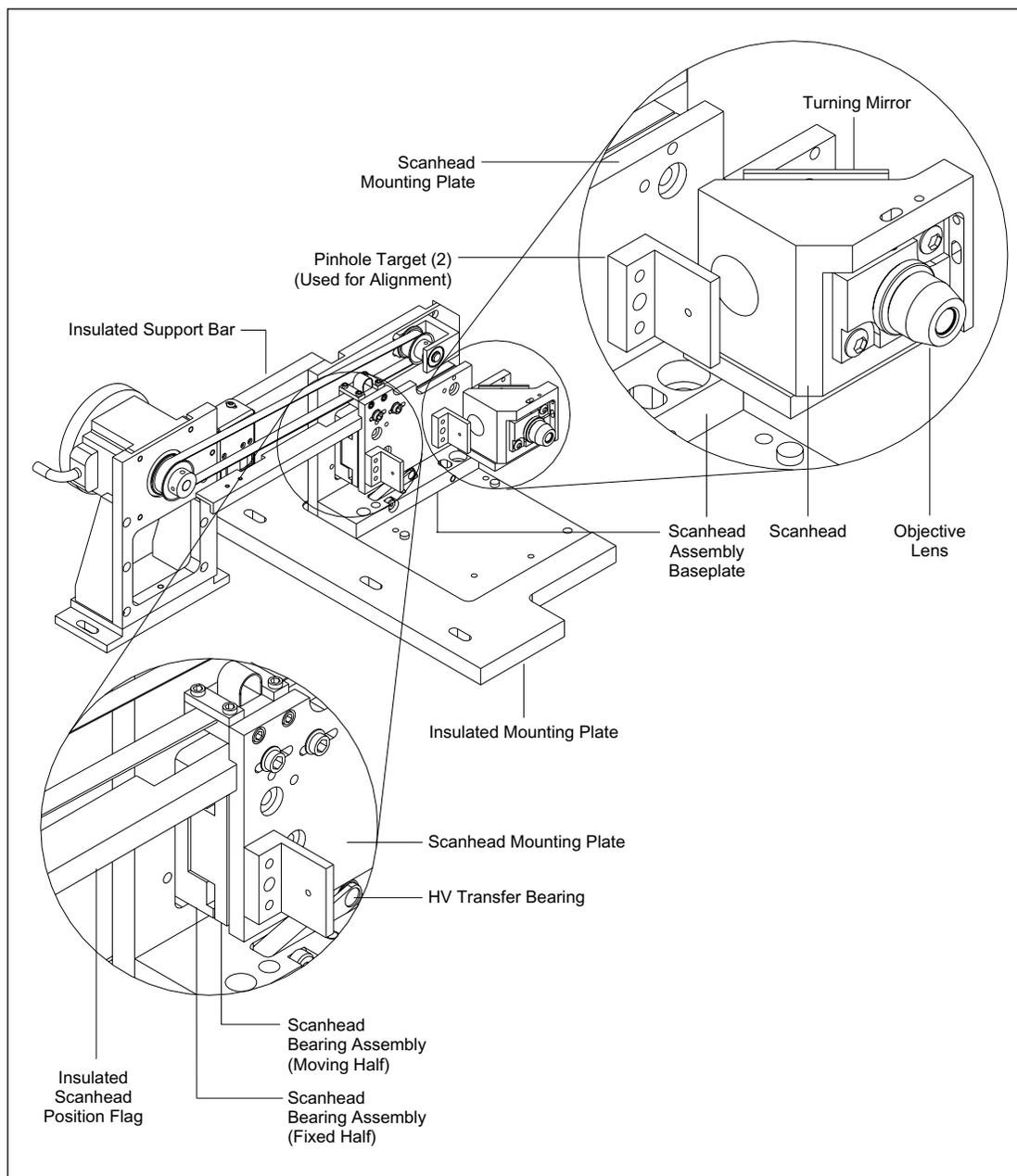
Figure 4-30. Scanhead Assembly.
