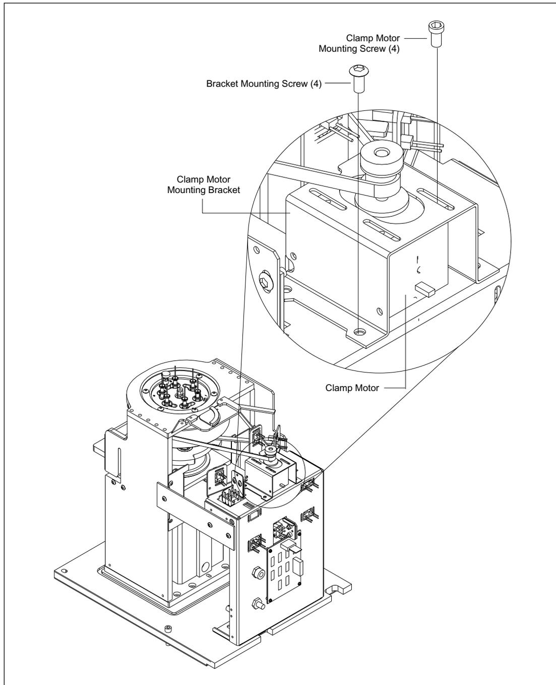
Figure 9-92. Anode Cover Locking Motor Mounting.
