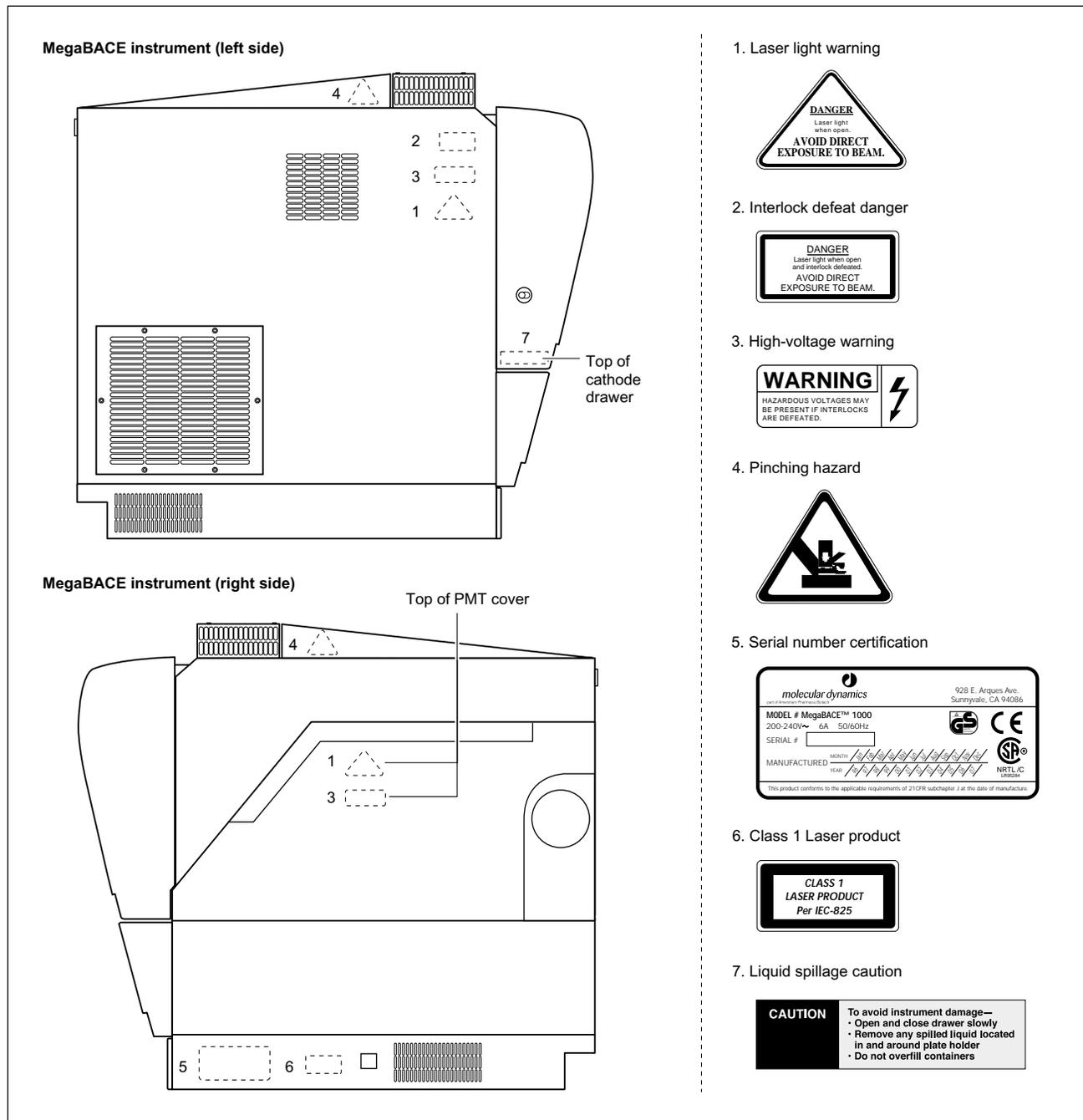
Figure 6-12. Location of Important Labels On The Instrument (Side Views).
