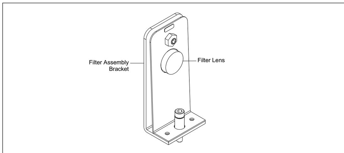
Figure 3-10. Laser Line Filter.
