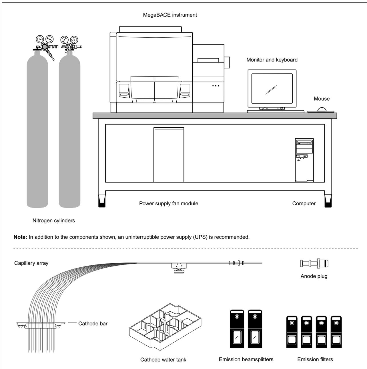
Figure 2-1. The MegaBACE Instrument.
