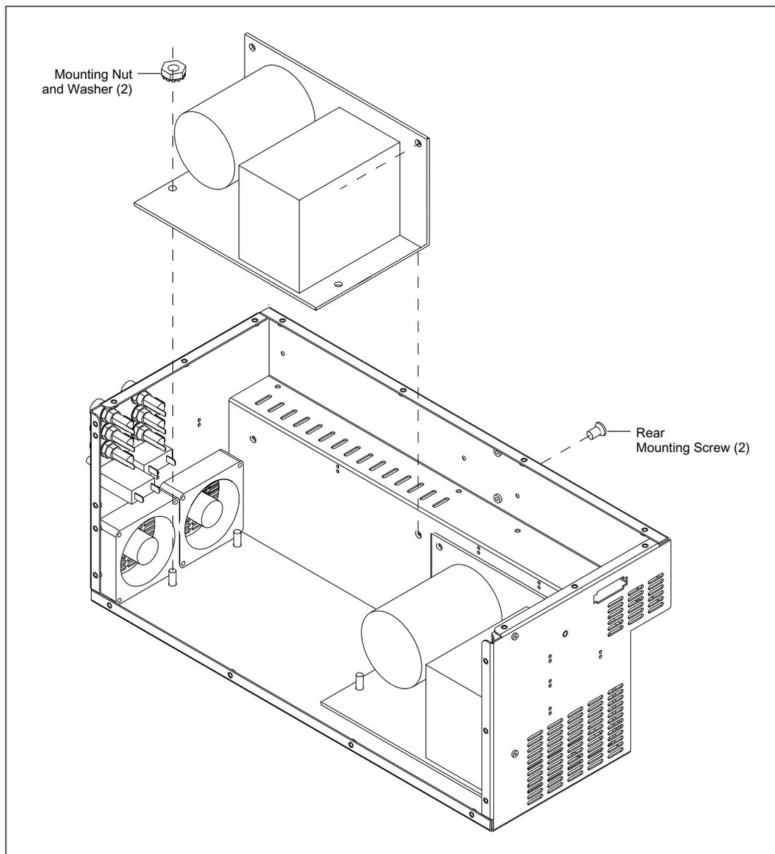
Figure 9-15. Cooler Power Supply Mounting.
