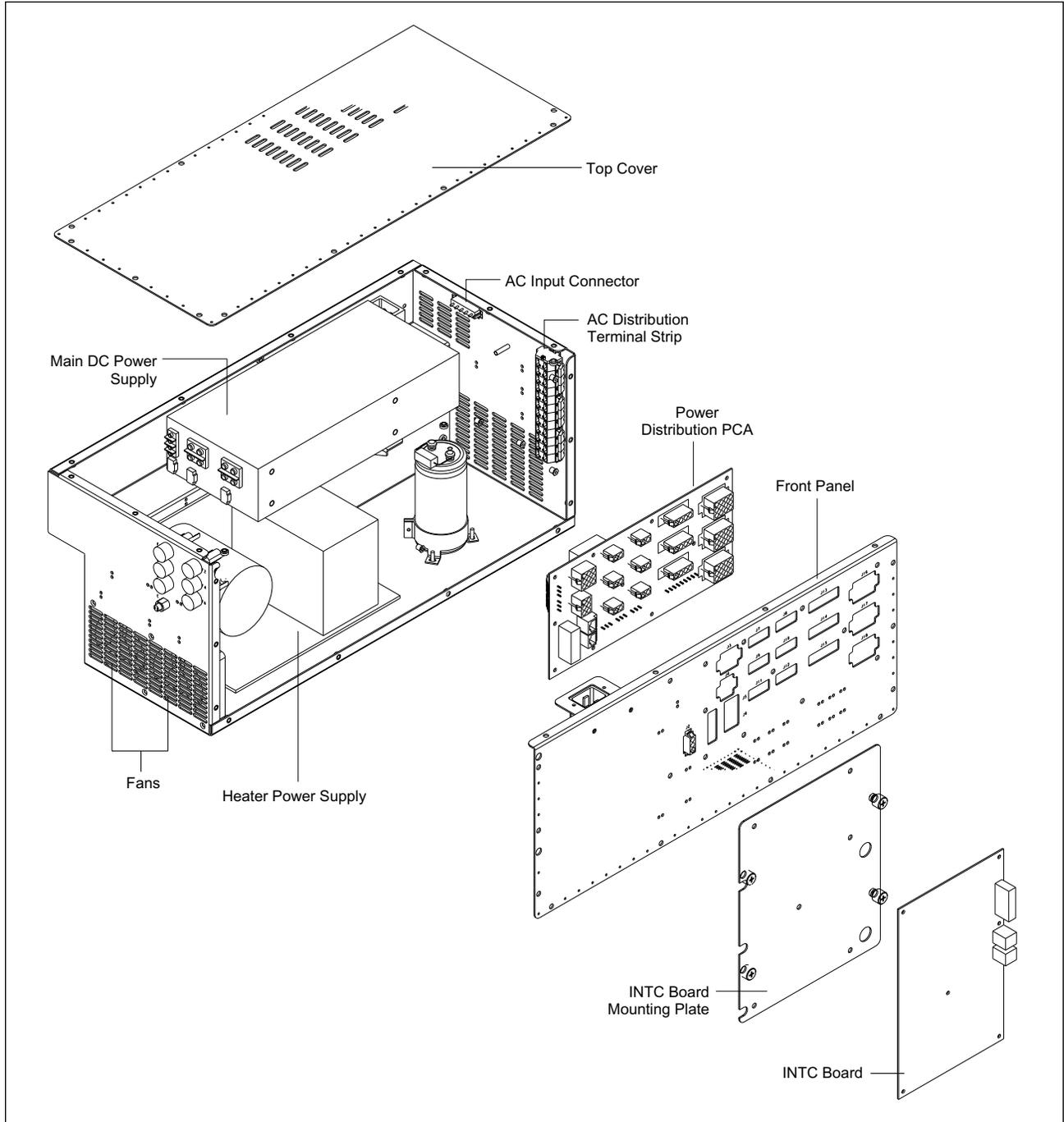
Figure 4-10. Power Supply Box Assembly.
