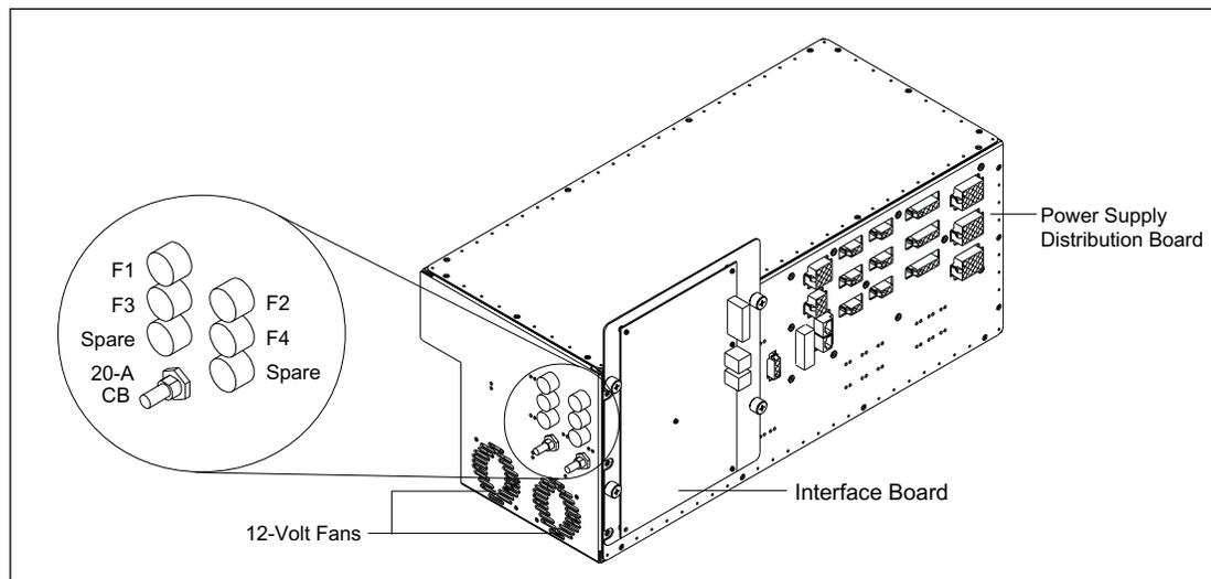
Figure 5-8. Power Supply Box (Two-Supply Model).
