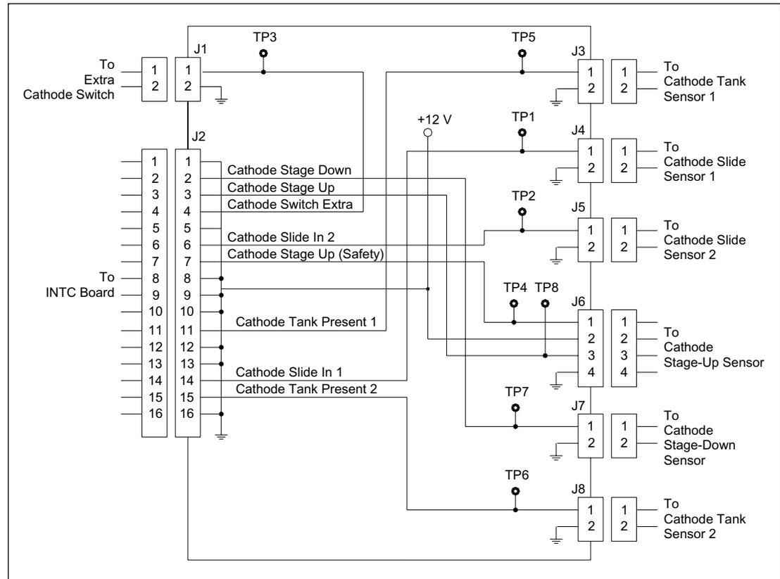
Figure 5-58. Cathode Connector Board Connector Detail Diagram.
