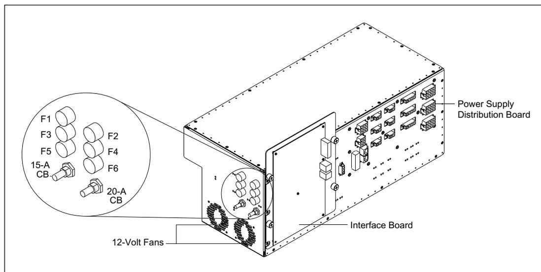
Figure 5-6. Power Supply Box (Four-Supply Model).
