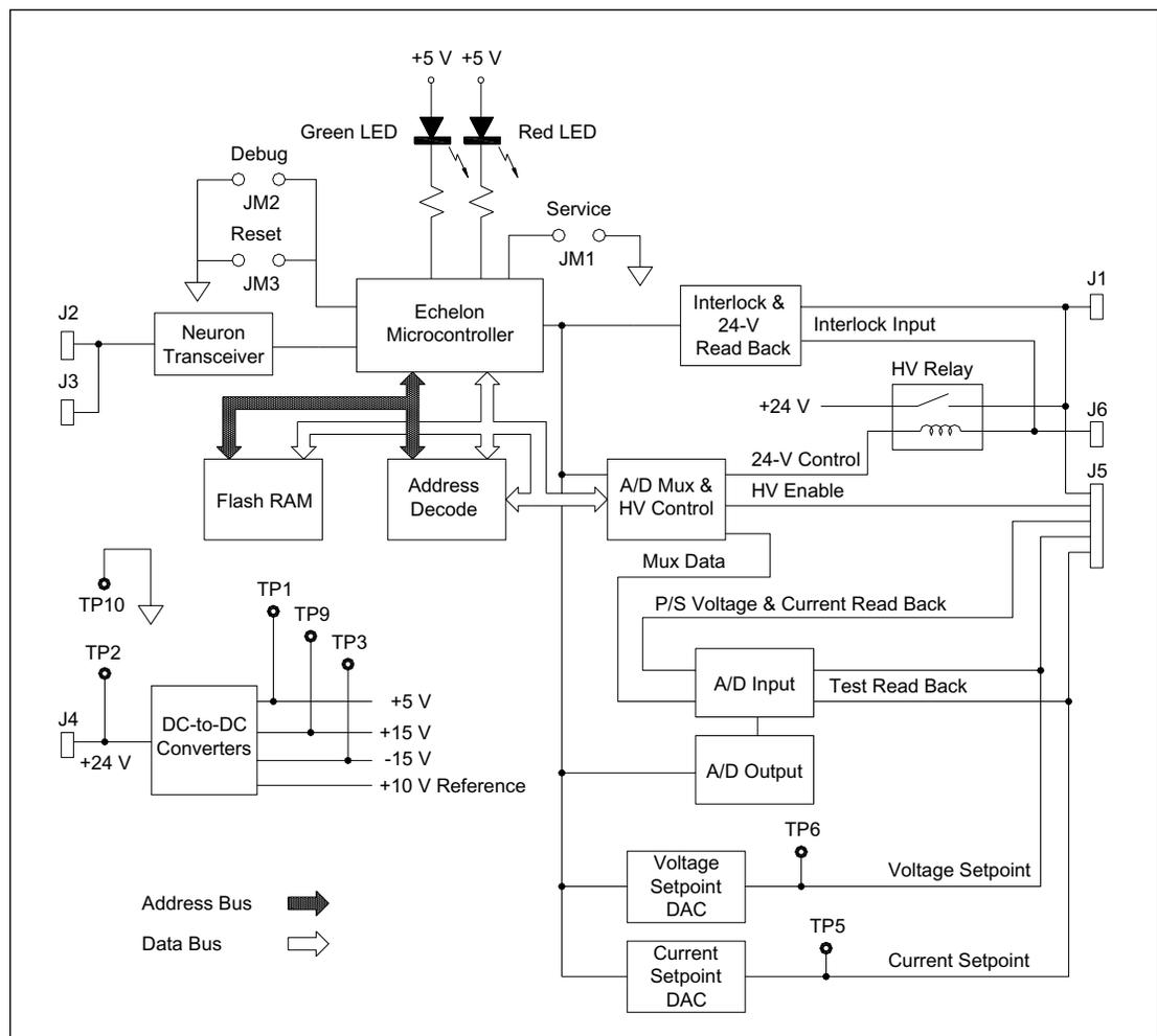
Figure 5-25. EPHV Board Block Diagram.
