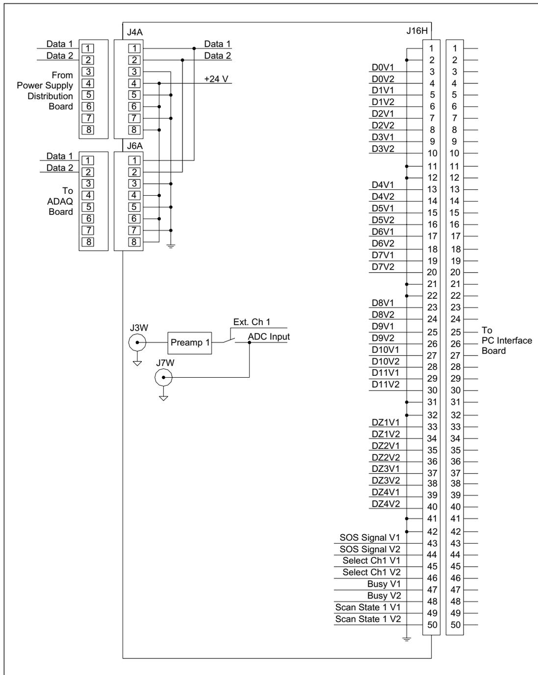
Figure 5-56. PDIO Board Connector Detail Diagram.
