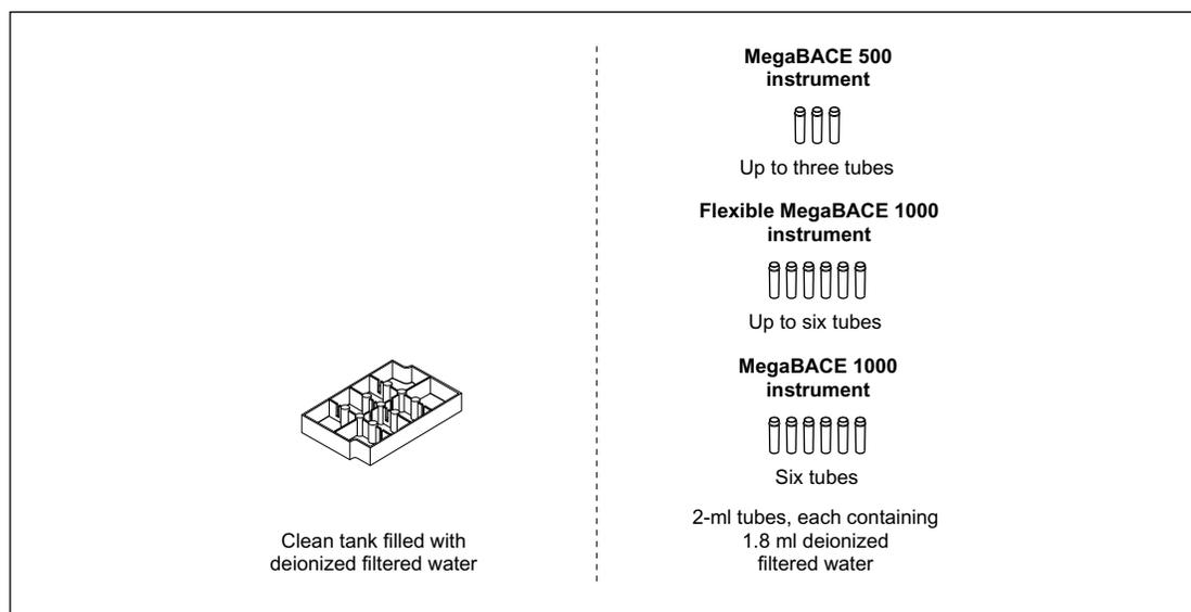
Figure 6-21. The Materials for the Store Capillaries Protocol. **Note:** You use one tube of water for each capillary array installed in the instrument.
