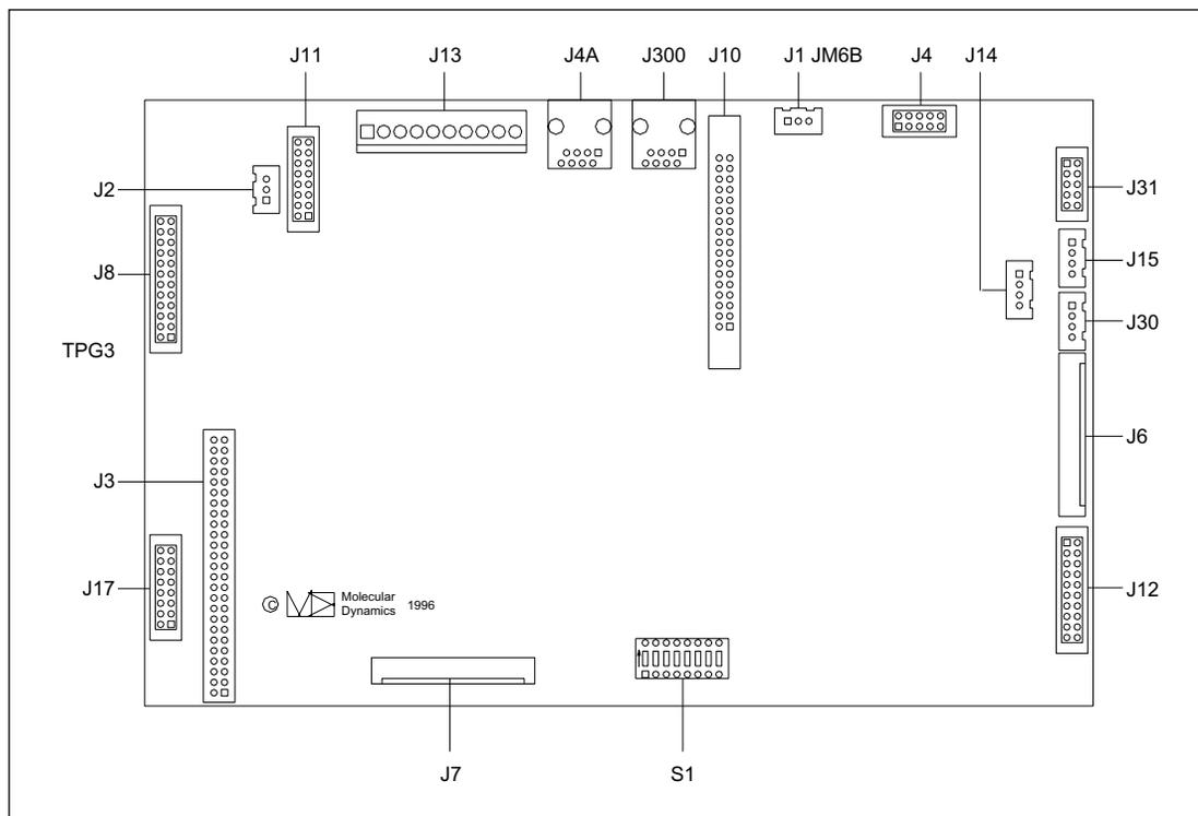
Figure 5-43. INTC Board (Later Model) Component Layout Diagram.
