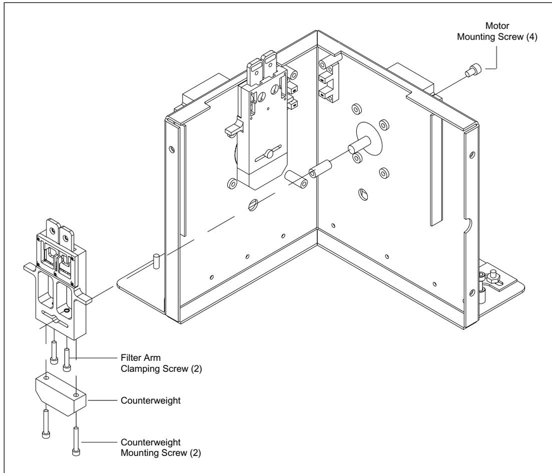
Figure 9-64. Filter Changer Arm Assembly Mounting.
