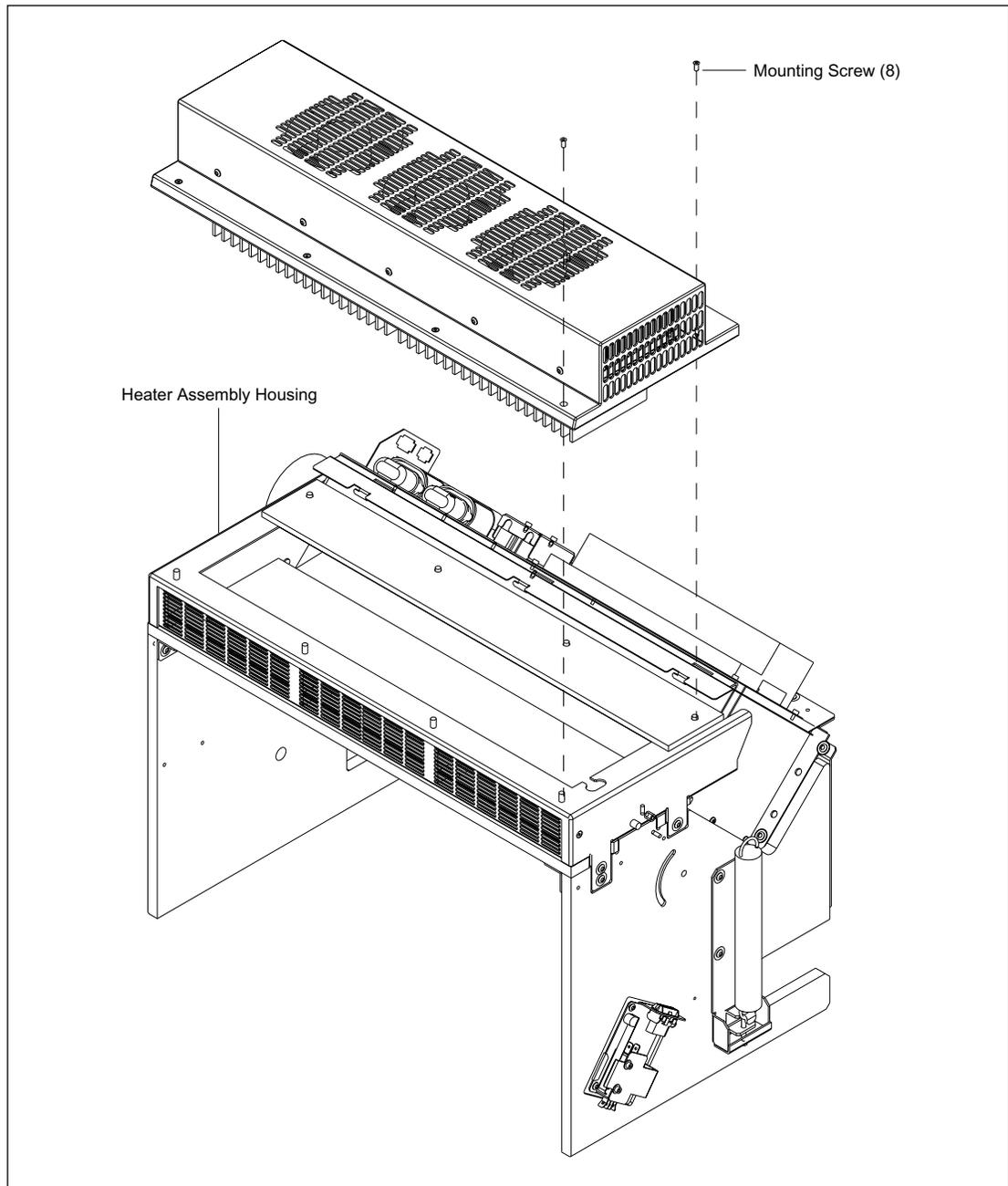
Figure 9-23. TE Cooler Assembly Mounting.
