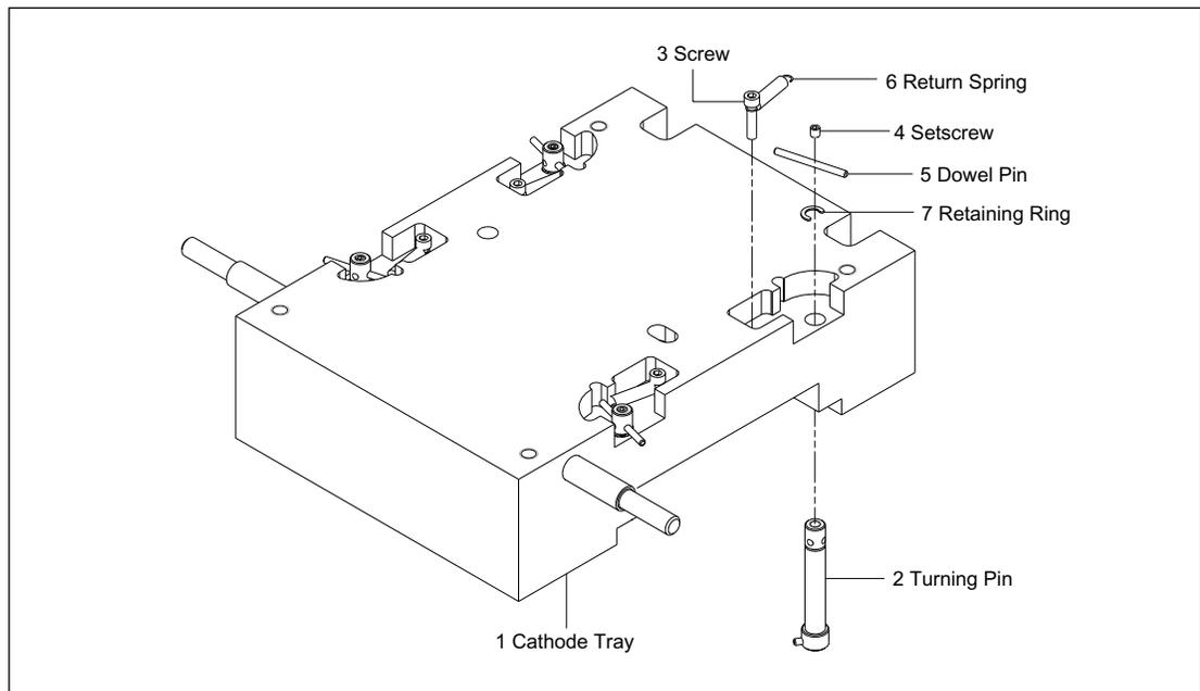
Figure 8-2. Cathode Tray, Bottom View.
