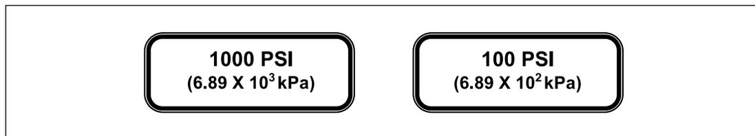
Figure 6-6. High- and Low-pressure Nitrogen Labels.
