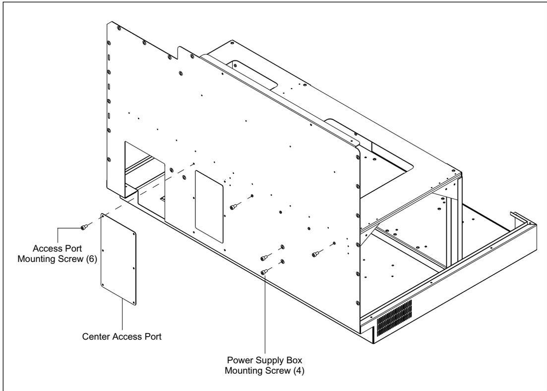
Figure 9-10. Power Supply Box Mounting.
