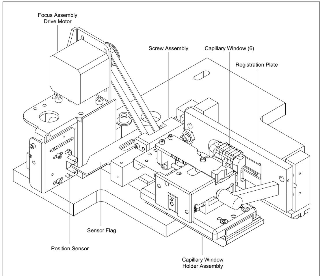
Figure 4-32. Capillary Window Platform Assembly.
