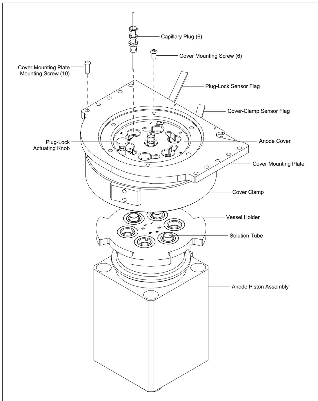
Figure 4-50. Anode Assembly, Simplified View.
