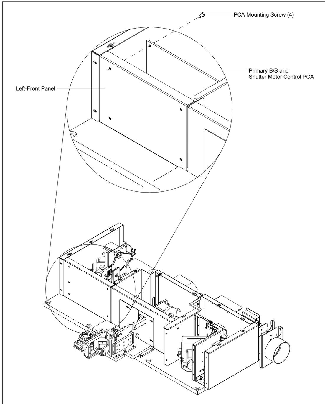
Figure 9-39. BEAM Board Mounting.
