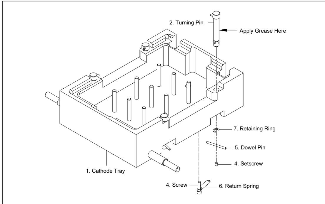
Figure 8-1. Cathode Tray, Top View.
