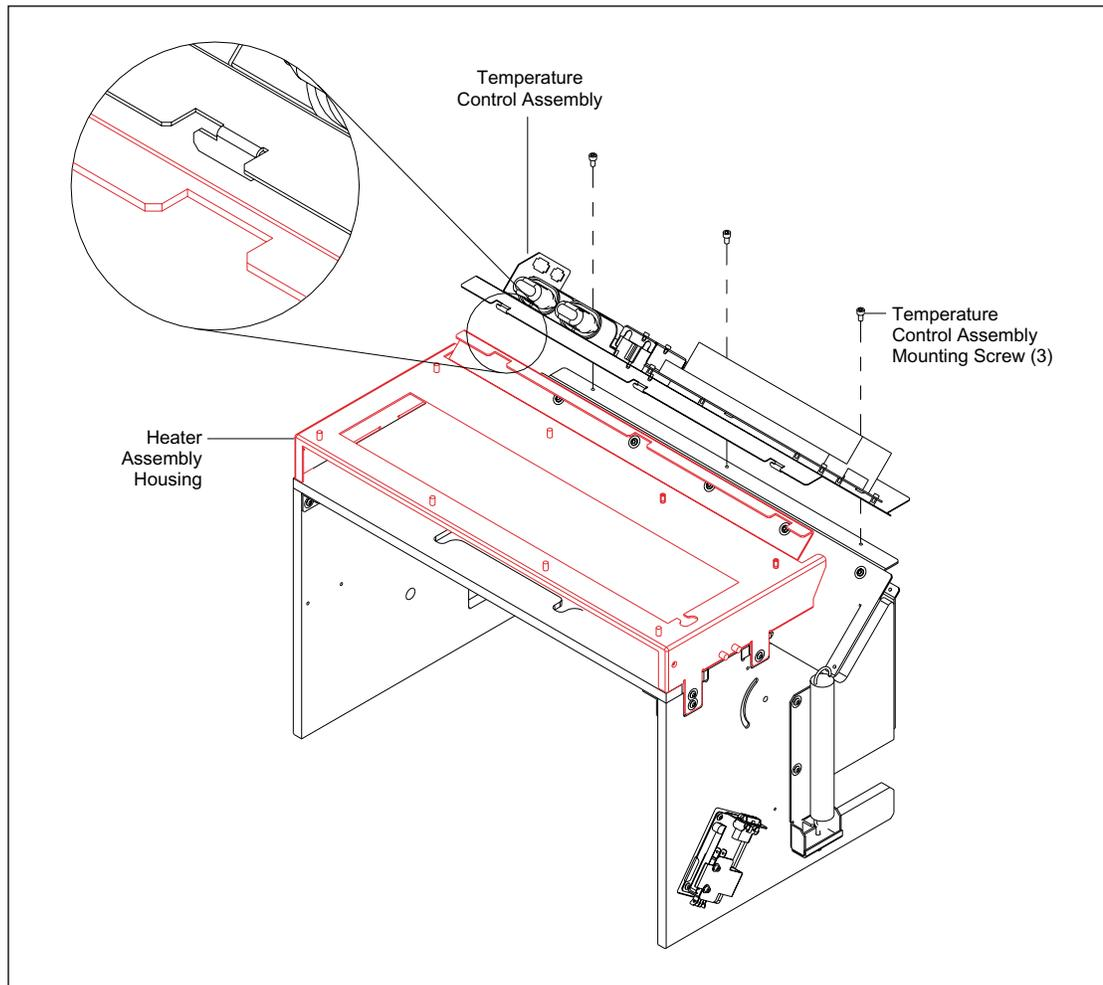
Figure 9-21. Temperature Control Assembly Mounting.
