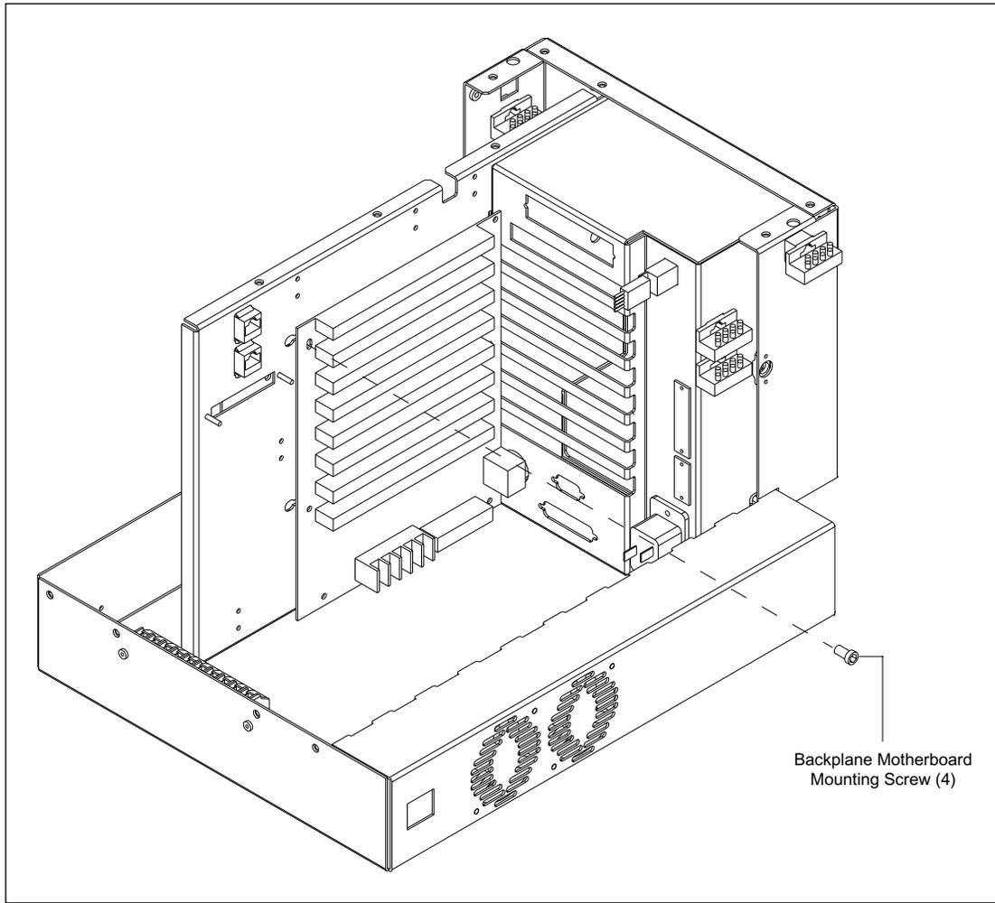
Figure 9-37. Backplane Motherboard Mounting.
