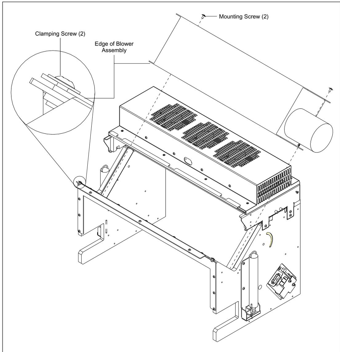
Figure 9-25. Blower Assembly Mounting.
