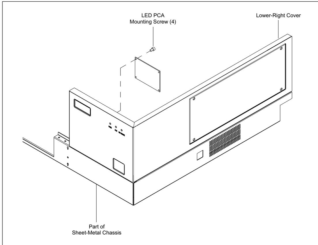
Figure 9-6. LED Board Mounting.
