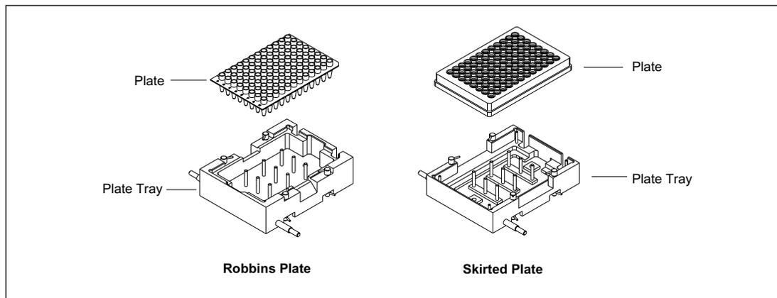
Figure 8-13. The water tank for the Robbins Plate and the Skirted Plate.
