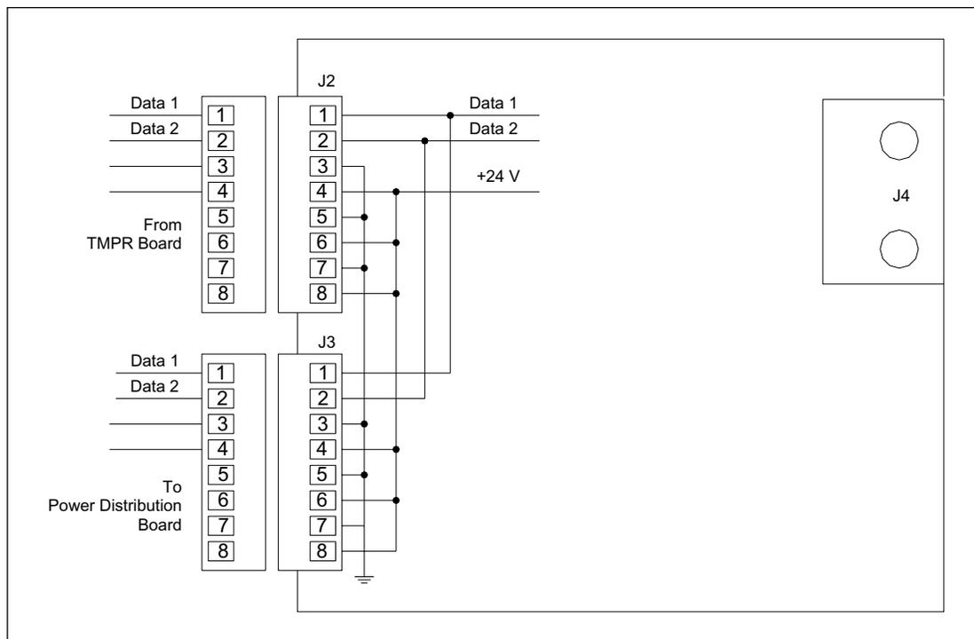
Figure 5-50. CMON Board Connector Detail Diagram.
