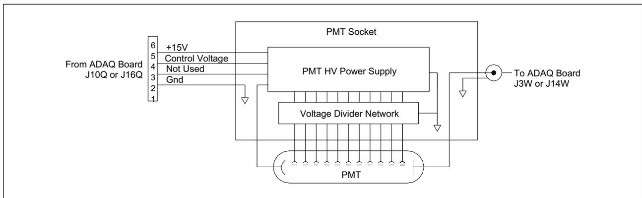
Figure 5-17. PMT High-Voltage Power Supply Block Diagram.
