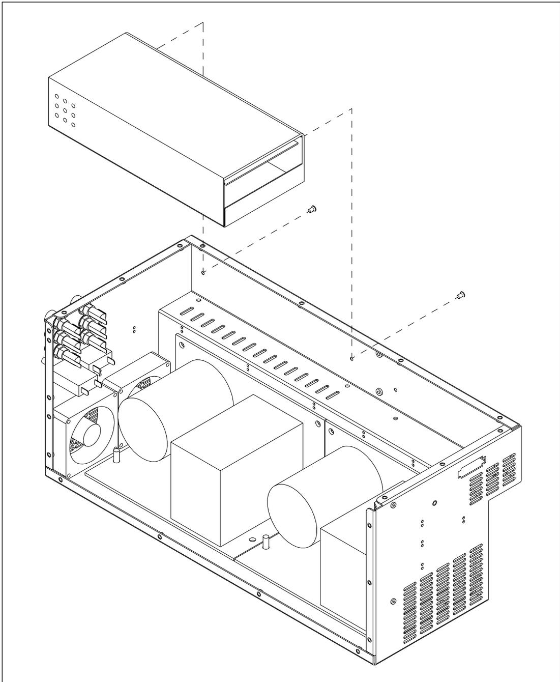
Figure 9-14. Echelon/Motor Power Supply Mounting.
