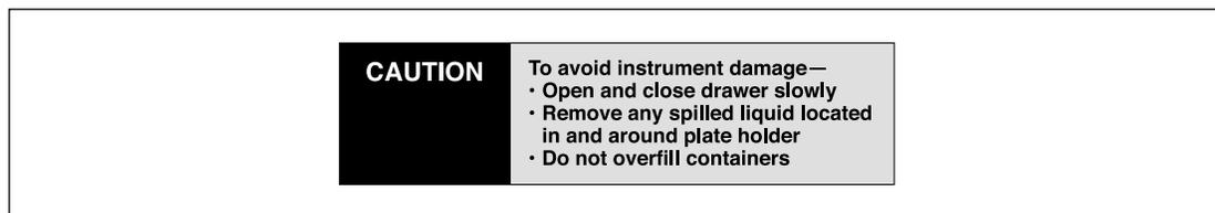
Figure 6-2. The liquid spillage caution label.
