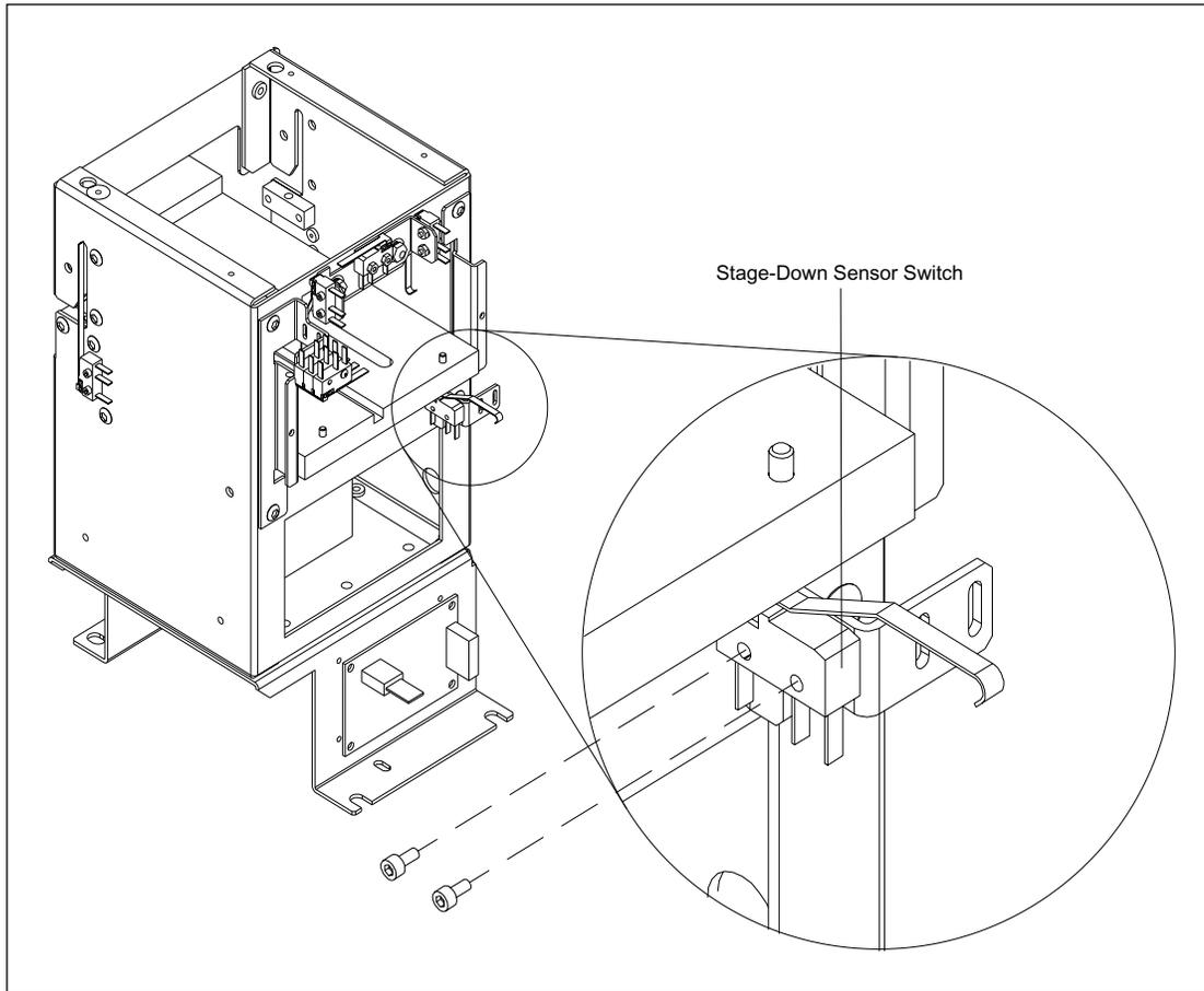
Figure 9-73. Cathode Stage-Down Sensor Switch Mounting.
