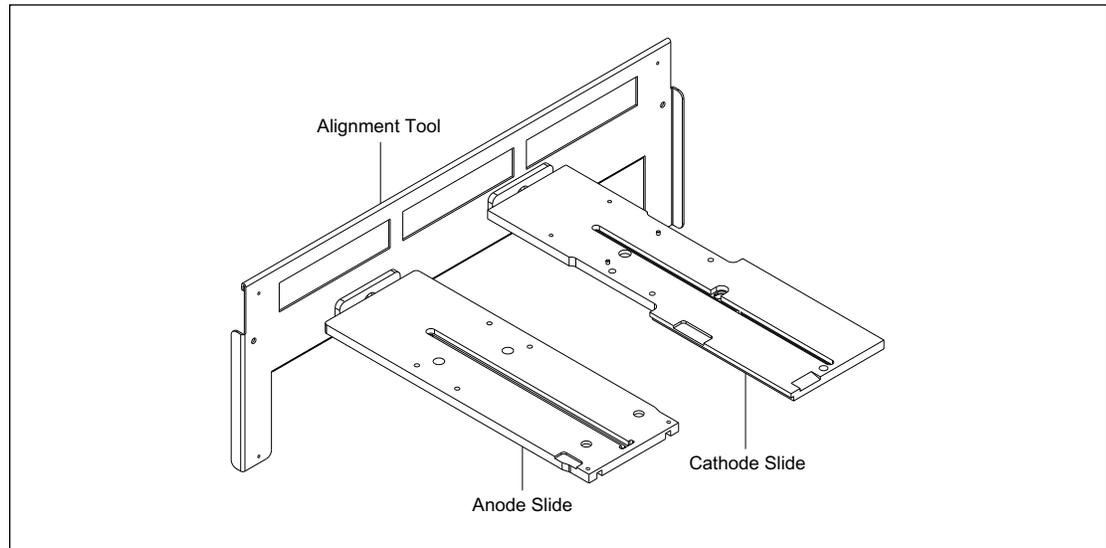
Figure 8-9. Slides Mated with Alignment Tool.
