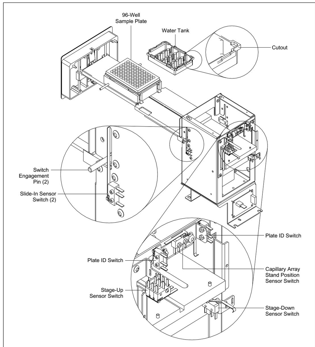
Figure 4-46. Cathode Assembly, Switch Locations.
