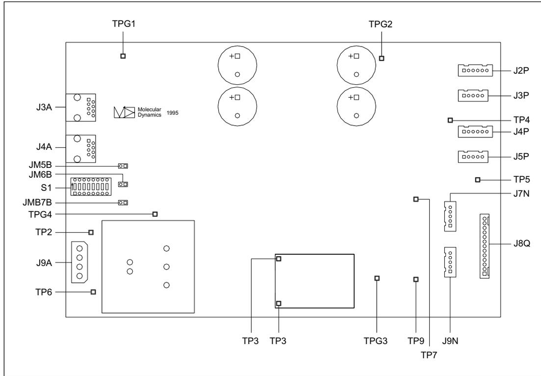
Figure 5-32. SCAN Board Component Layout Diagram.
