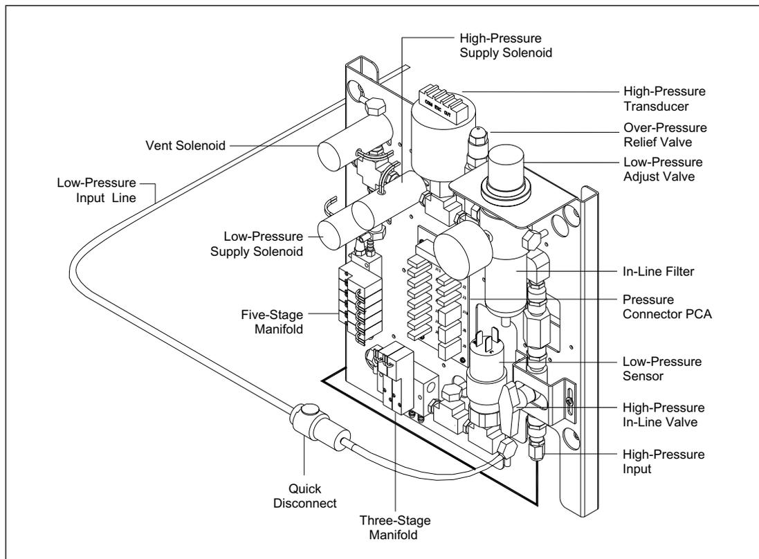
Figure 4-55. Pneumatic Assembly (MB 1000).
