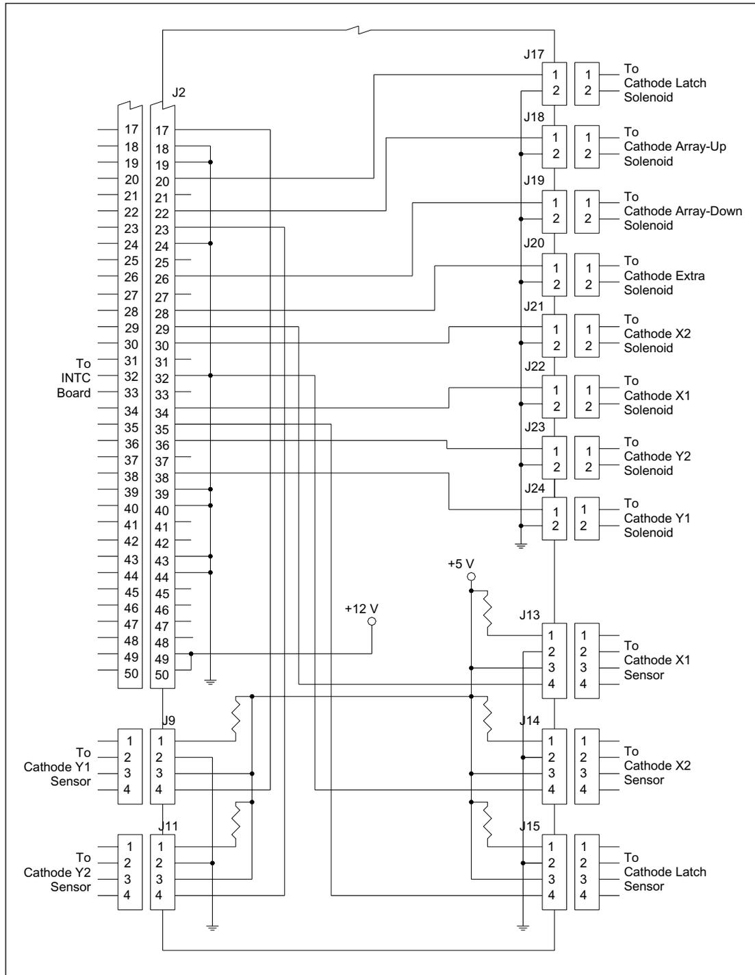
Figure 5-61. Cathode Connector Board Connector Detail Diagram (MB 2000) (Sheet 2 of 2).
