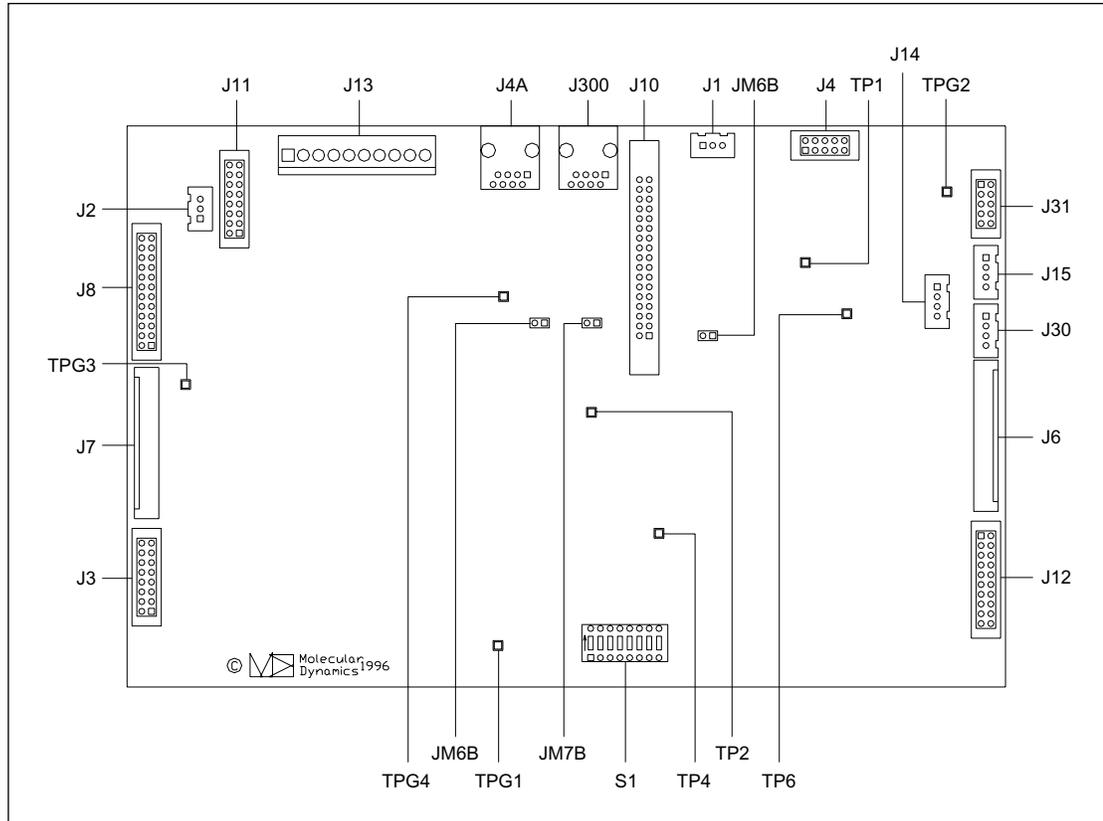
Figure 5-38. INTC Board Component Layout Diagram.
