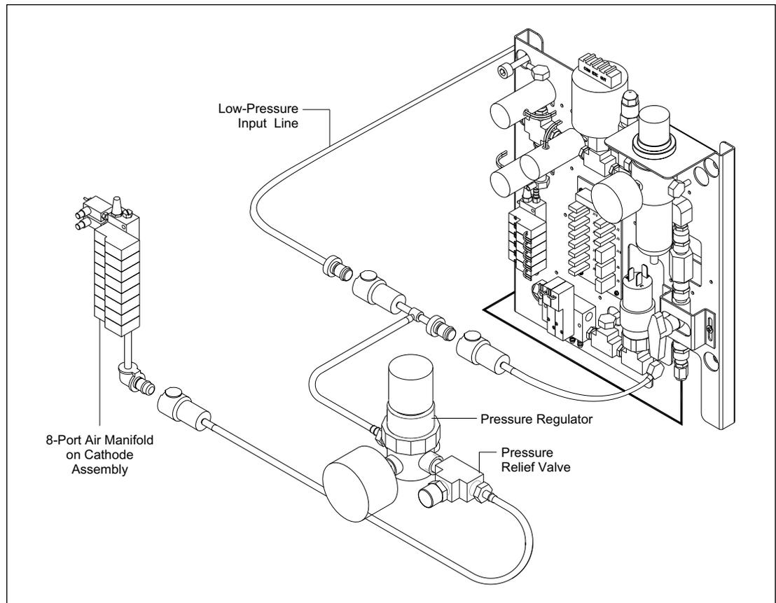
Figure 4-56. Pneumatic Assembly (MB 2000).
