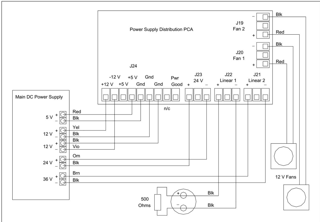
Figure 5-11. Power Supply Box DC Distribution Block Diagram (CE 2001).
