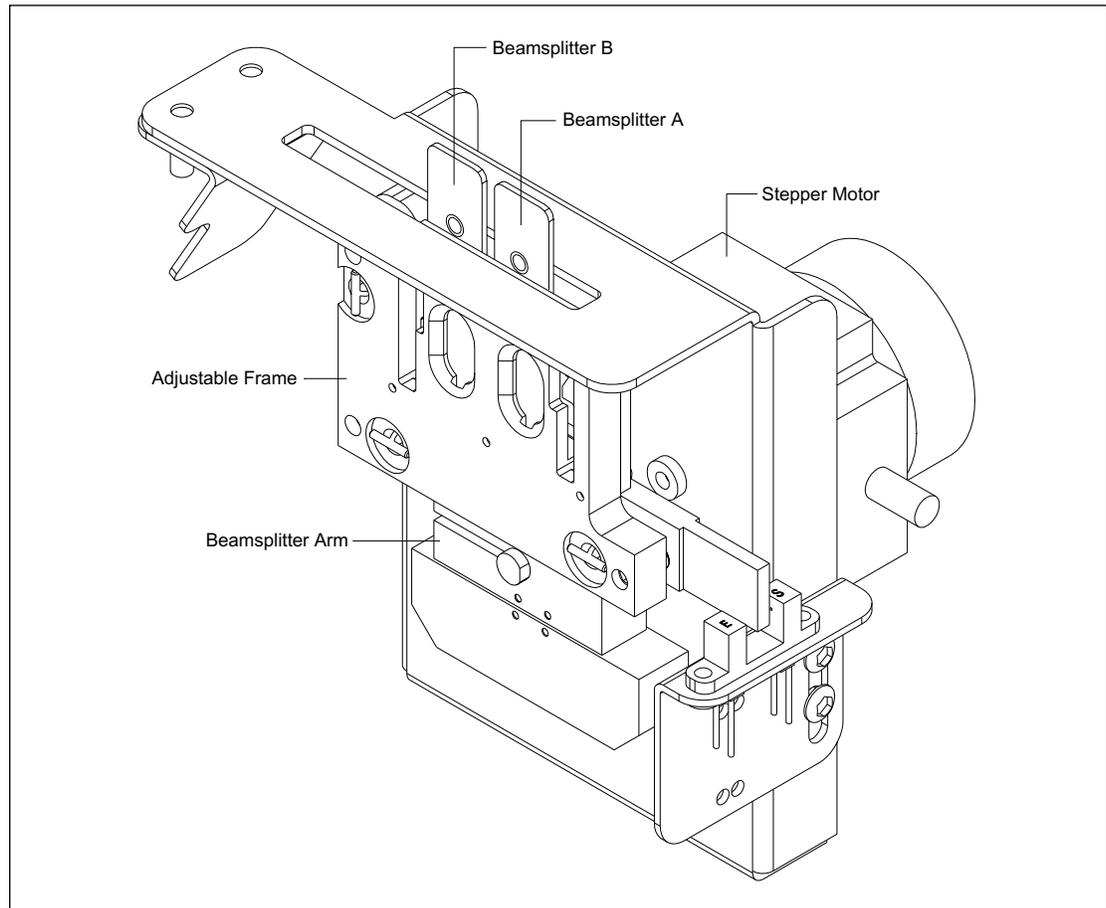
Figure 4-35. Secondary Beamsplitter Changer Assembly.
