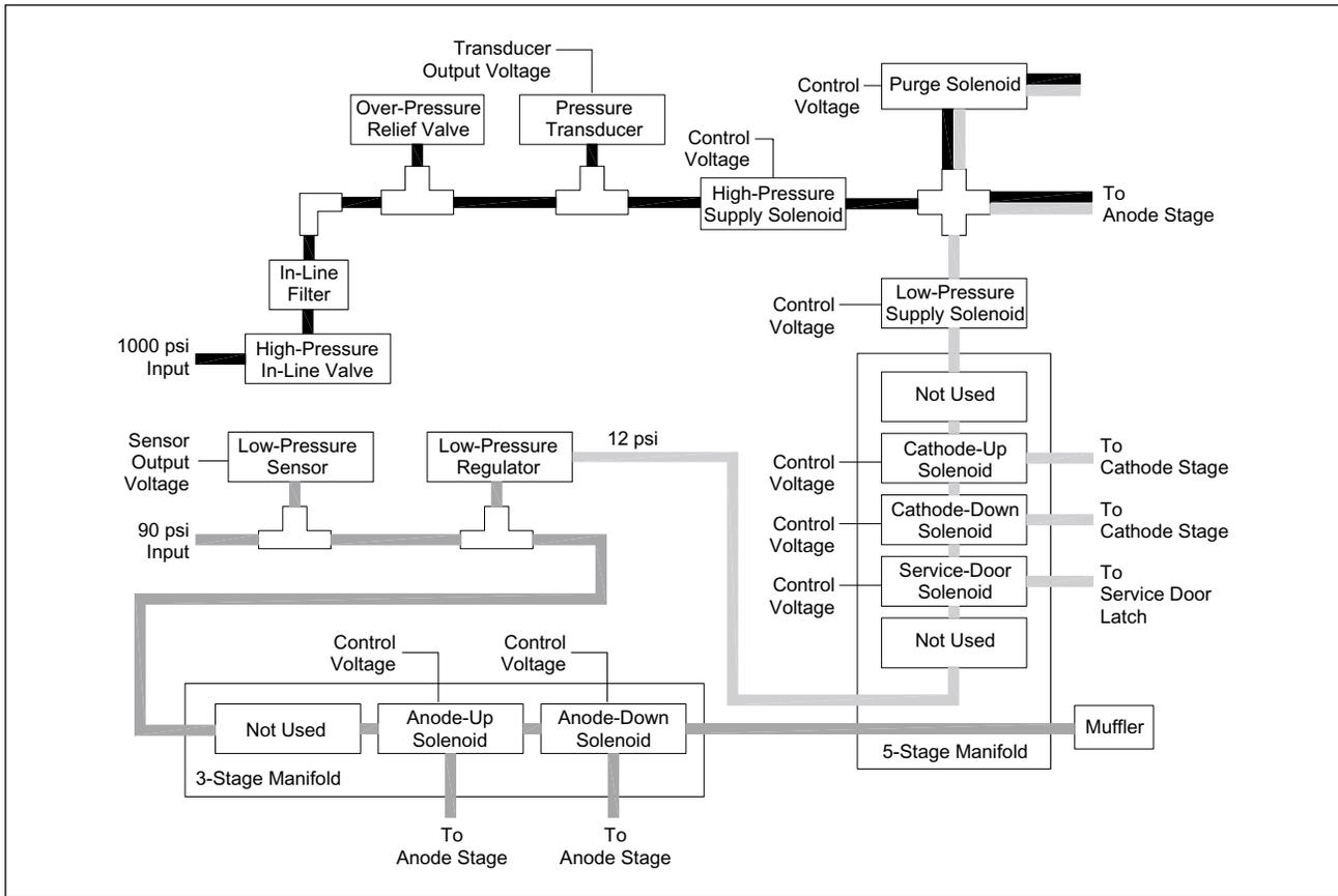
Figure 2-6. Pneumatics, Simplified Block Diagram.
