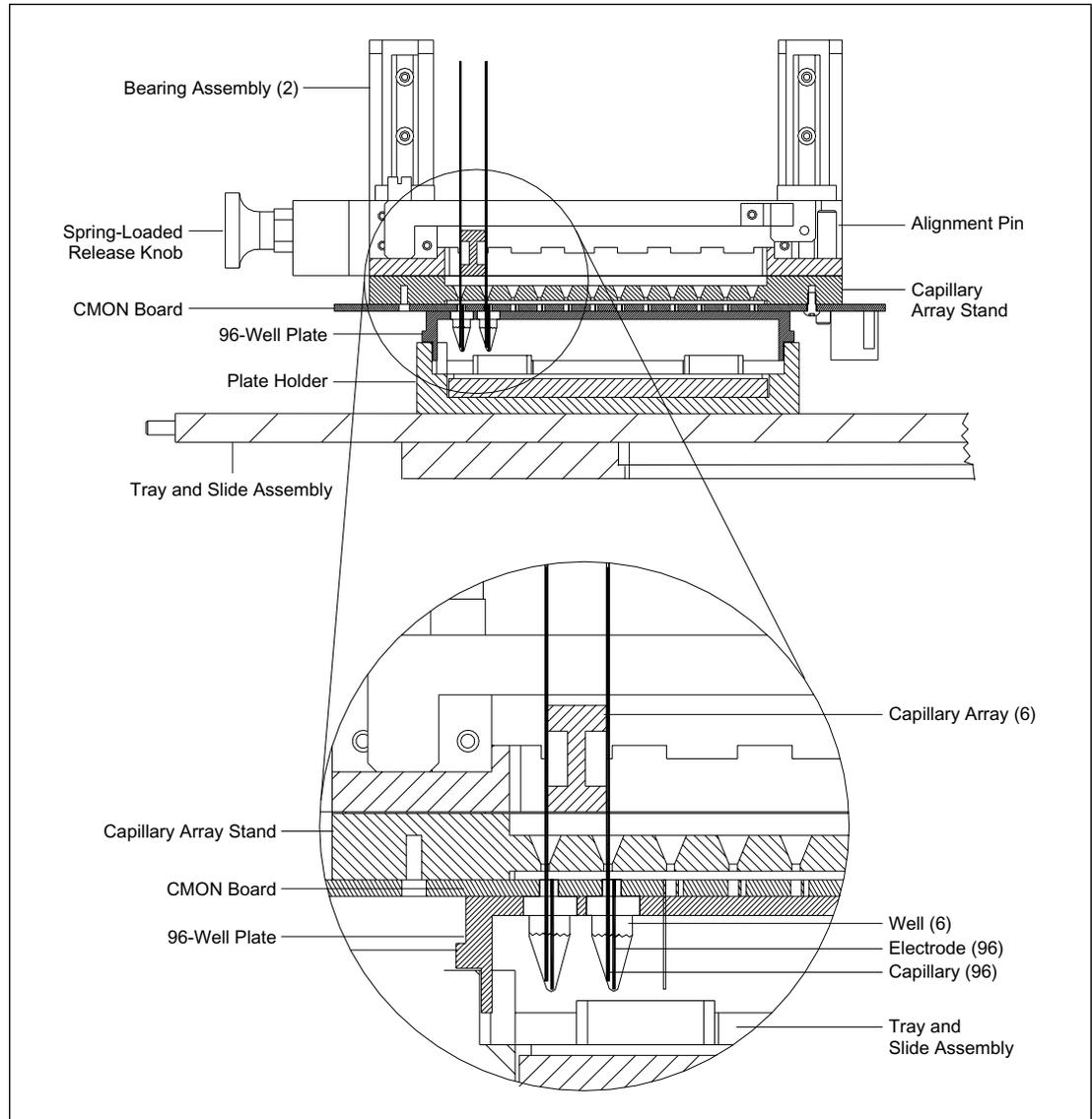
Figure 4-44. Cathode Assembly, Cross Section.
