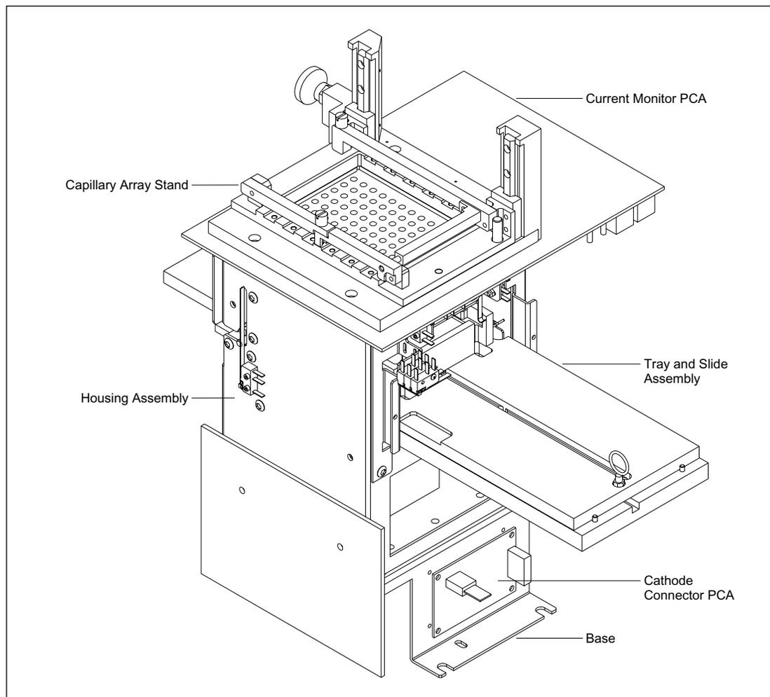
Figure 4-41. Cathode Assembly.
