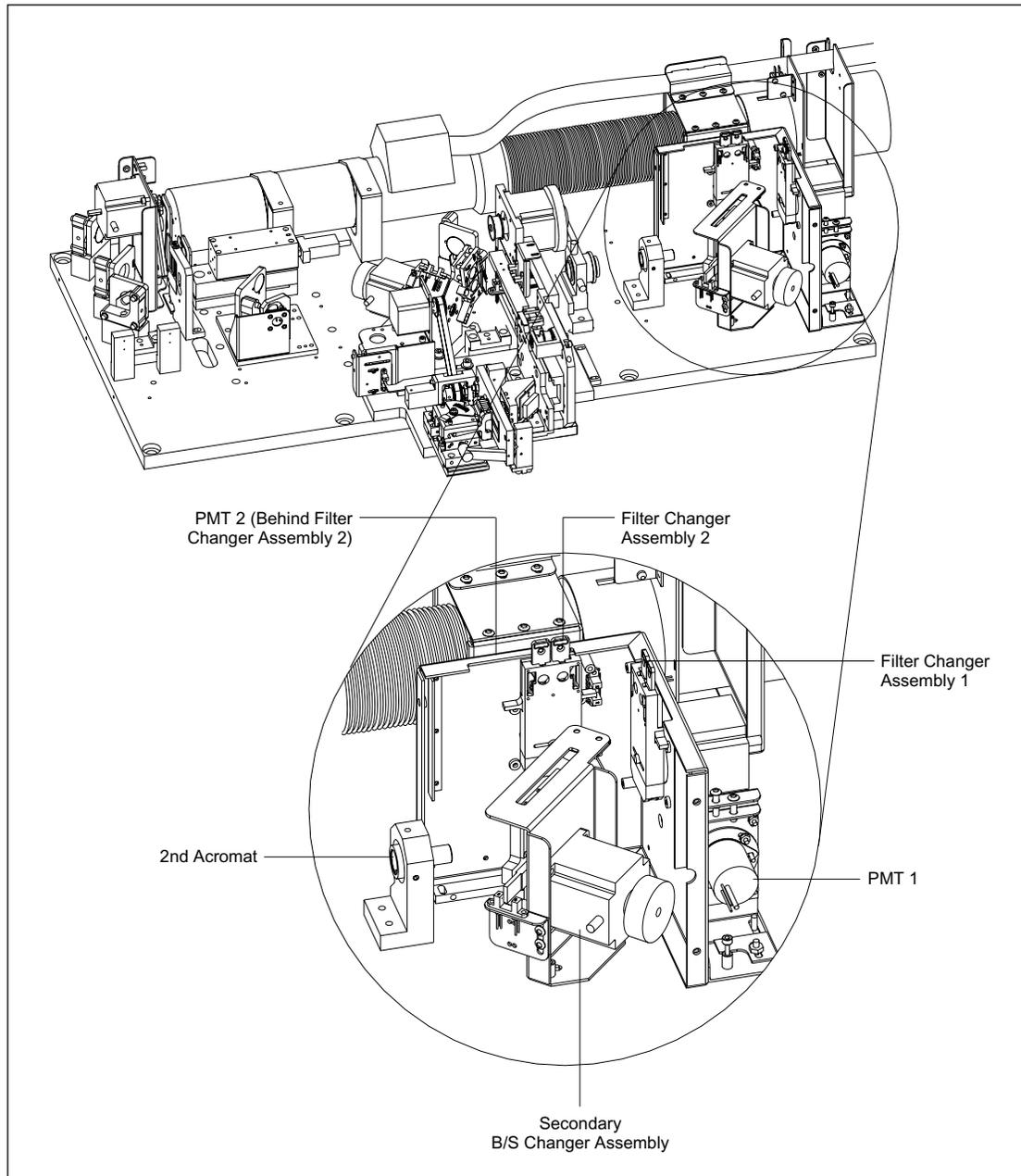
Figure 4-18. Optical Components Assembly (Sheet 3 of 3).
