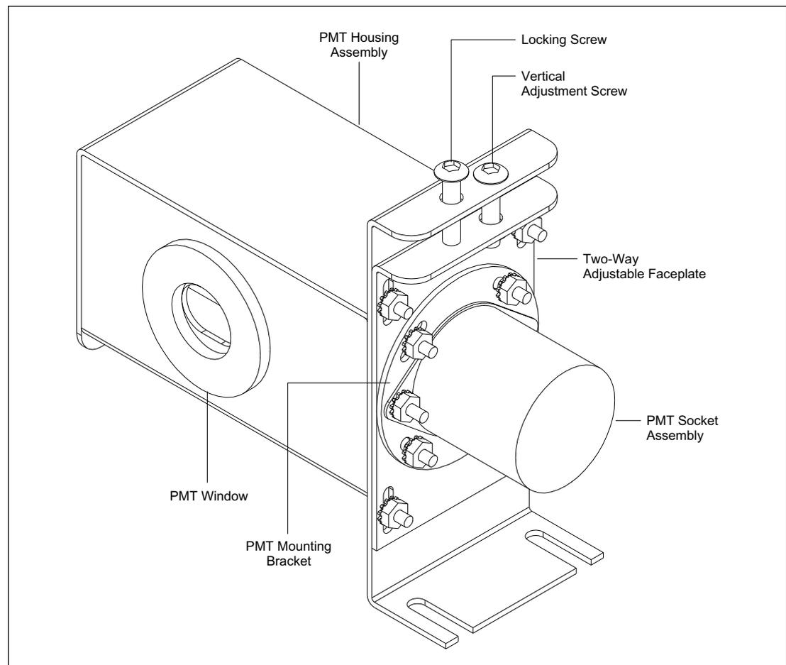
Figure 4-39. PMT Assembly.
