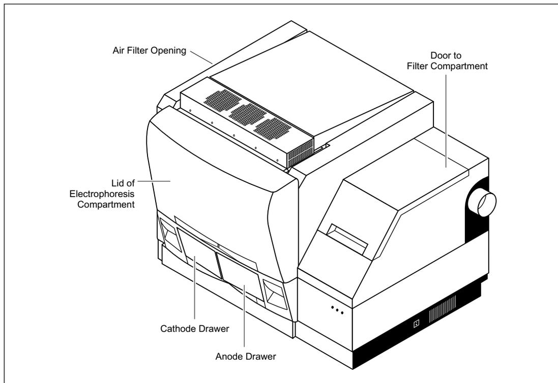
Figure 6-1. Instrument Access Ports.
