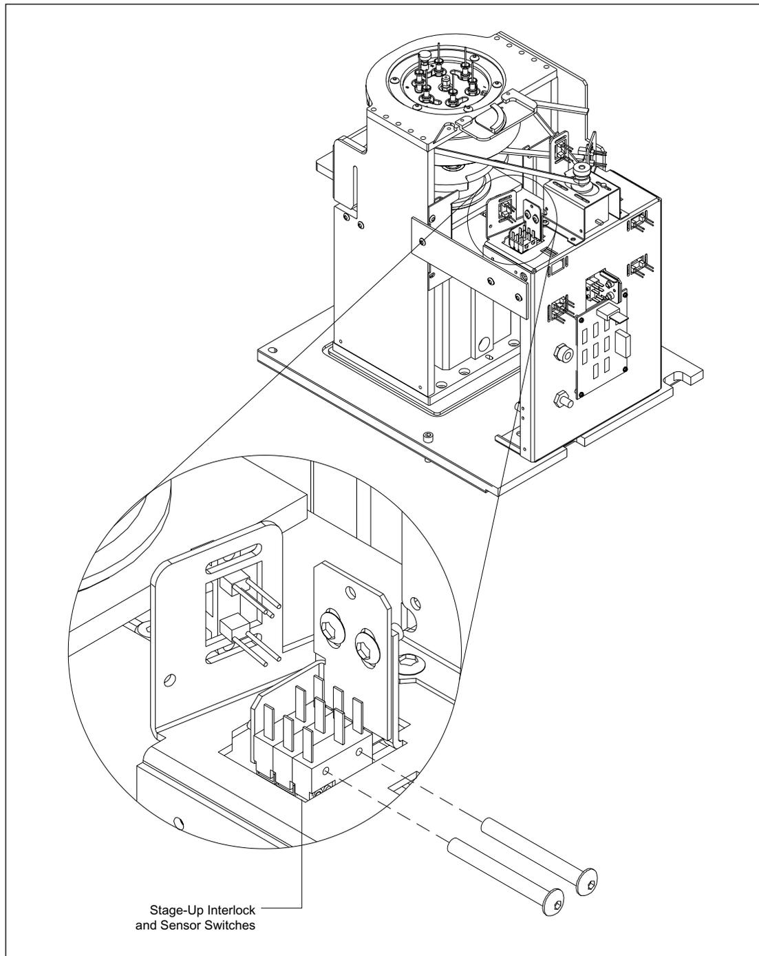
Figure 9-85. Anode Stage-Up Interlock and Sensor Switch Mounting.
