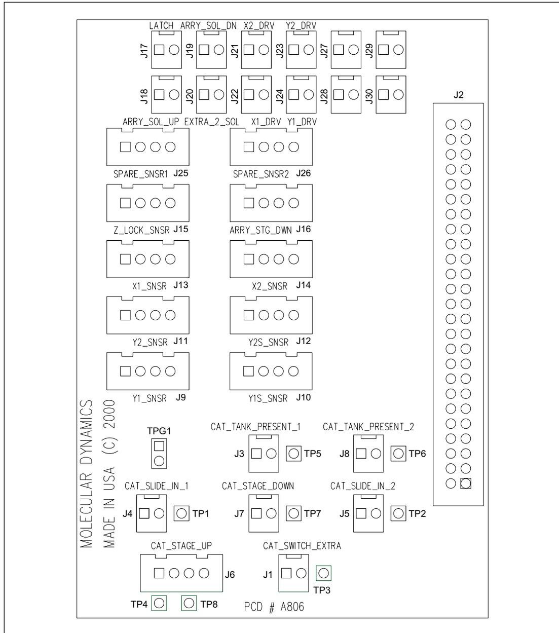
Figure 5-59. Cathode Connector Board Component Layout Diagram (MB 2000).
