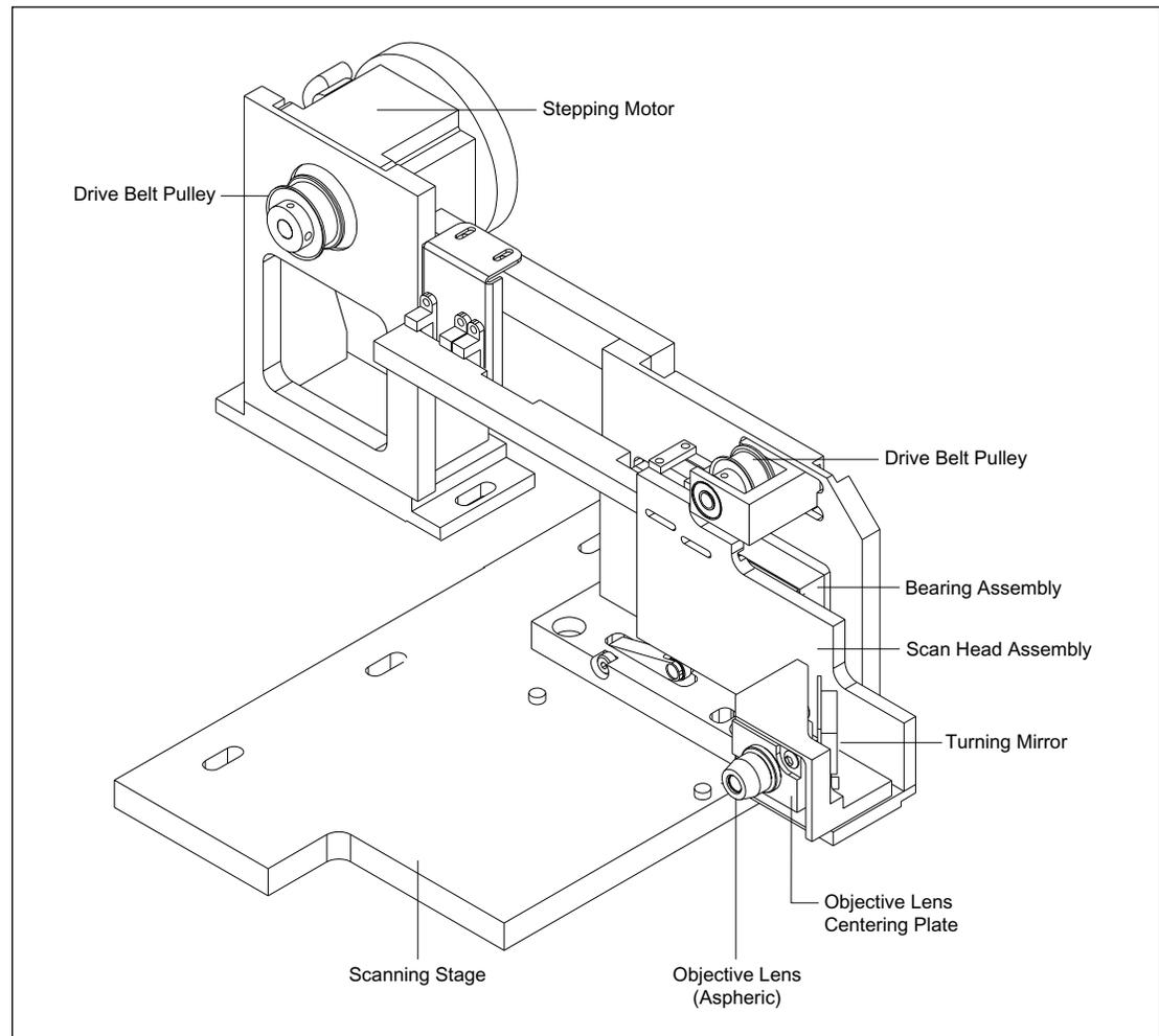
Figure 3-18. Scanning Stage.
