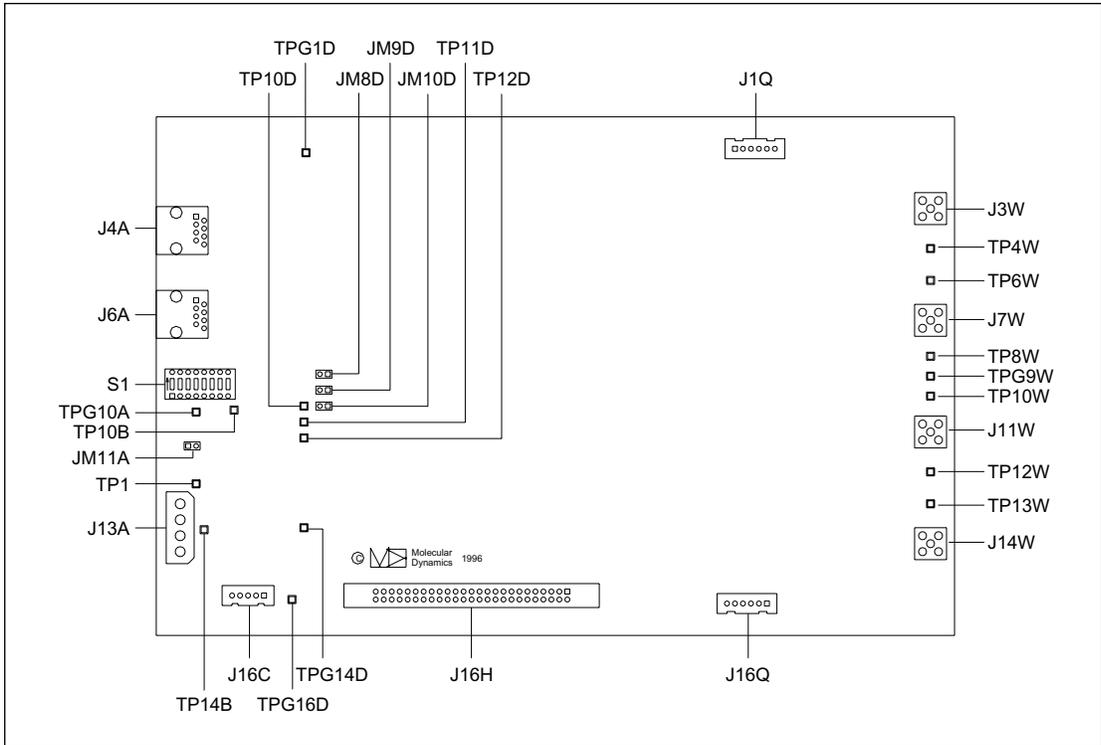
Figure 5-52. ADAQ Board Component Layout Diagram.
