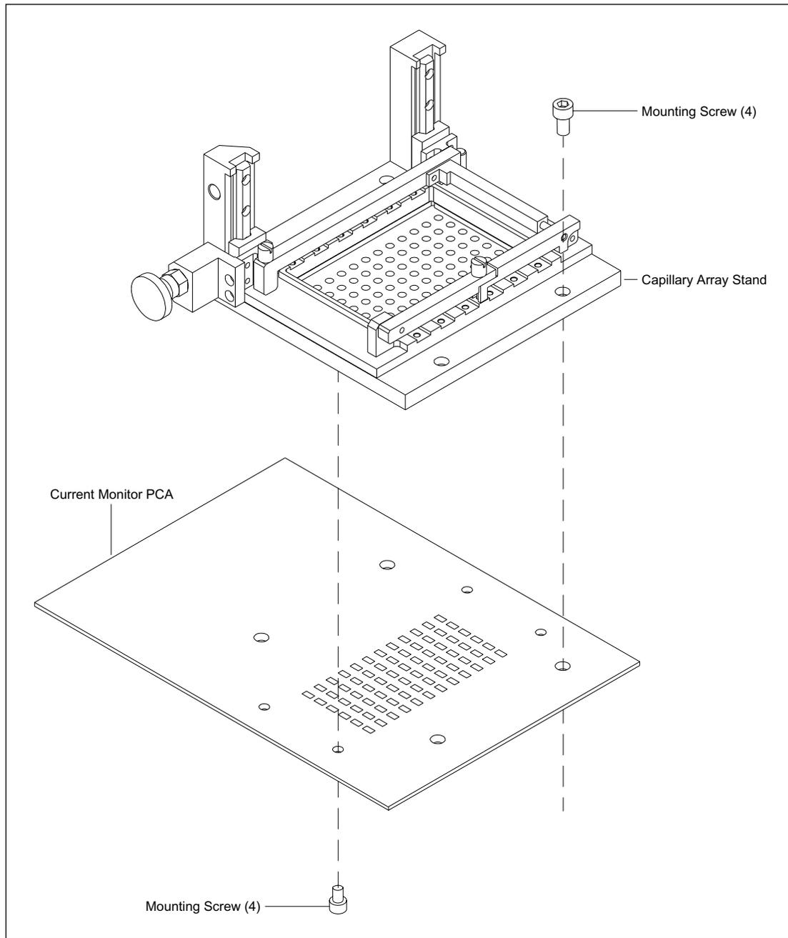
Figure 9-68. Array Stage and CMON Board Mounting.
