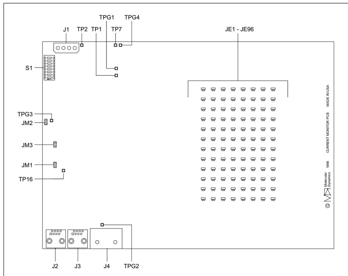
Figure 5-49. CMON Board Component Layout Diagram.
