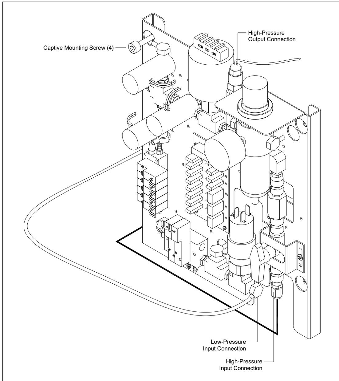
Figure 9-93. Nitrogen Pressure Manifold.
