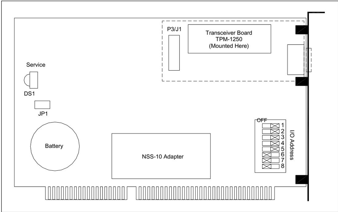
Figure 5-21. Neuron Network Control Board Component Layout Diagram.
