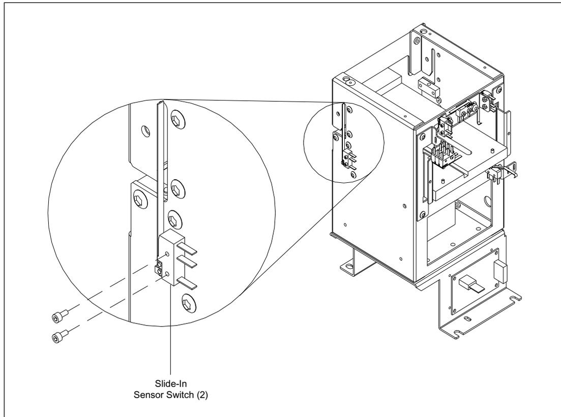
Figure 9-69. Cathode Slide-In Sensor Mounting.
