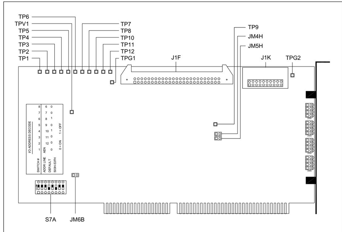
Figure 5-23. PC Interface Board Component Layout Diagram.
