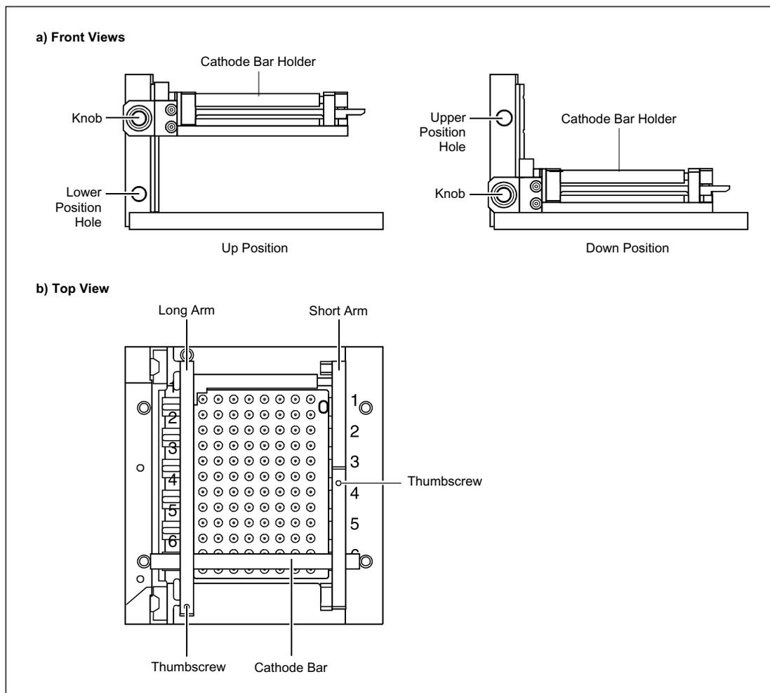
Figure 3-5. Cathode Array Stand.
