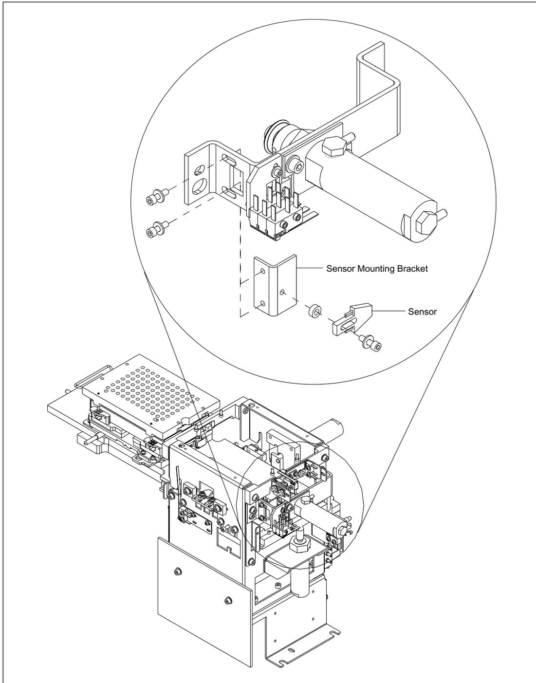
Figure 9-78. Indexer Y-Position Lock Sensor Mounting (MB 2000).
