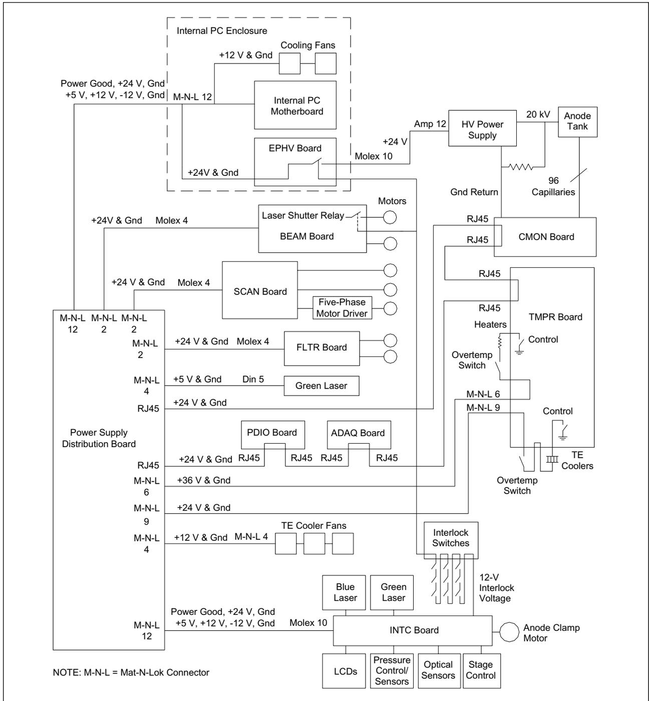
Figure 5-13. Instrument DC Distribution Block Diagram.
