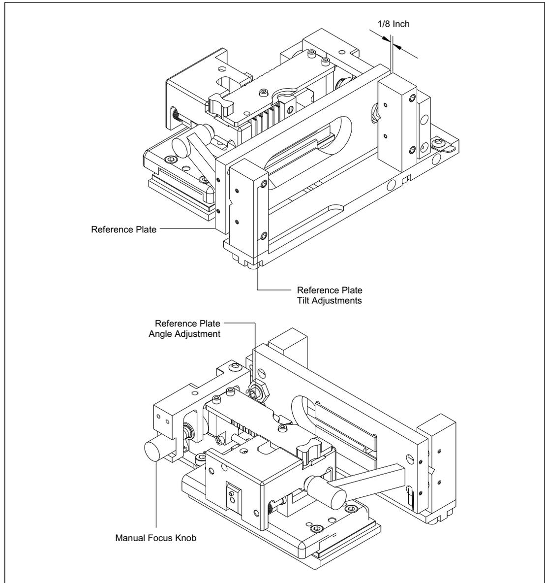
Figure 8-6. Capillary Clamp Assembly.
