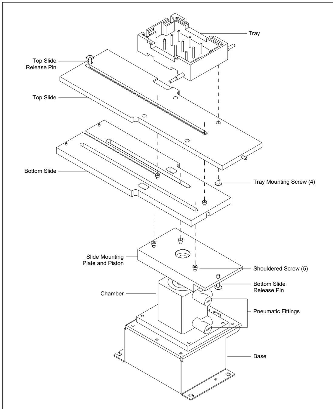
Figure 4-45. Cathode Piston Assembly.
