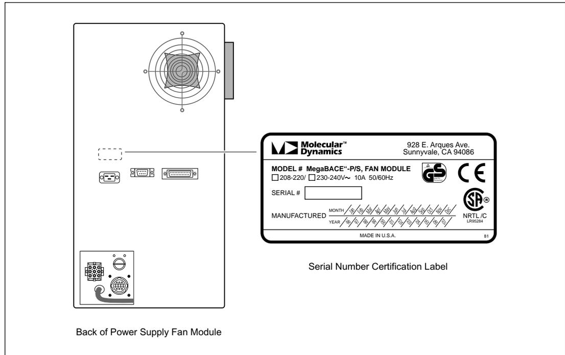
Figure 6-14. Location of the Serial Number Certification Label on the Power Supply Fan Module.
