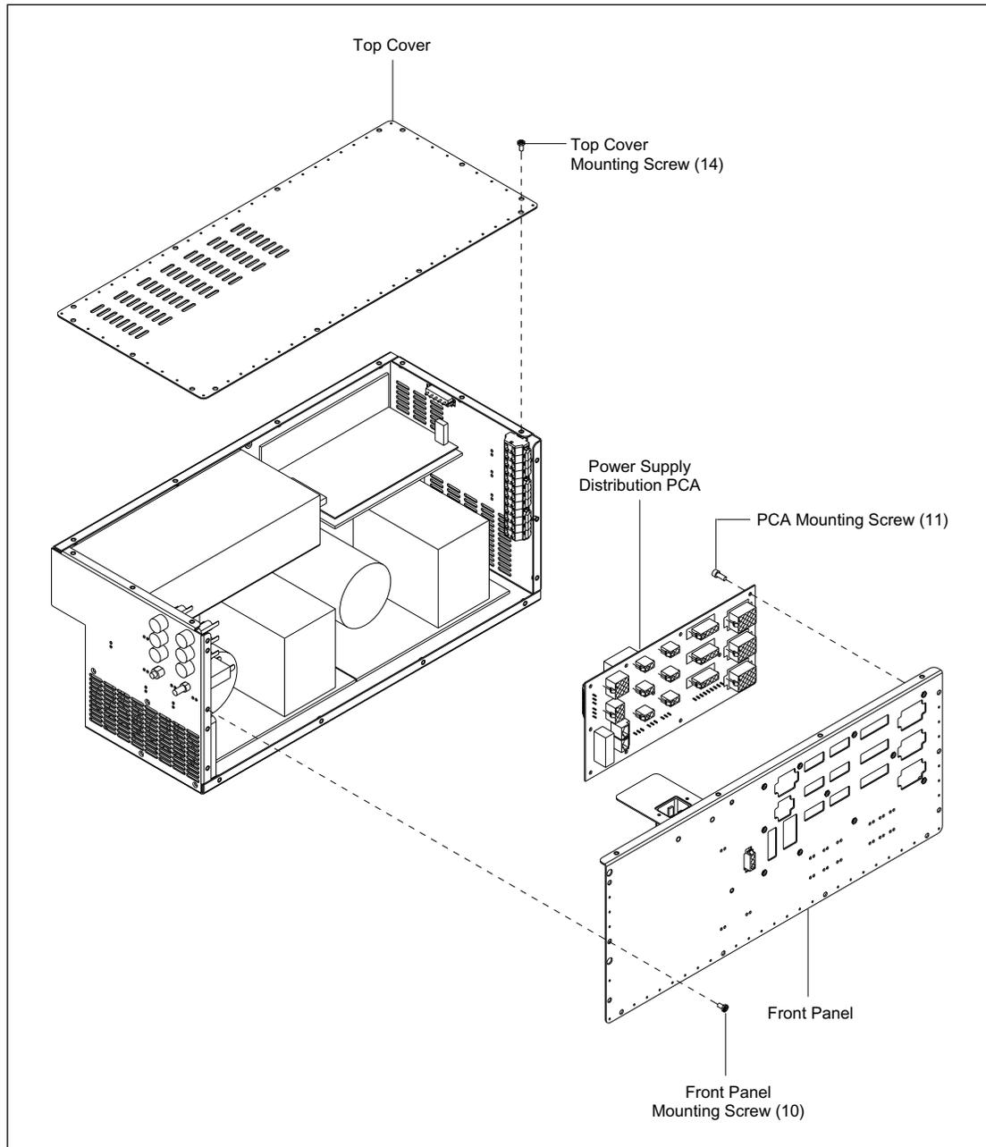
Figure 9-12. Power Supply Distribution Board Mounting.
