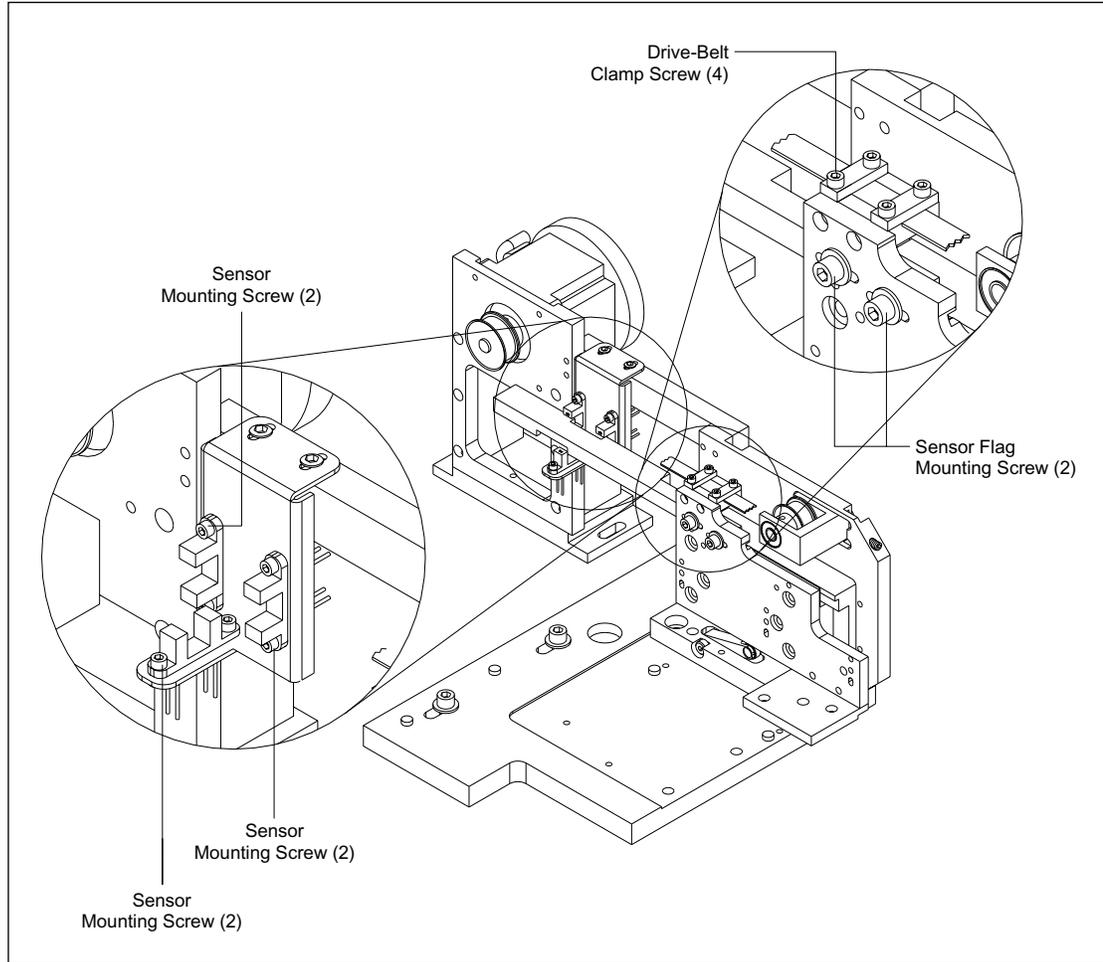
Figure 9-53. Scan Head Position Sensor Mounting.
