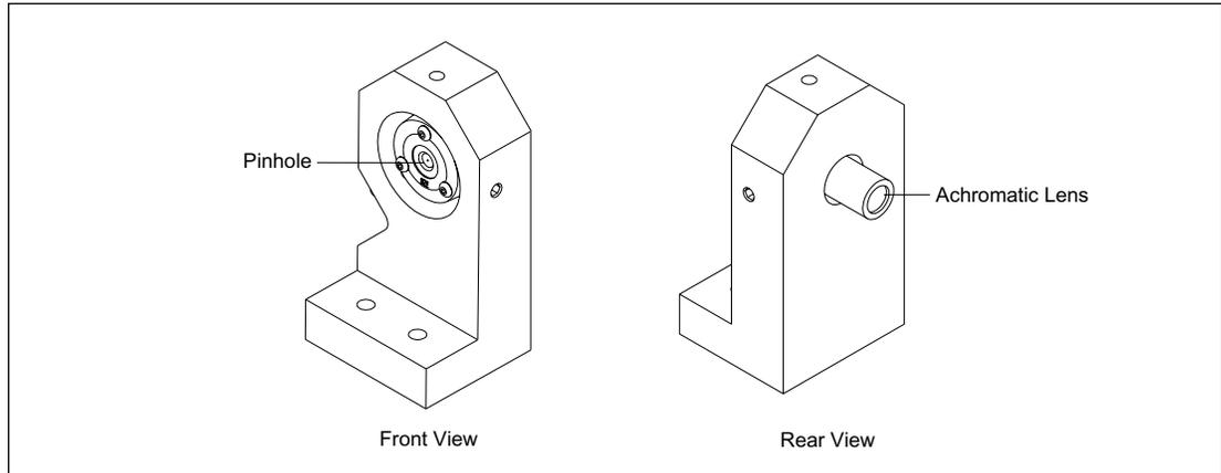
Figure 3-21. Pinhole and Second Achromatic Lens.
