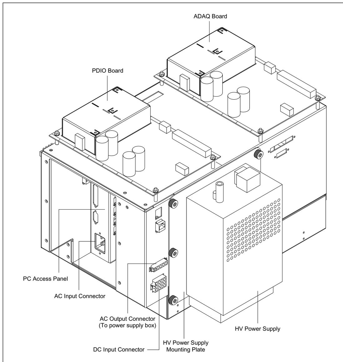
Figure 4-12. Internal Computer Assembly.
