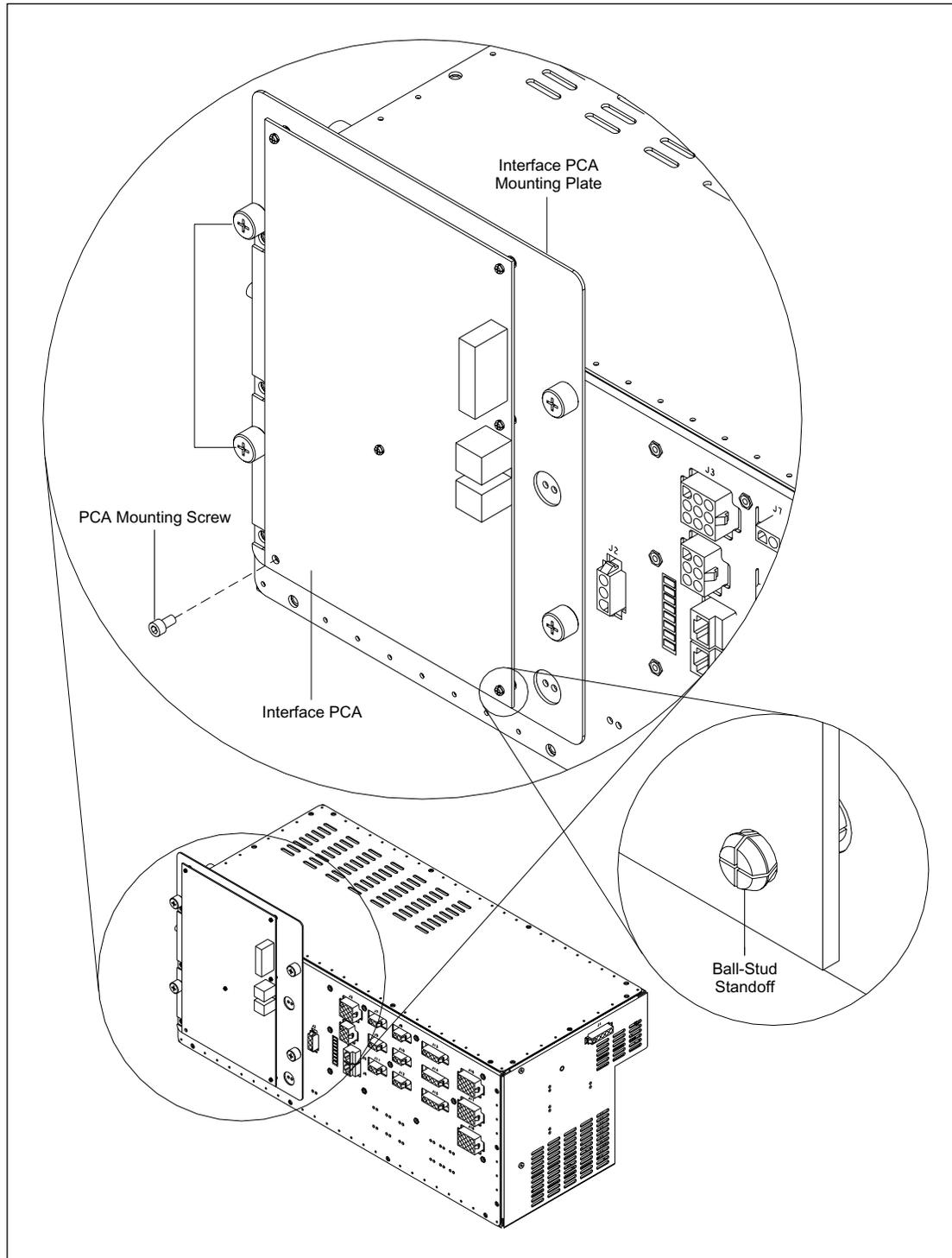
Figure 9-11. INTC Board Mounting.
