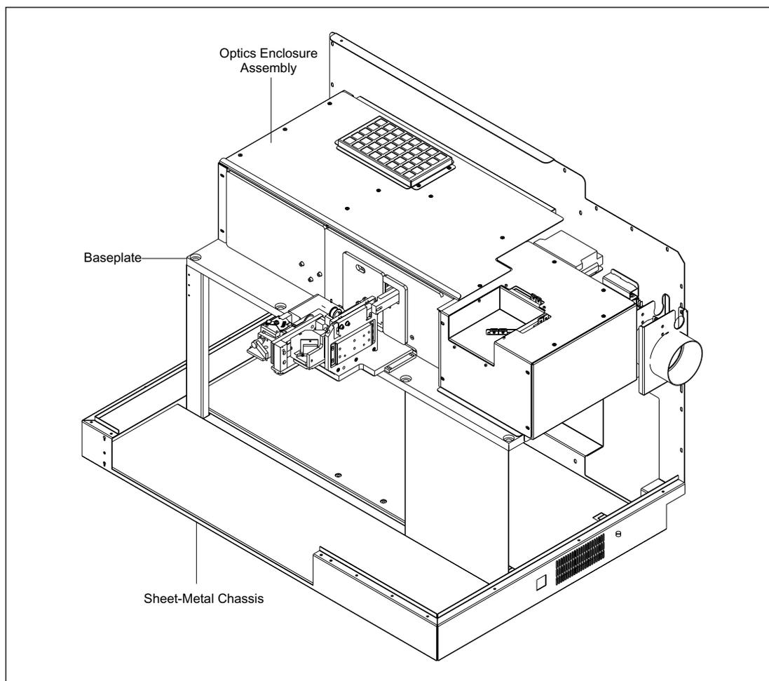
Figure 4-14. Optics Plate Assembly.
