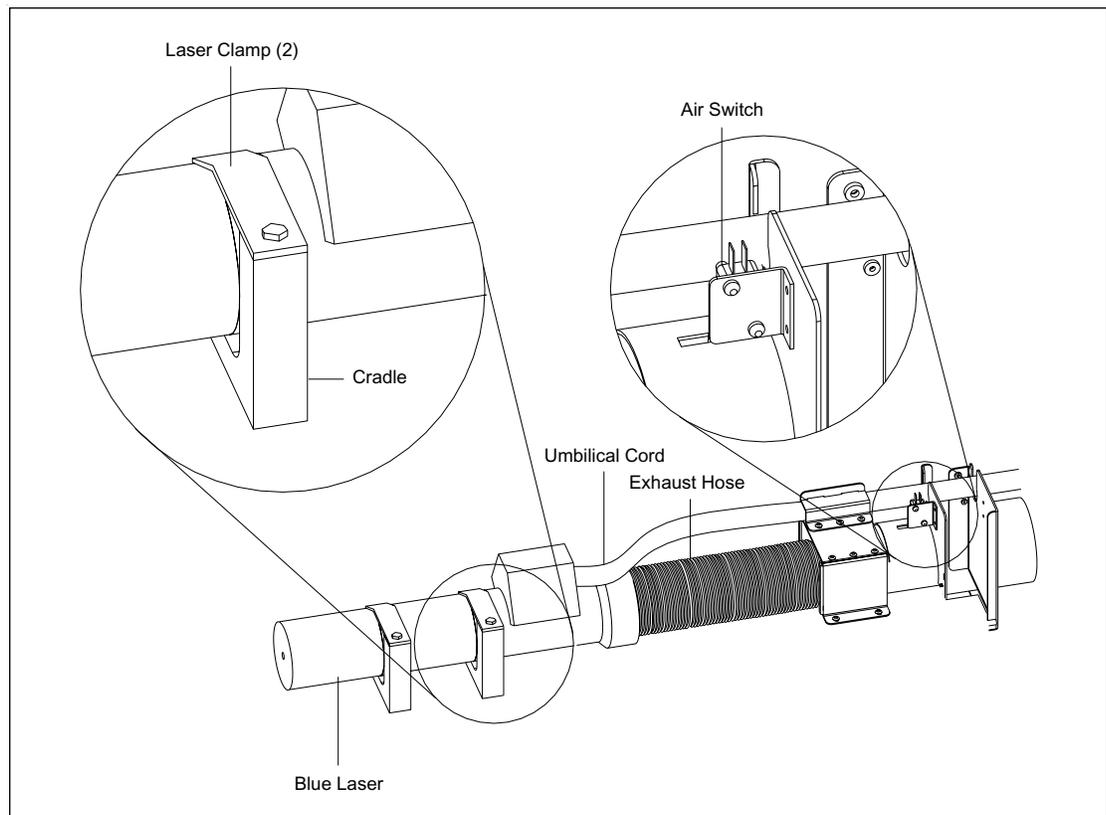
Figure 4-19. Blue Laser Assembly.
