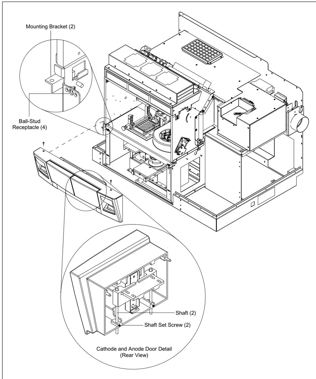
Figure 9-7. Front Panel Assembly Mounting.
