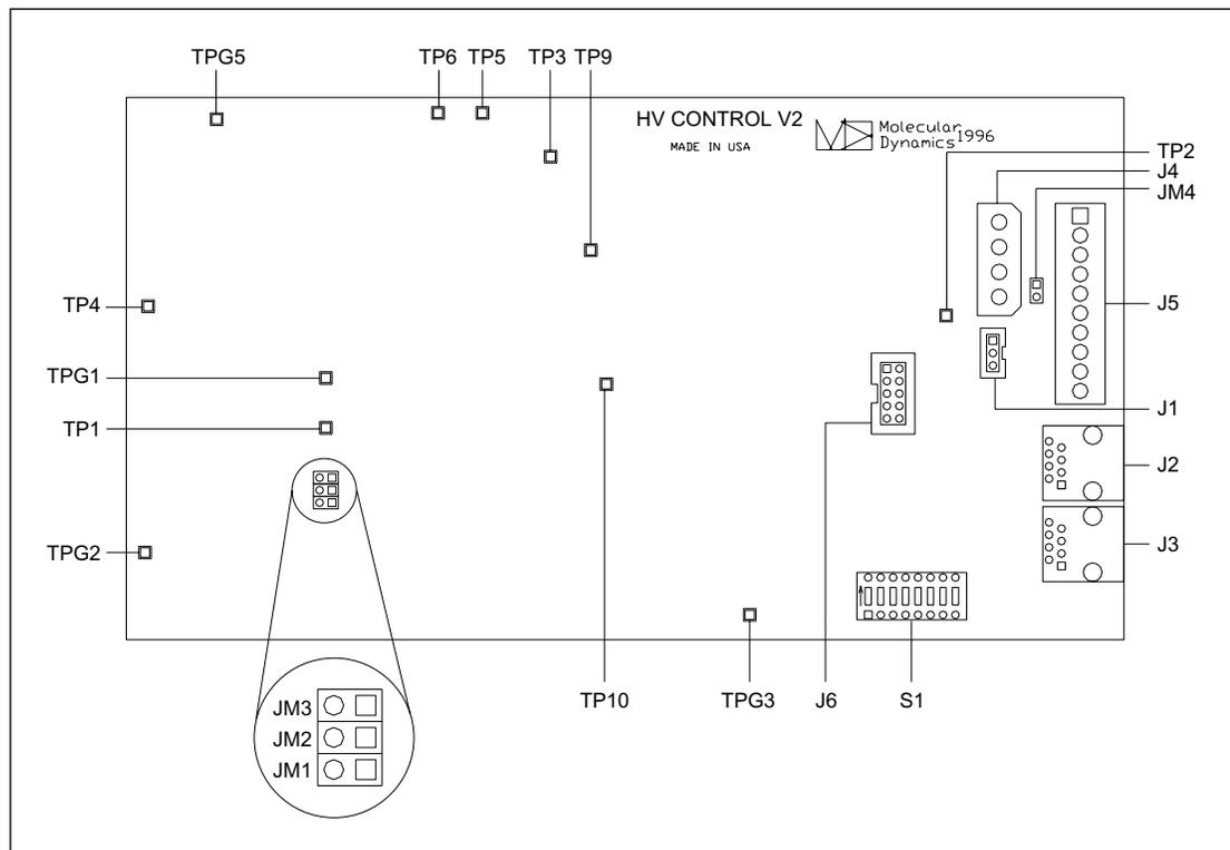
Figure 5-26. EPHV Board Component Layout Diagram.
