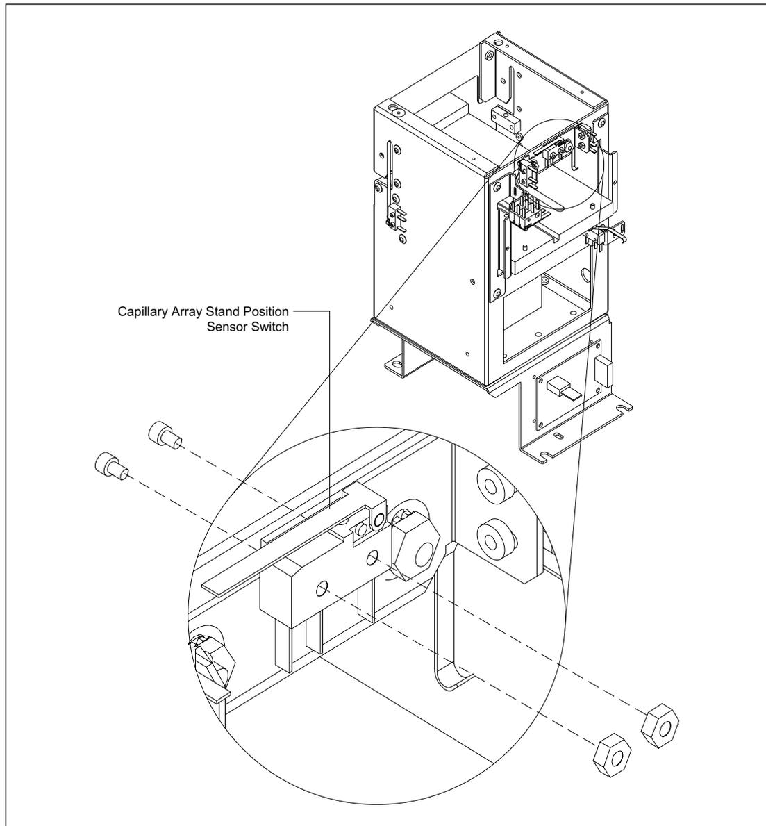
Figure 9-72. Array Stage Position Sensor Mounting.
