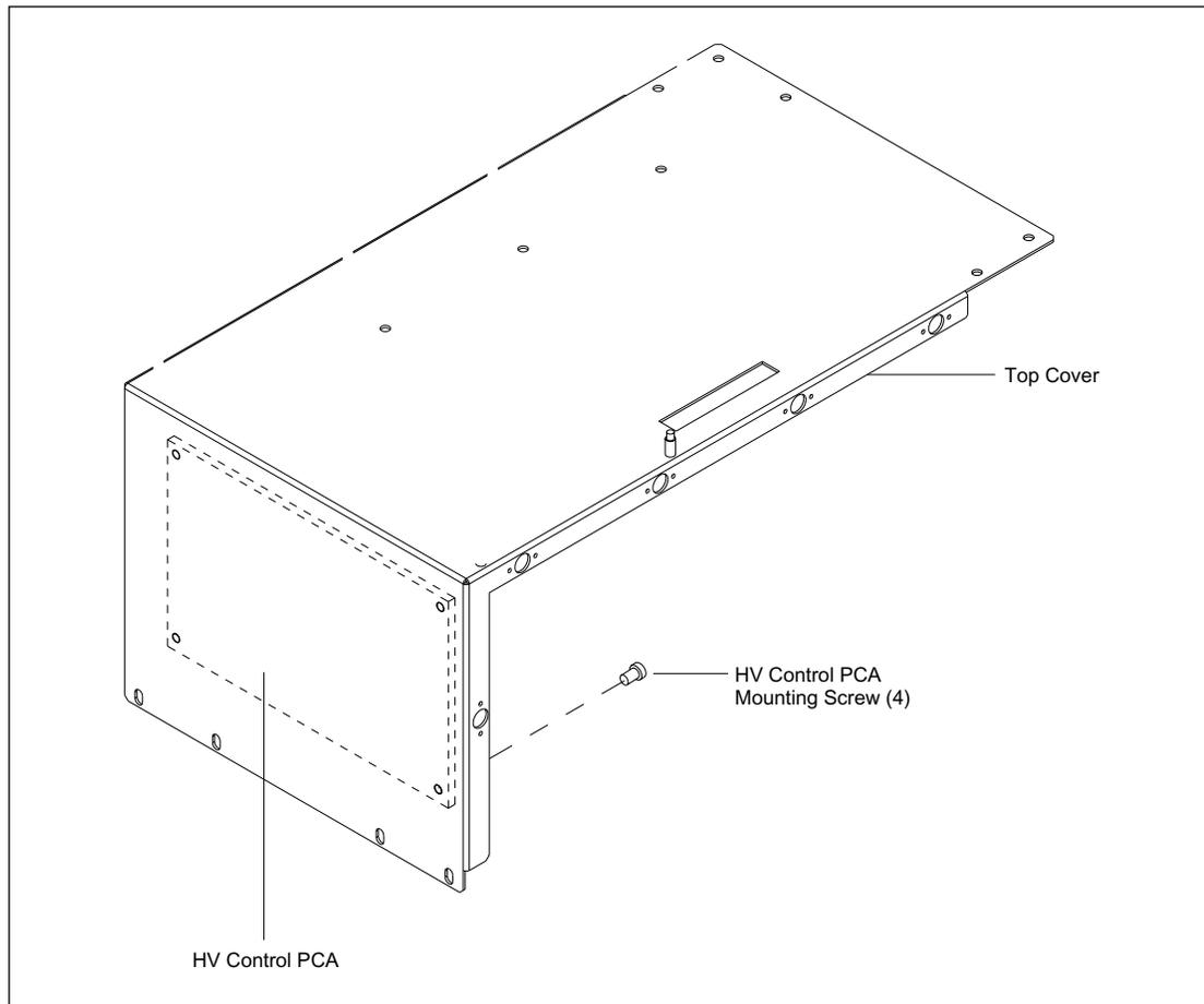
Figure 9-38. EPHV Board Mounting.
