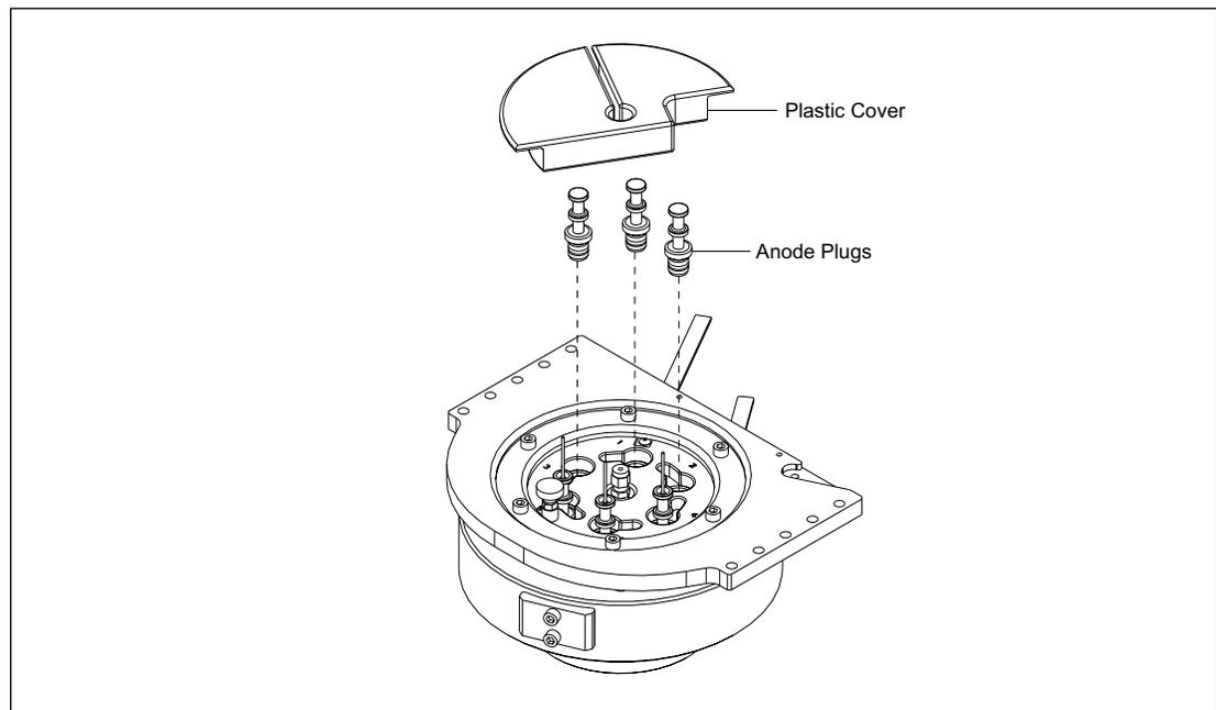
Figure 8-12. Anode Plugs and Plastic Anode Cover.
