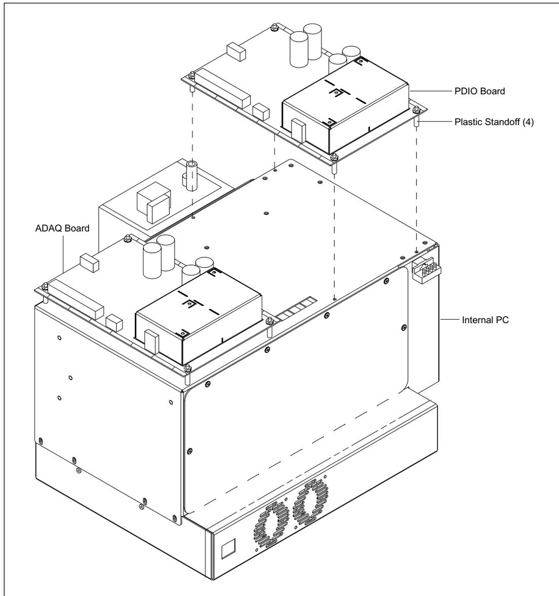
Figure 9-28. PDIO Board Mounting.
