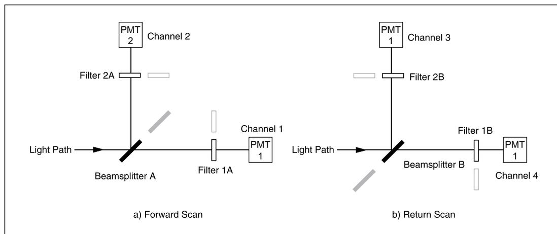
Figure 3-3. Emission Paths Functional Block Diagram.
