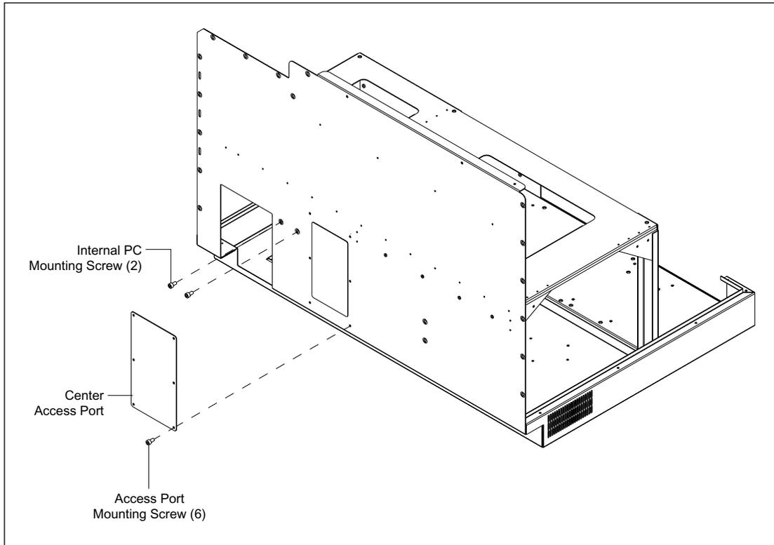
Figure 9-29. Internal Computer Mounting.
