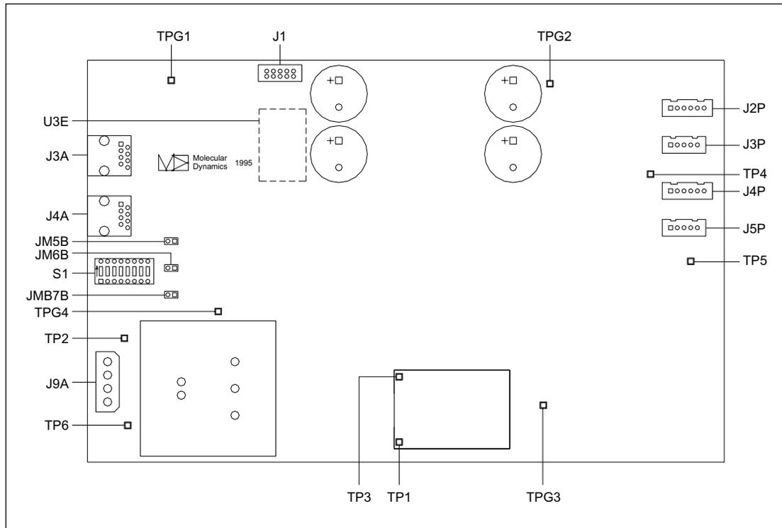
Figure 5-35. BEAM Board Component Layout Diagram.
