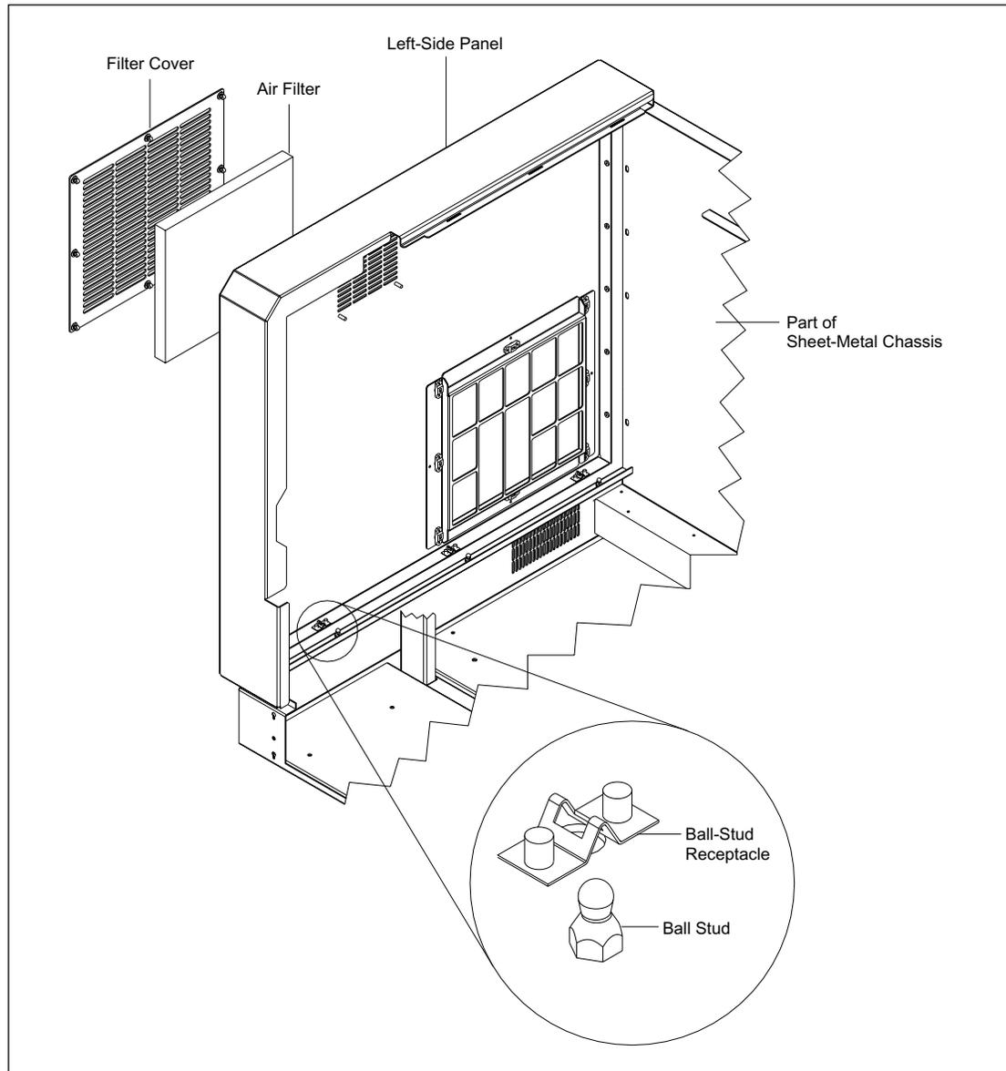
Figure 4-4. Left Panel Assembly.
