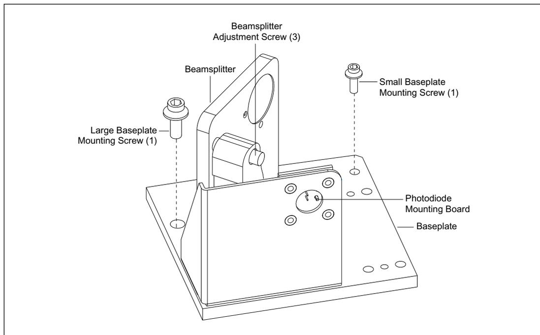
Figure 4-26. Capillary Detection Assembly.
