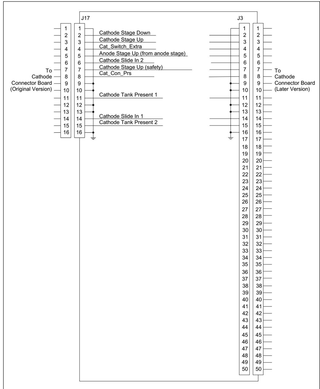
Figure 5-44. INTC Board Connector Detail Diagram (Later Model).
