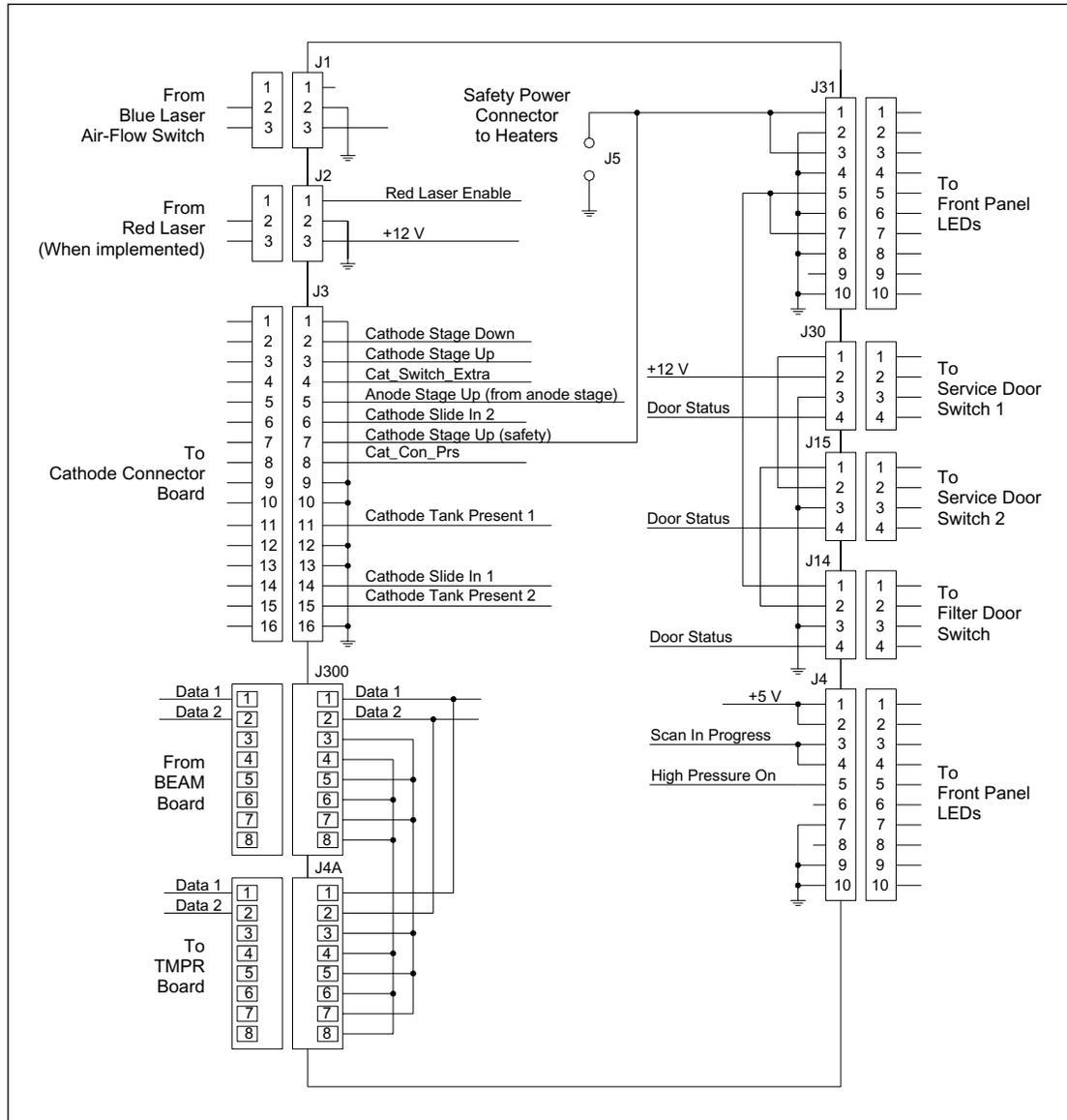
Figure 5-39. INTC Board Connector Detail Diagram (Sheet 1 of 3).
