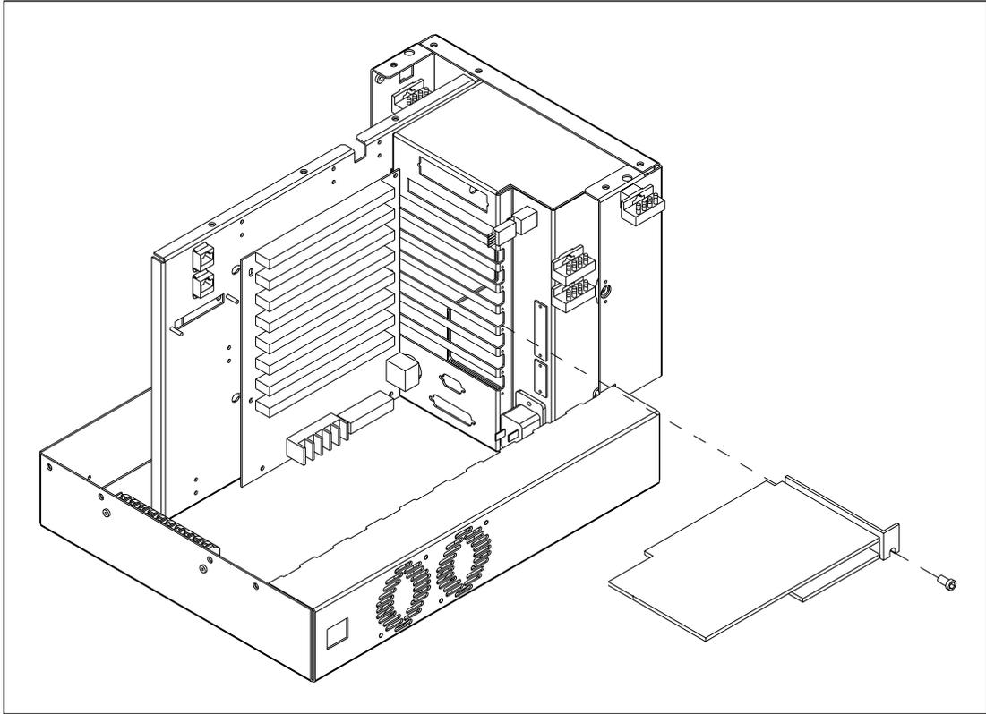
Figure 9-35. Echelon Network Interface Board Mounting.
