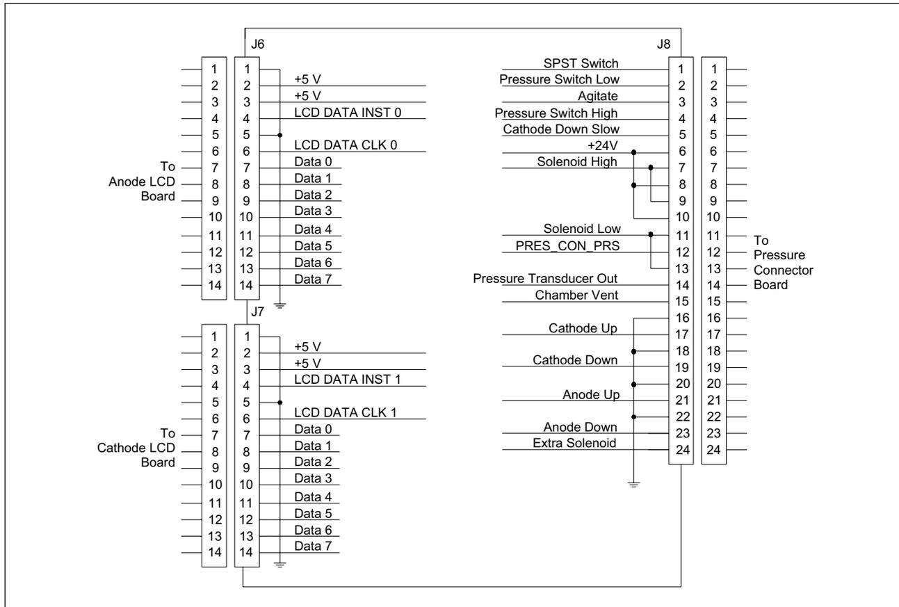
Figure 5-40. INTC Board Connector Detail Diagram (Sheet 2 of 3).
