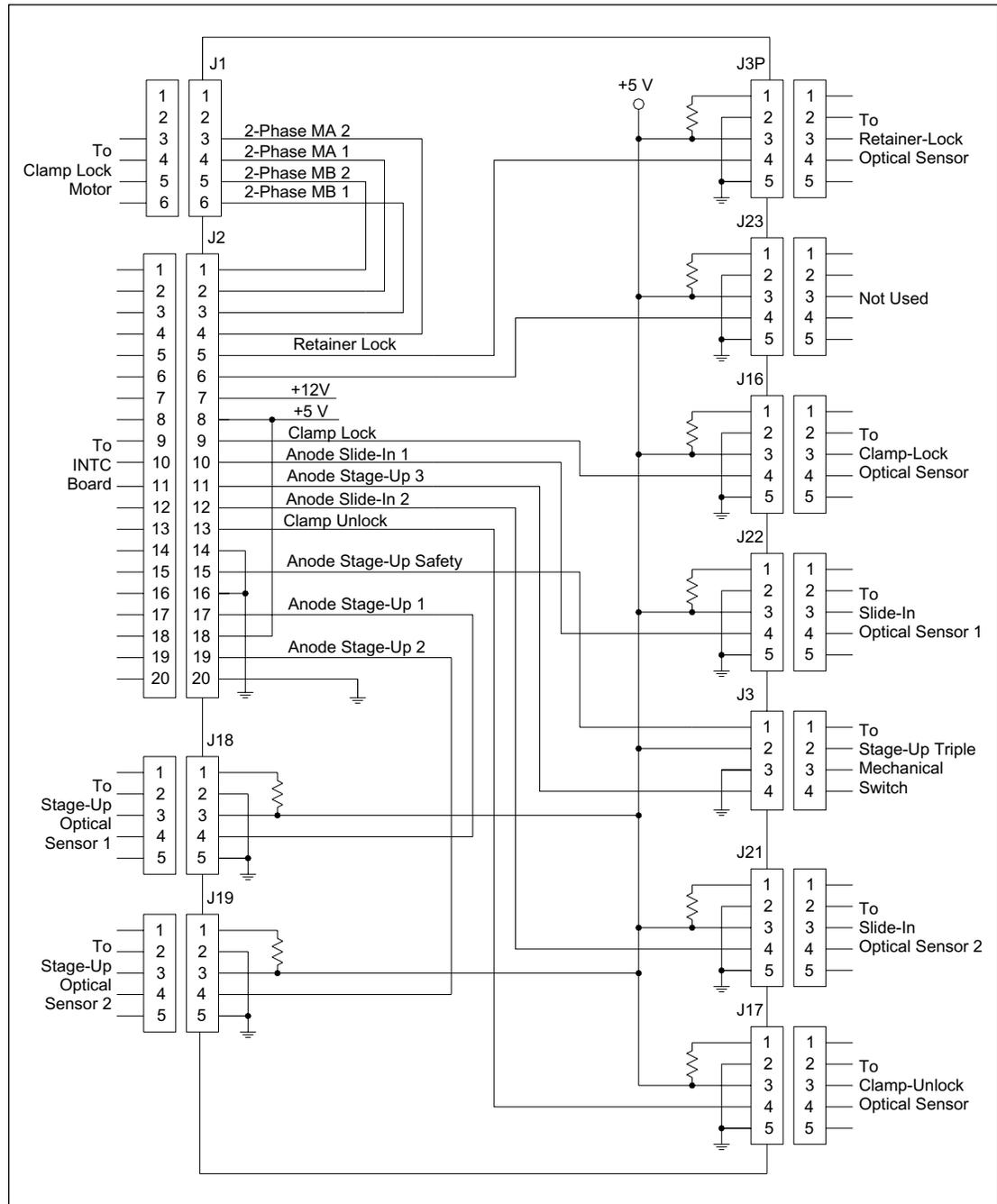
Figure 5-63. Anode Connector Board Connector Detail Diagram.
