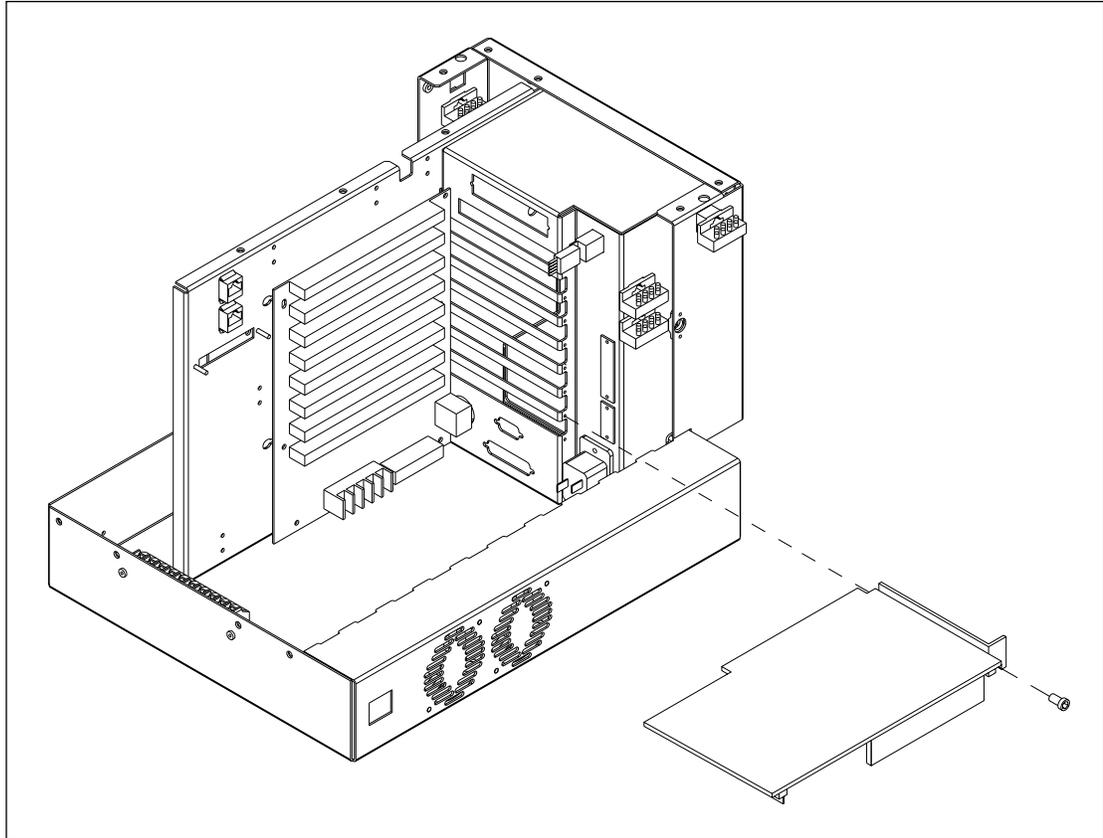
Figure 9-36. CPU Board Mounting.
