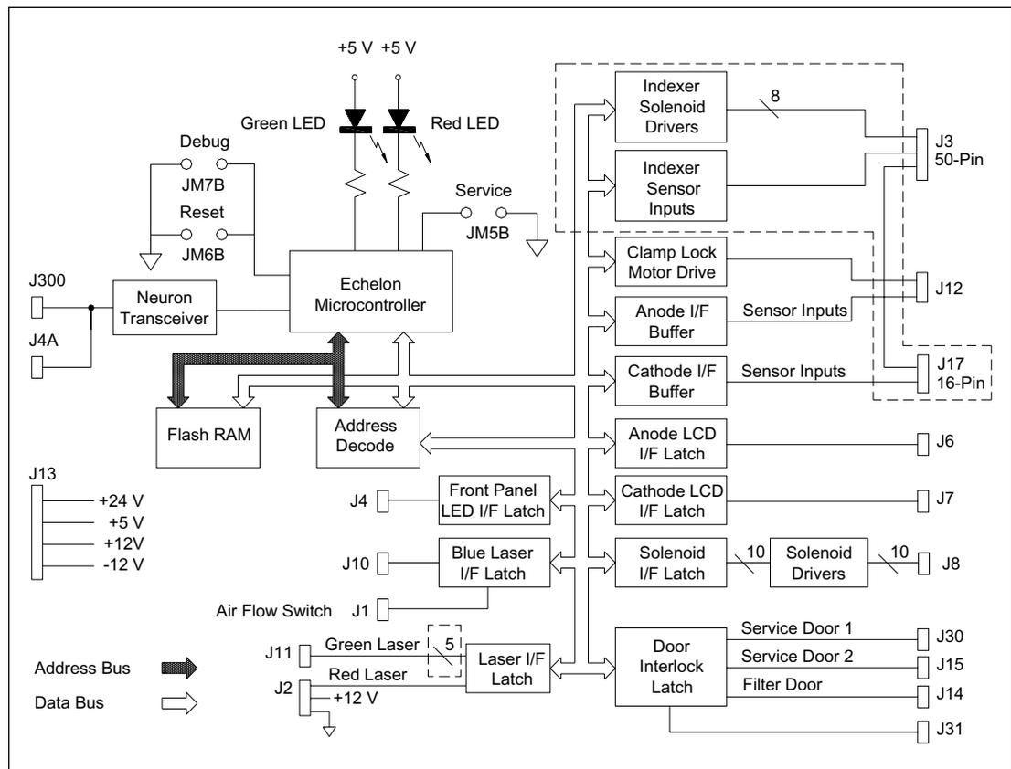
Figure 5-42. INTC Board Block Diagram (Later Model).
