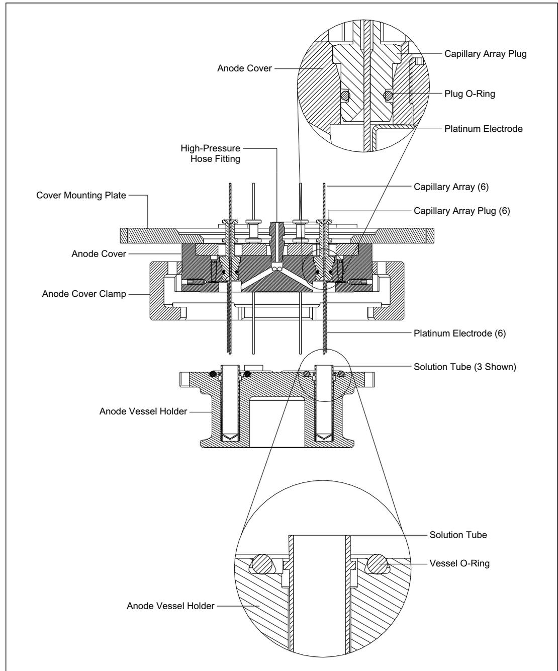
Figure 4-51. Anode Assembly, Cross Section.
