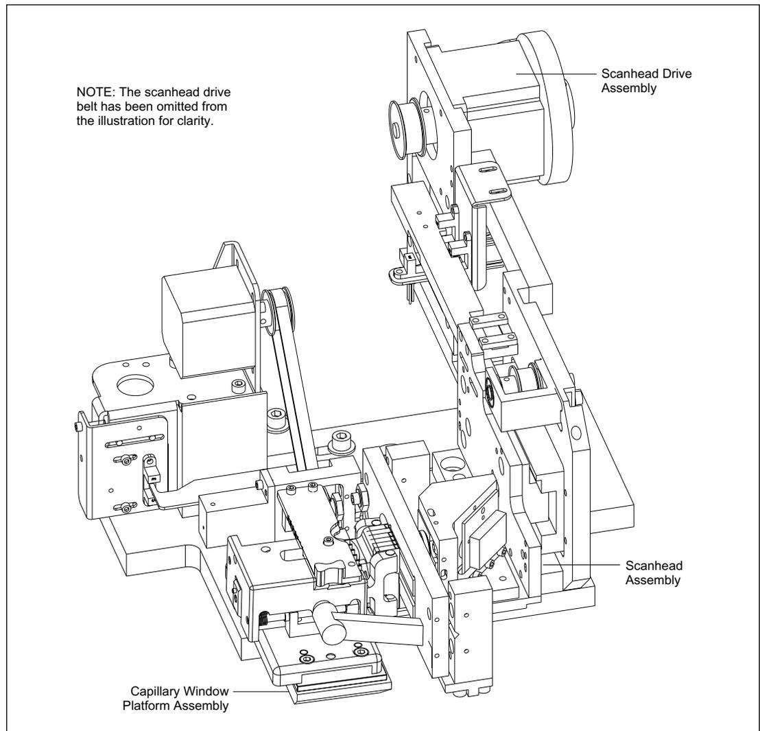
Figure 4-29. Scanning Stage Assembly.
