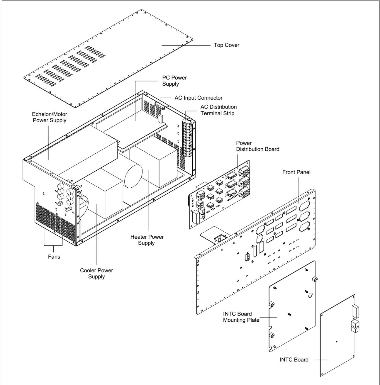
Figure 4-9. Power Supply Box Assembly.
