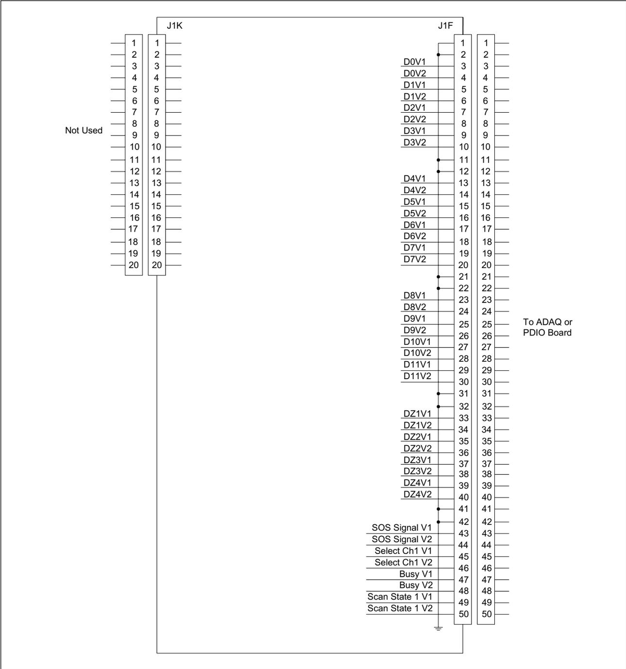
Figure 5-24. PC Interface Board Connector Detail Diagram.
