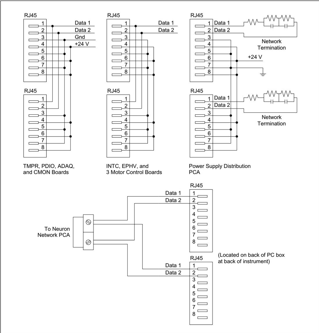
Figure 5-15. Neuron Network Connector Detail Diagram.
