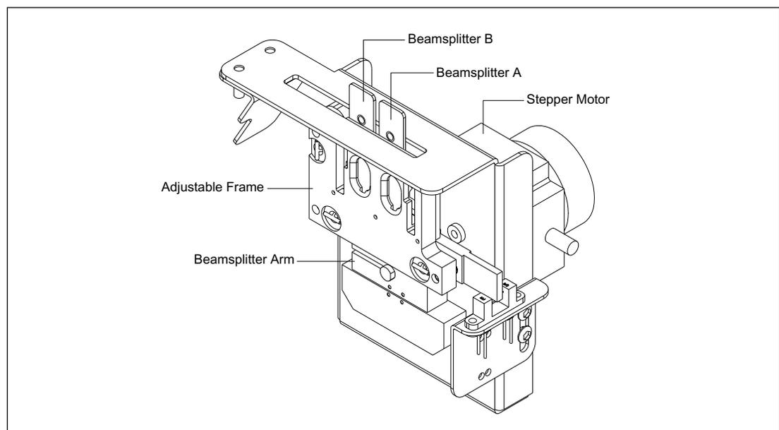
Figure 3-22. Secondary Beamsplitter Changer.
