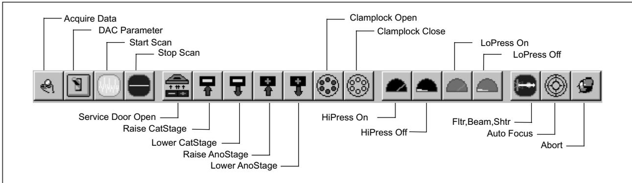
Figure 7-5. Instrument Control Area.
