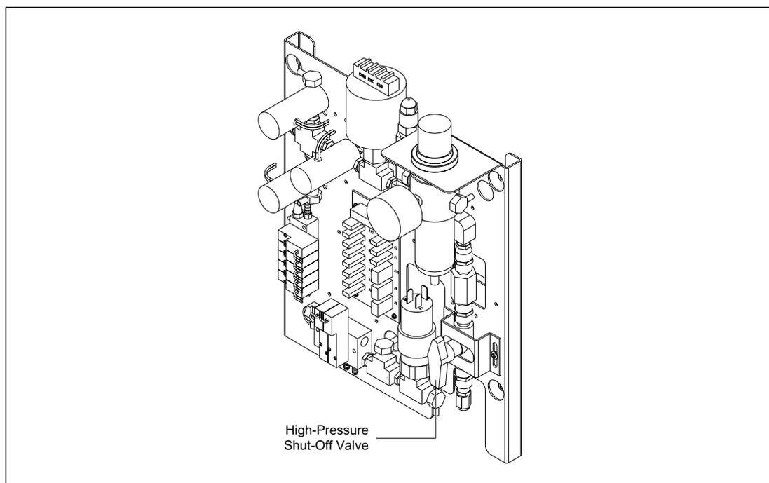
Figure 8-4. High-Pressure Shut-Off Valve.
