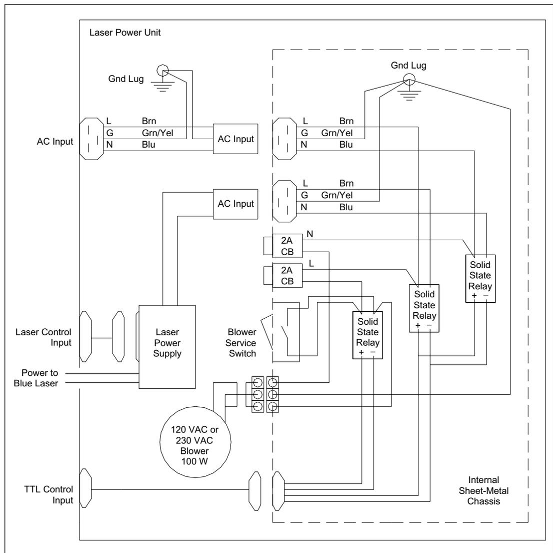
Figure 5-5. Power Supply Fan Module AC Distribution Block Diagram.
