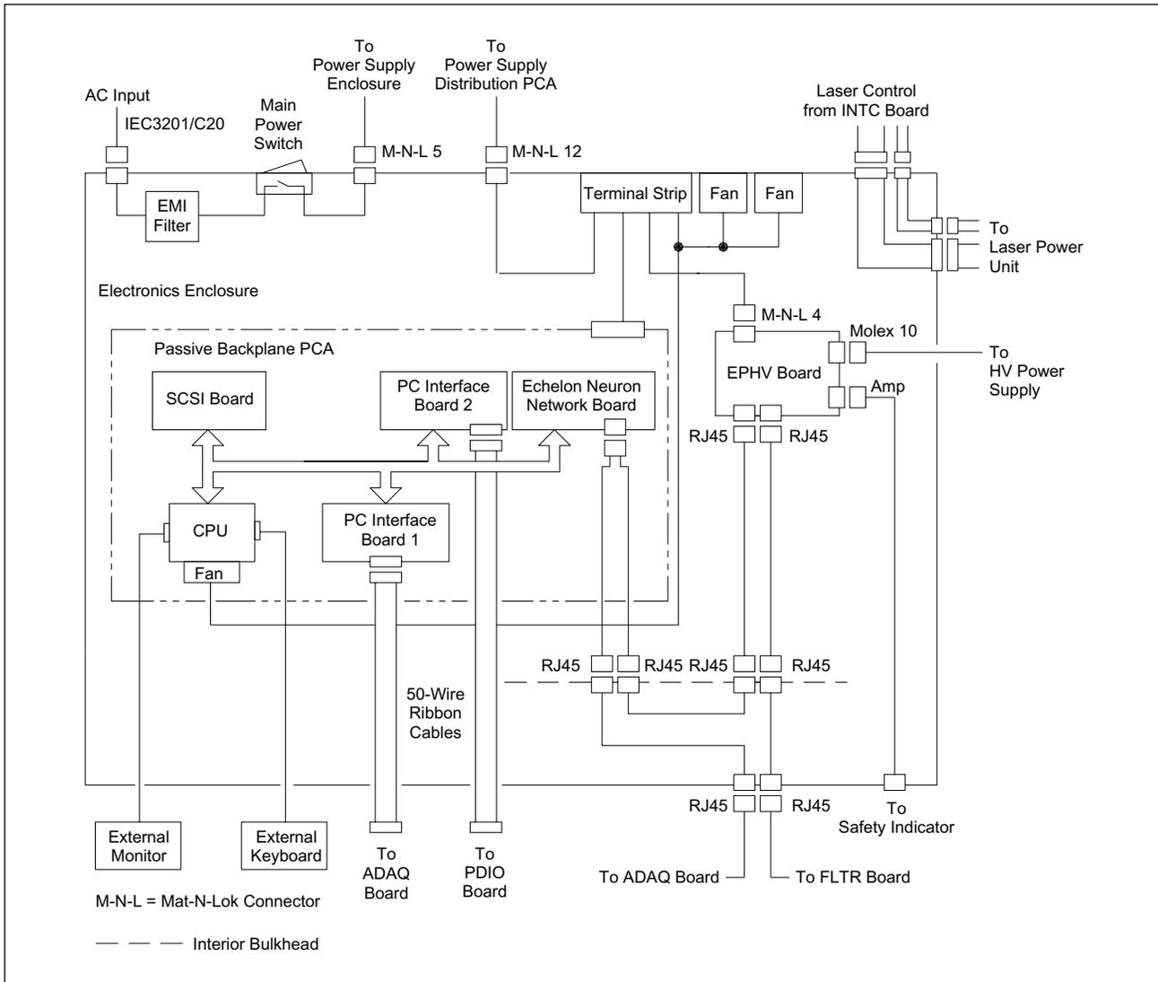
Figure 5-18. Internal Computer Block Diagram.
