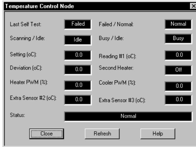
Figure 7-17. Temperature Control Node.
