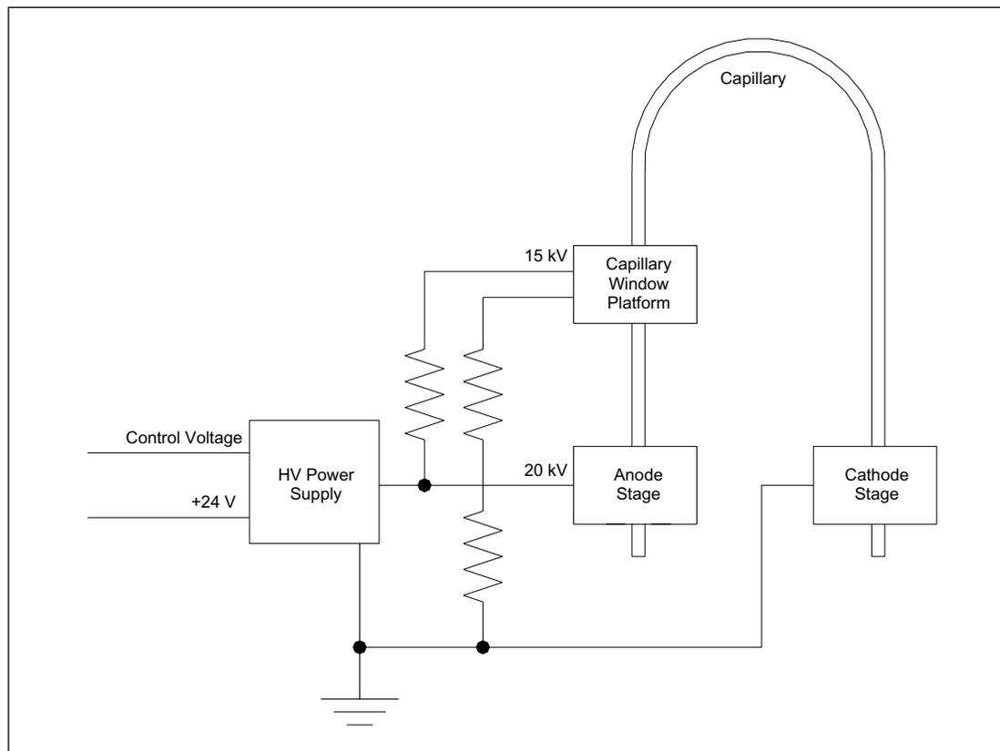
Figure 5-16. HV Power Distribution Block Diagram.
