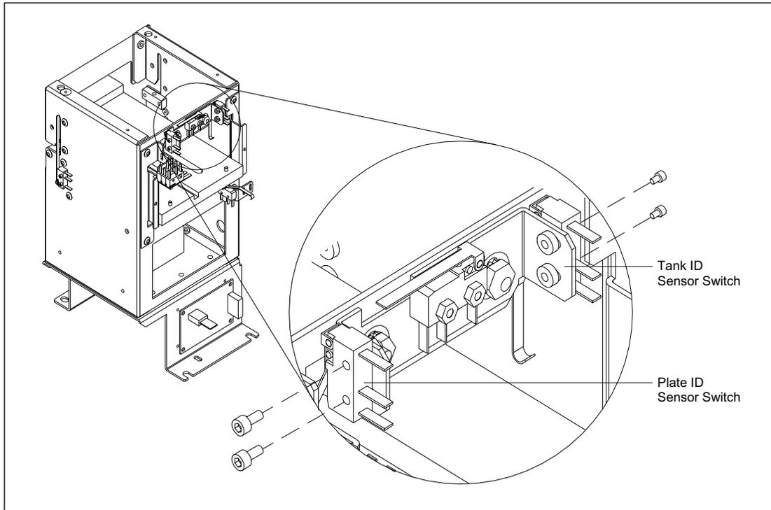
Figure 9-71. Cathode Plate and Tank ID Sensor Switches Mounting.
