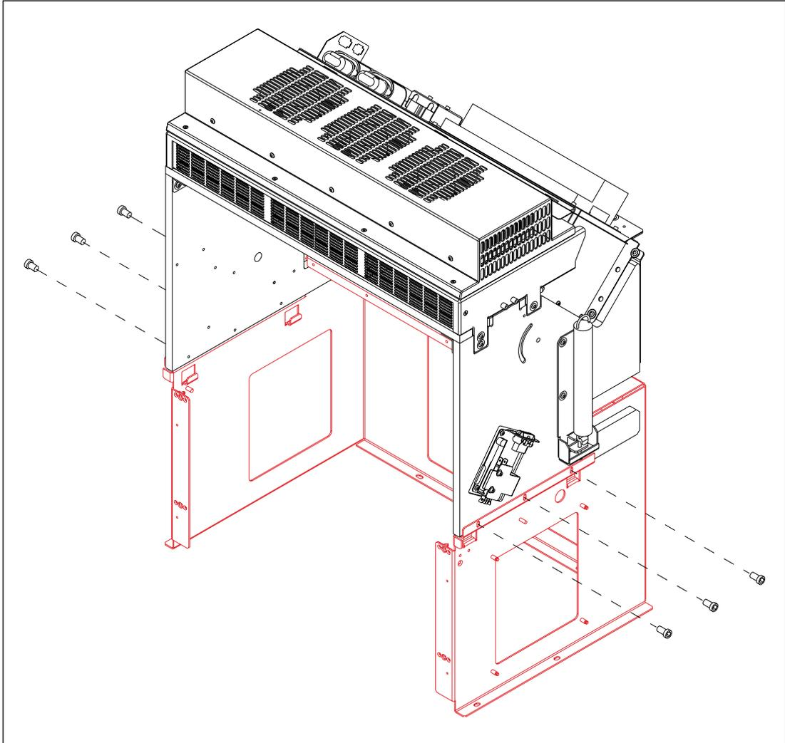
Figure 9-20. Heater/Cooler Assembly Mounting.
