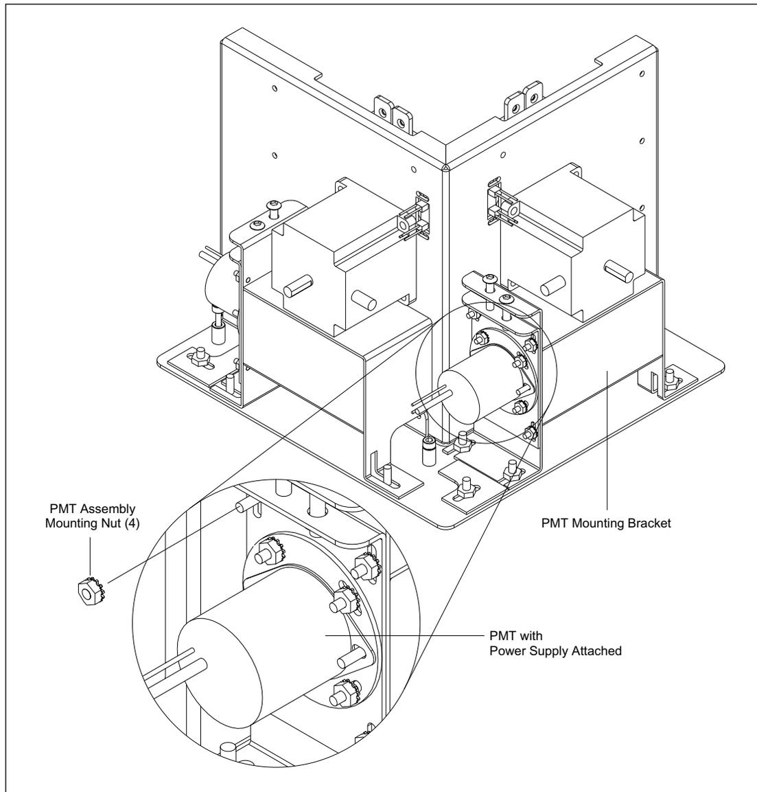
Figure 9-66. PMT Assembly Mounting.
