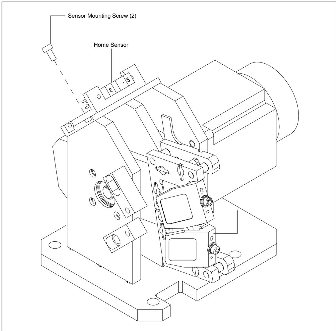
Figure 9-50. Primary Beamsplitter Changer Home Sensor Mounting.
