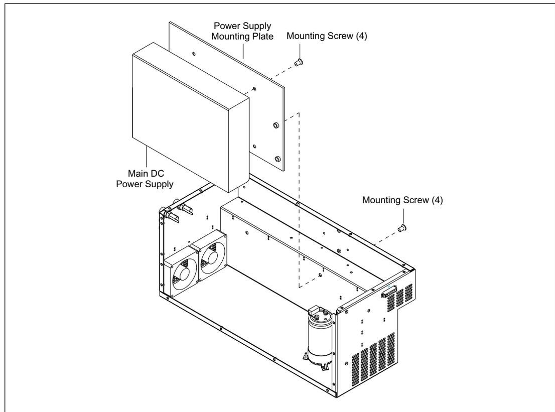
Figure 4-11. Power Supply Box Assembly.
