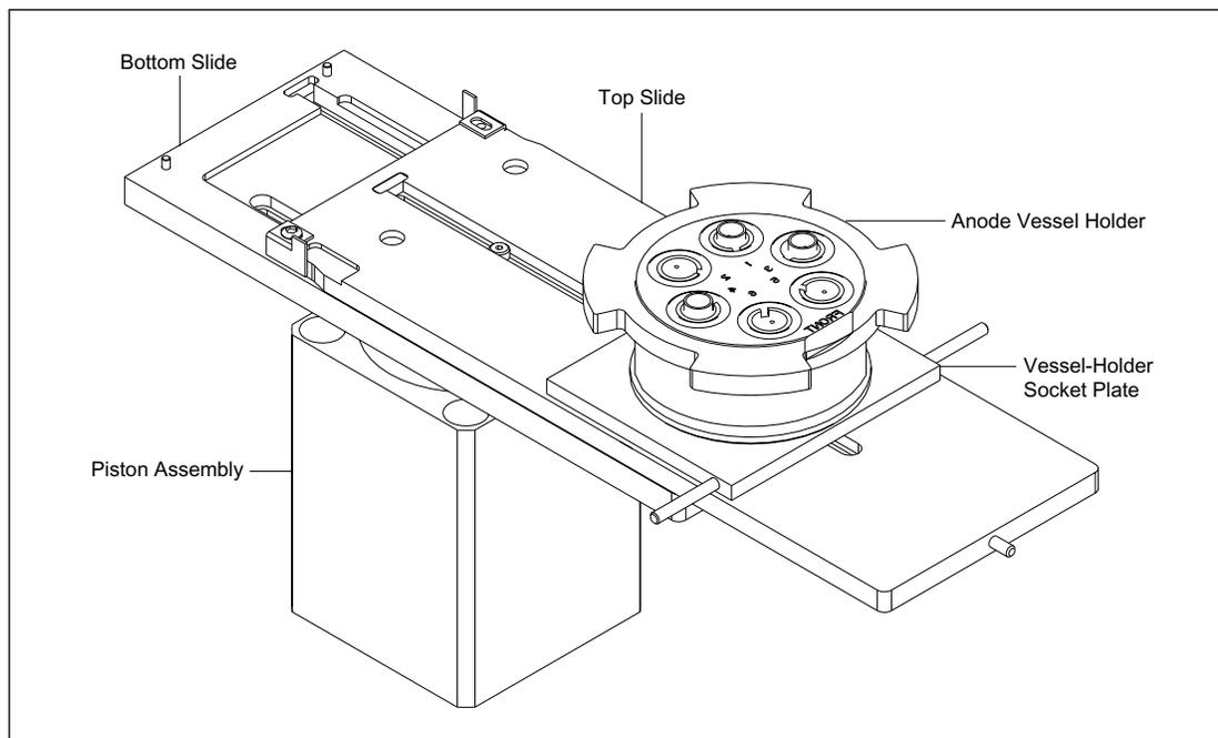
Figure 4-52. Anode Vessel and Slide Assembly.
