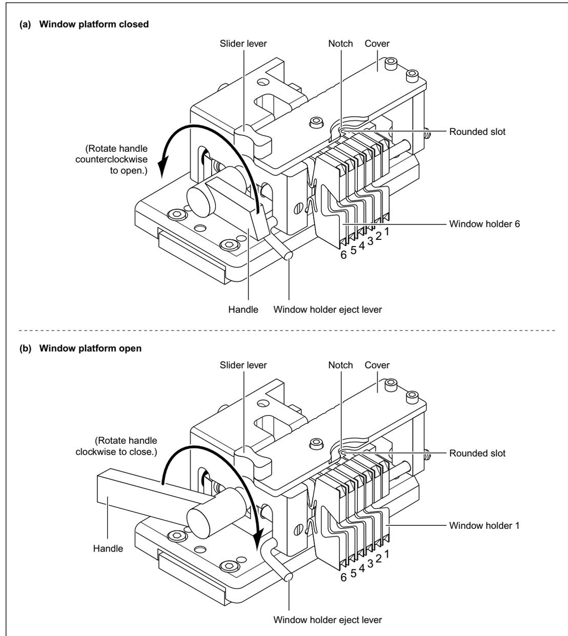
Figure 3-6. Capillary Window Platform.
