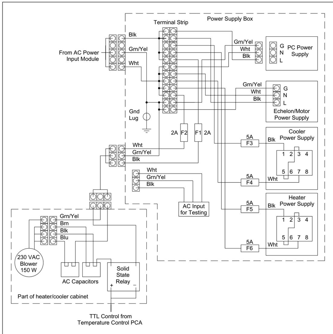
Figure 5-2. Main AC Distribution Block Diagram (Four-Supply Model).
