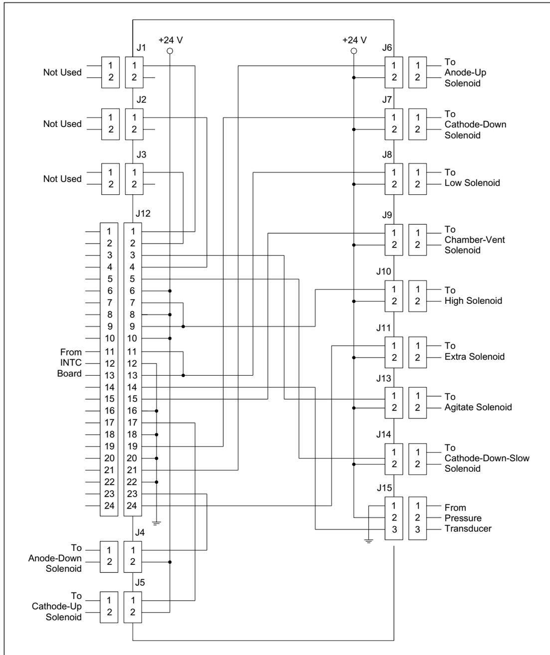
Figure 5-65. Pressure Connector Board Connector Detail Diagram.
