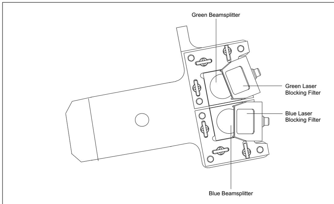
Figure 3-17. Beamsplitter Arm Assembly.
