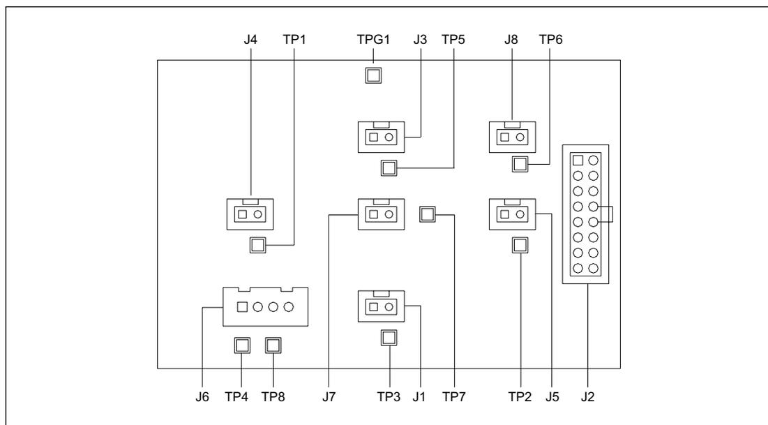
Figure 5-57. Cathode Connector Board Component Layout Diagram.
