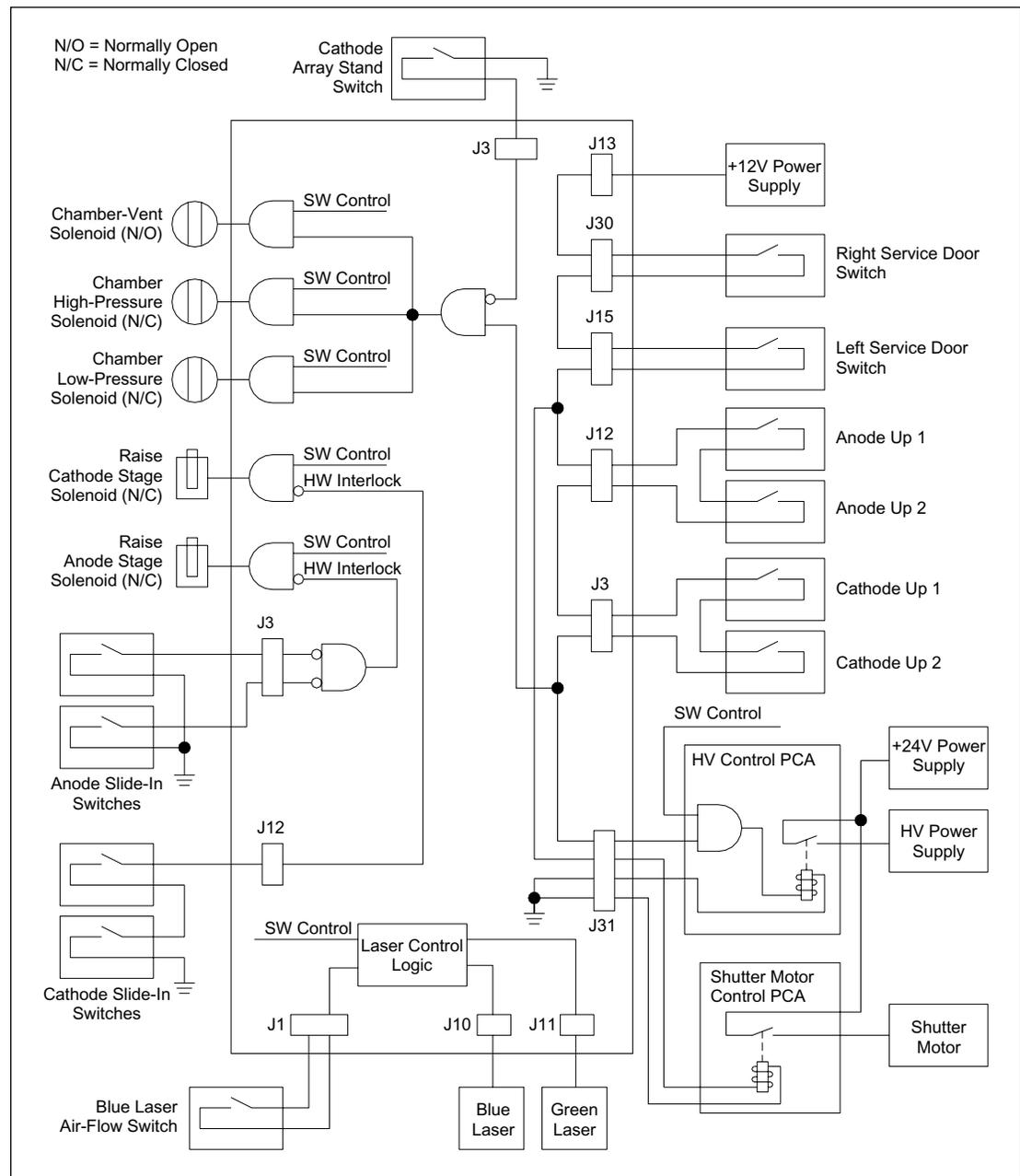
Figure 5-66. Safety Interlock System Block Diagram.
