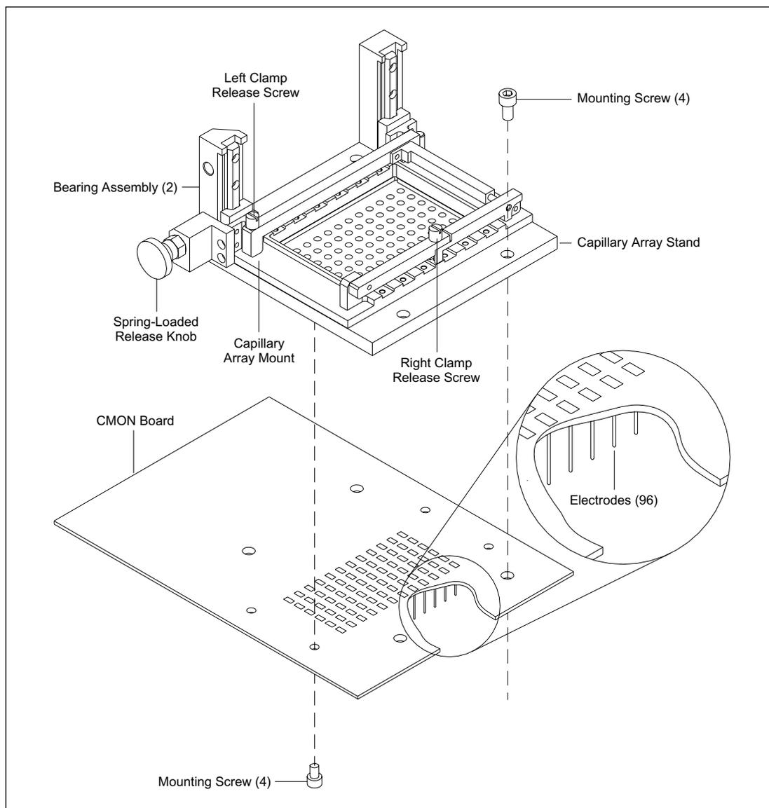
Figure 4-43. Cathode Array Stand Assembly.
