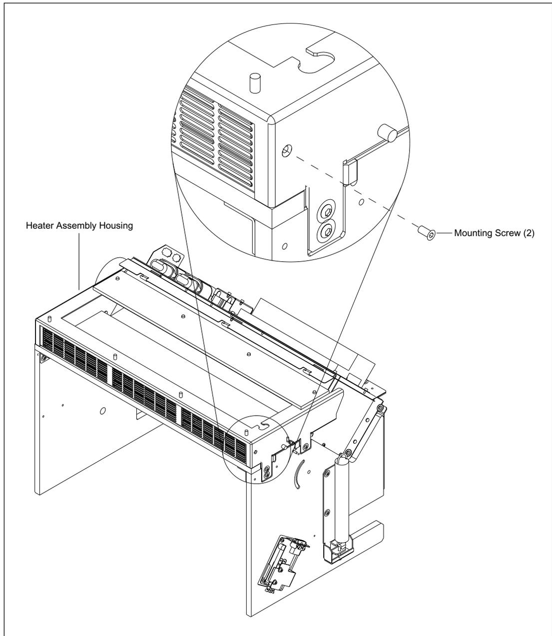
Figure 9-24. Heater Assembly Mounting.
