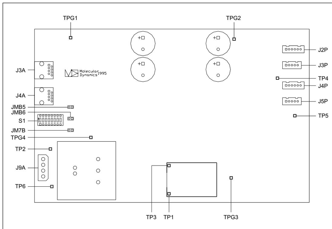
Figure 5-29. FLTR Board Component Layout Diagram.
