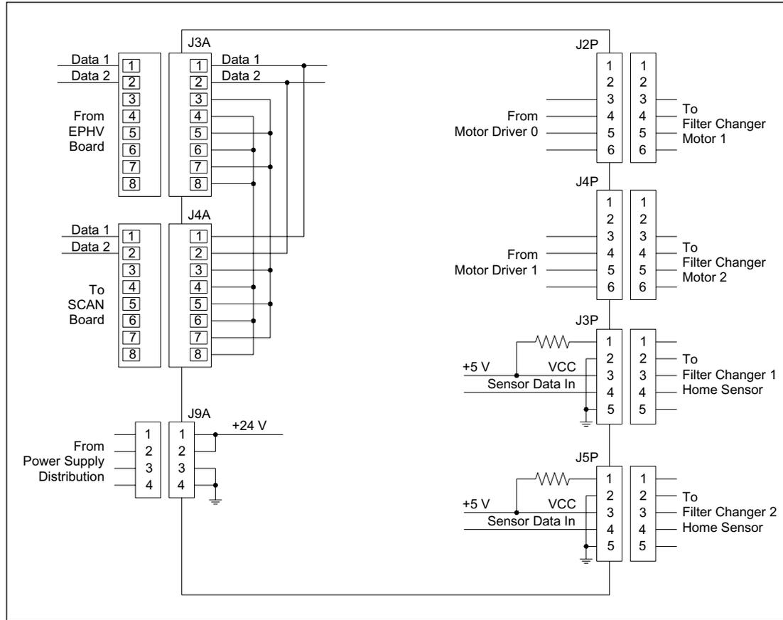
Figure 5-30. FLTR Board Connector Detail Diagram.
