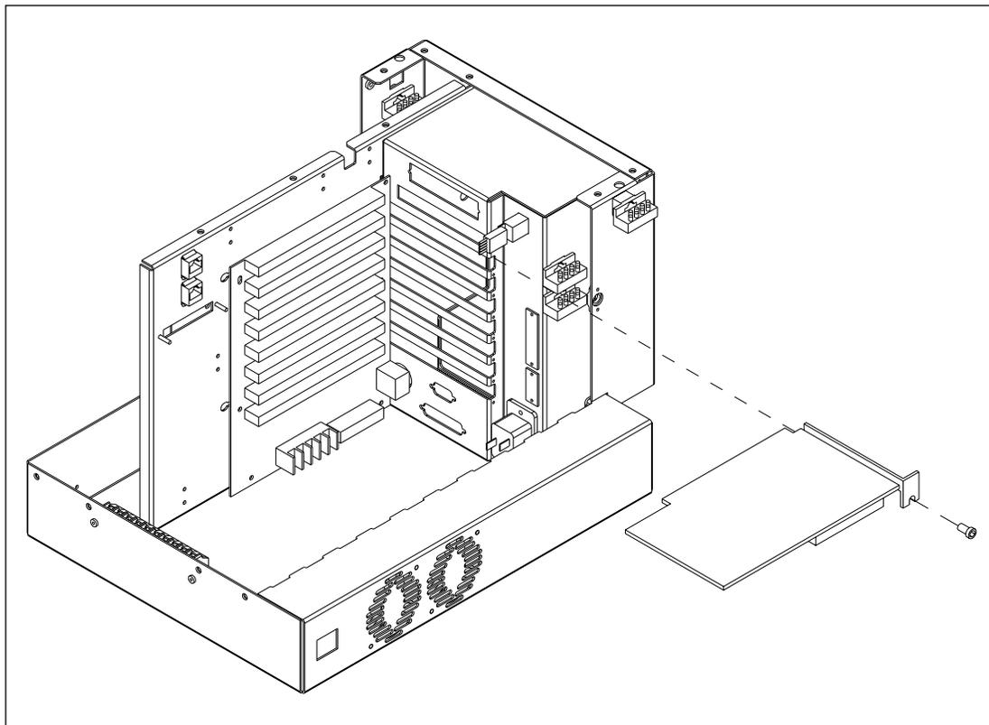
Figure 9-31. Host SCSI Interface Board Mounting.
