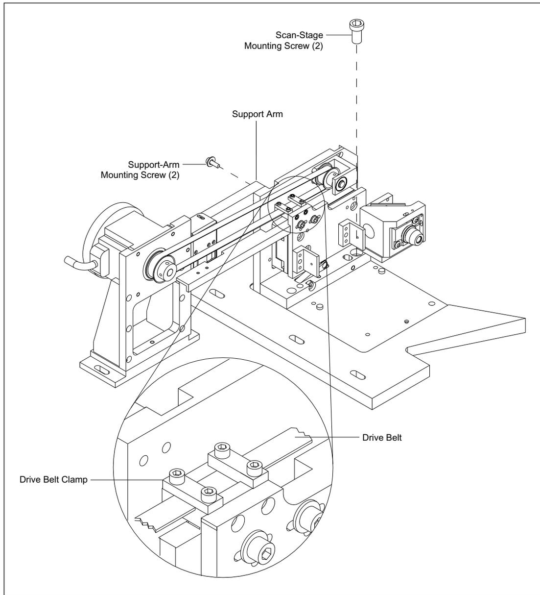
Figure 9-51. Scanning Stage Assembly Mounting.
