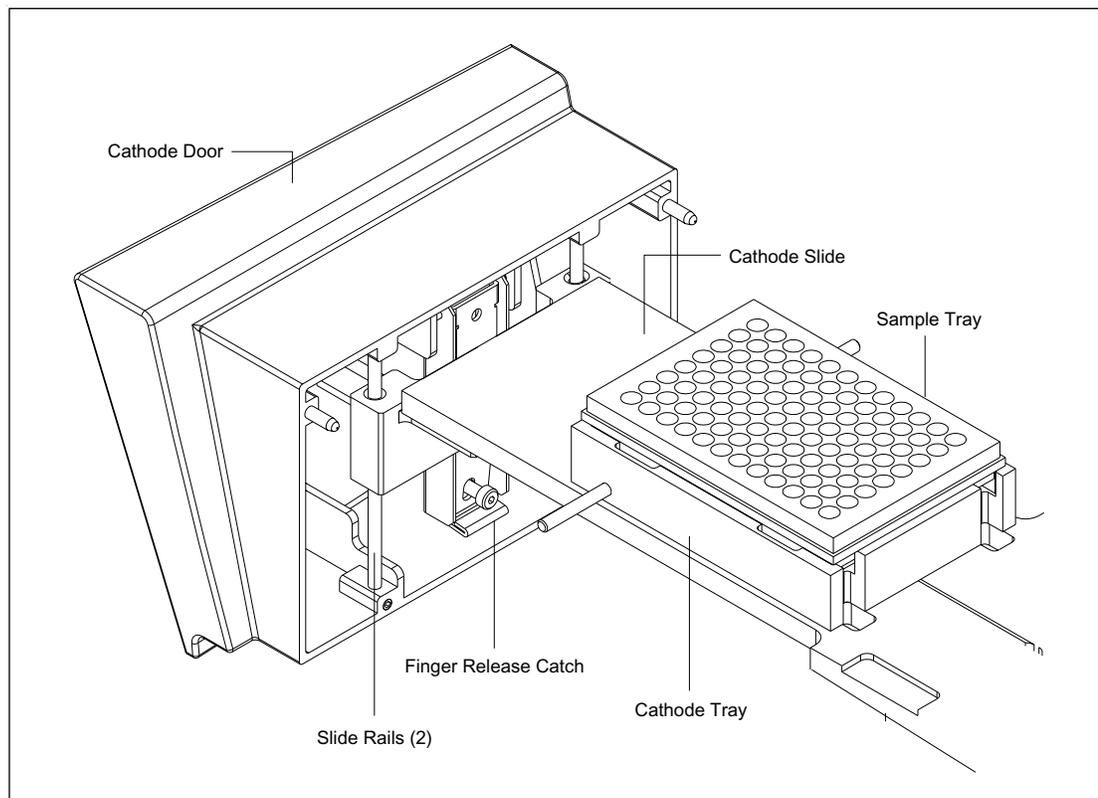
Figure 4-8. Cathode Door Assembly.
