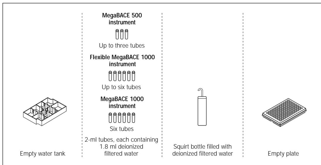
Figure 6-24. The Materials for the Prepare Capillaries Protocol. **Note:** You use one tube of water for each capillary array installed in the instrument.
