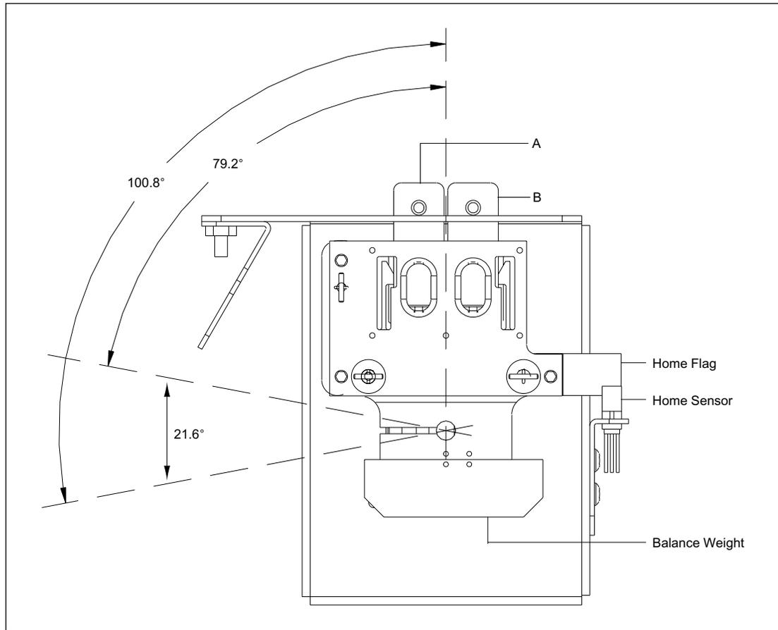
Figure 4-36. Secondary Beamsplitter Arm Assembly.
