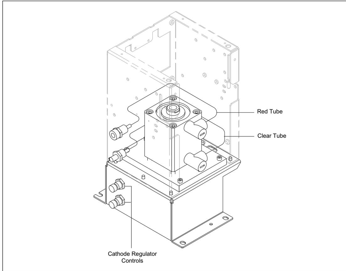
Figure 8-19. Converted Cathode.
