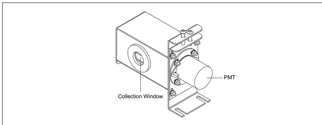
Figure 3-24. PMT Assembly.
