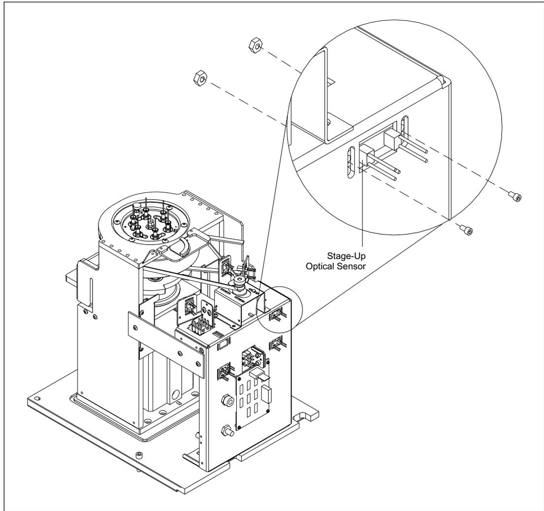
Figure 9-91. Anode Stage-Up Optical Sensor Mounting.
