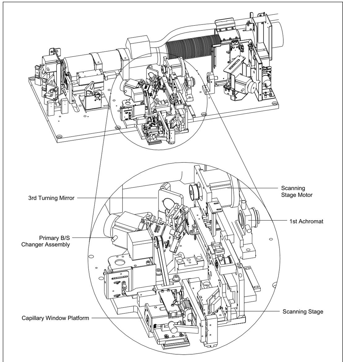
Figure 4-17. Optical Components Assembly (Sheet 2 of 3).
