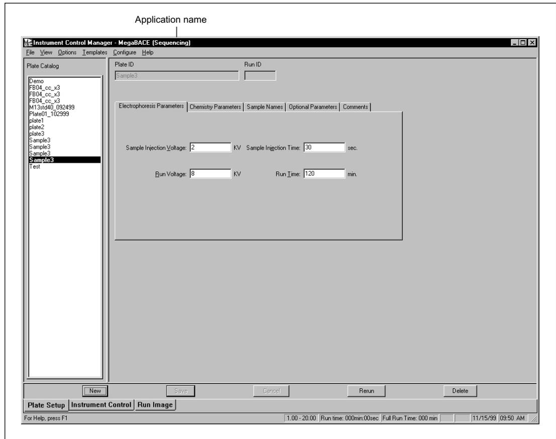
Figure 6-20. The Plate Setup window. The name of the selected application appears in the title bar of each of the Instrument Control Manager windows.
