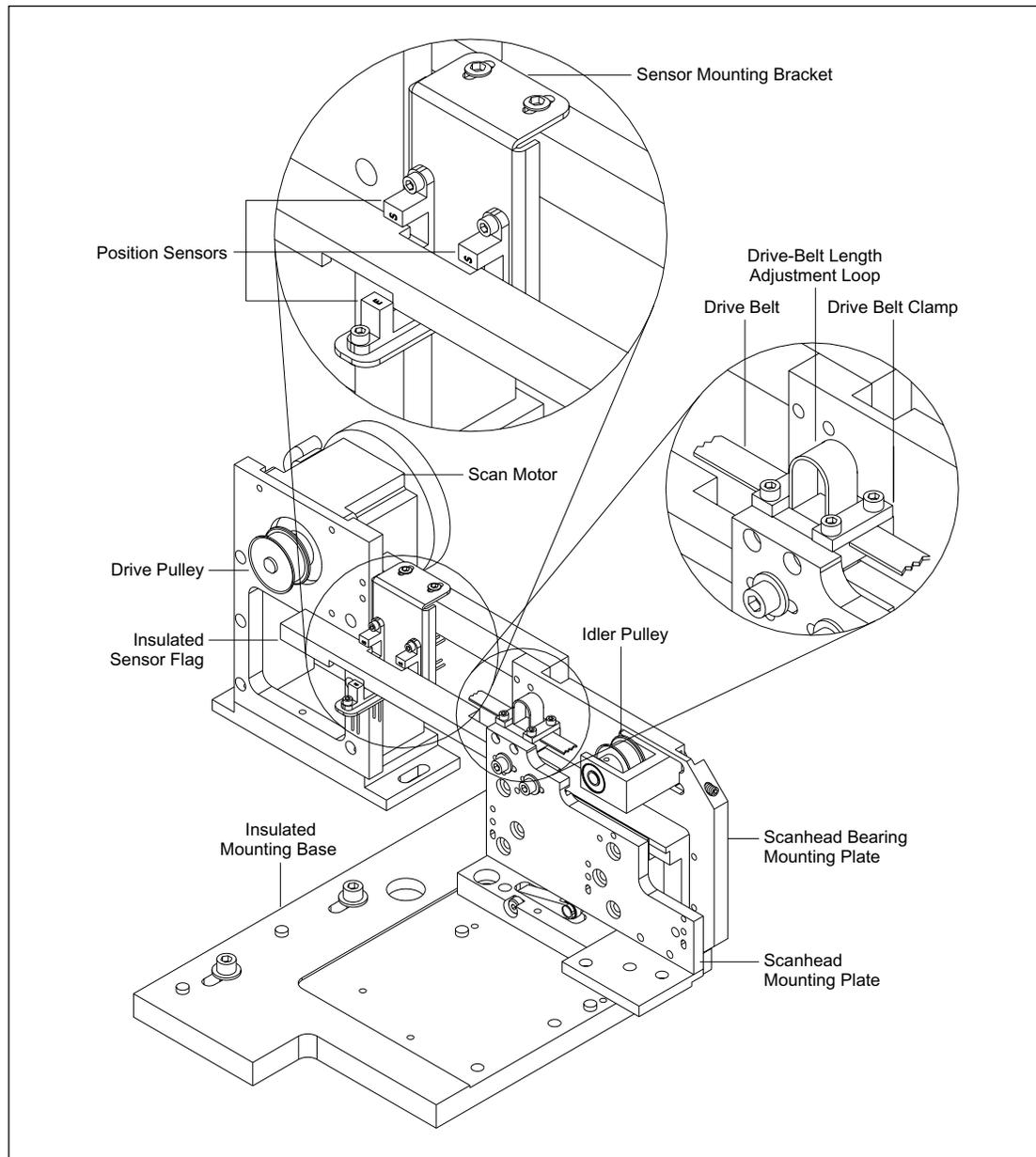
Figure 4-31. Scanhead Drive Assembly.
