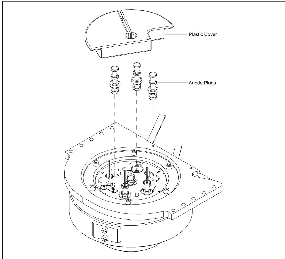
Figure 3-9. Anode Cover (MB 500).
