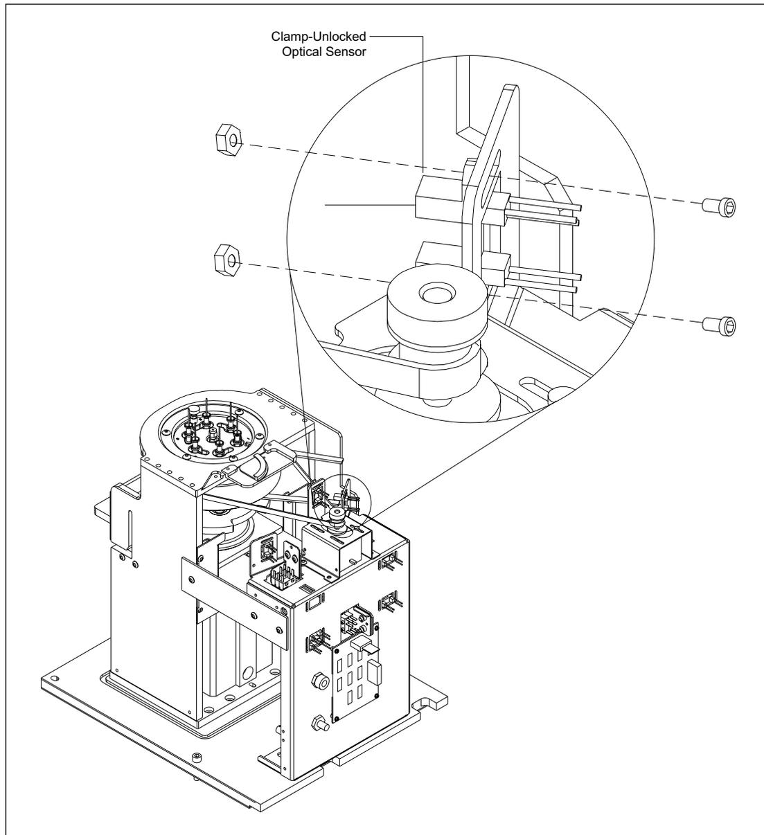
Figure 9-87. Anode Cover Clamp-Unlocked Optical Sensor Mounting.
