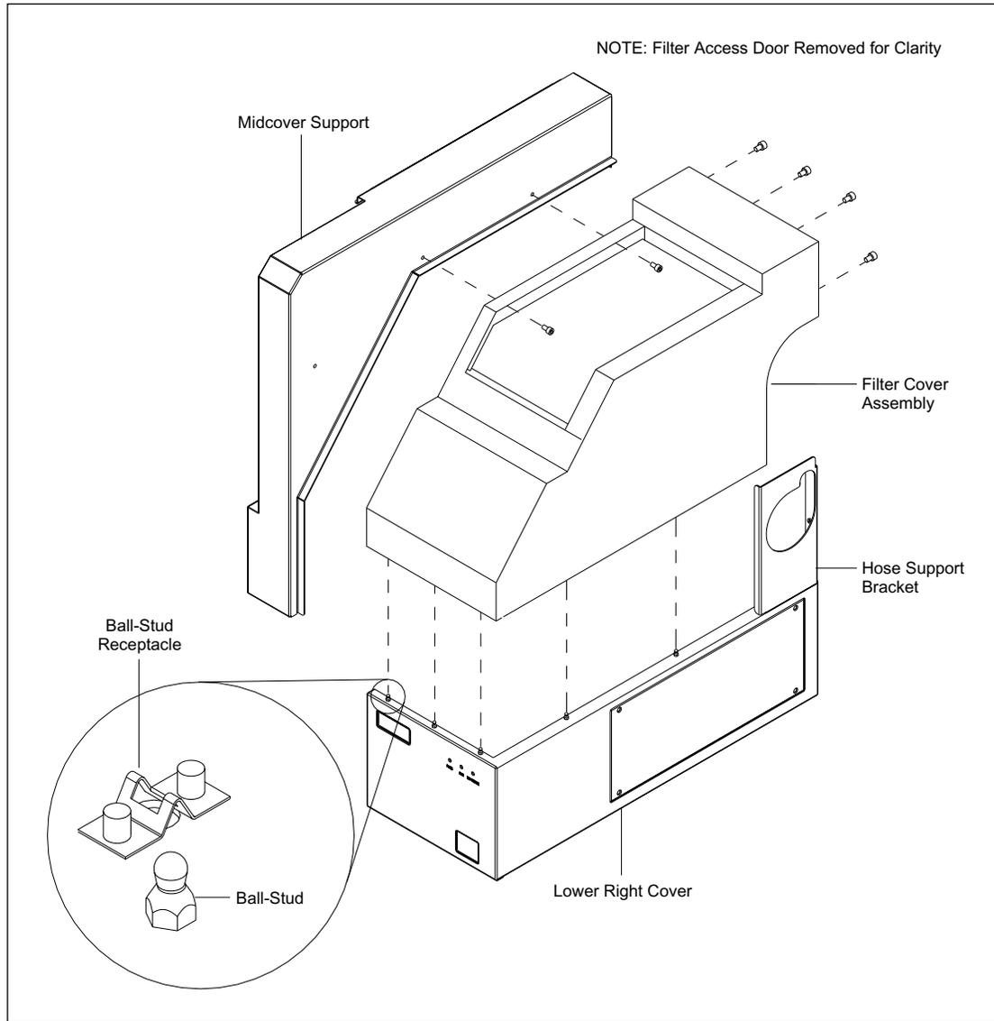
Figure 9-3. Filter Cover Assembly Mounting.
