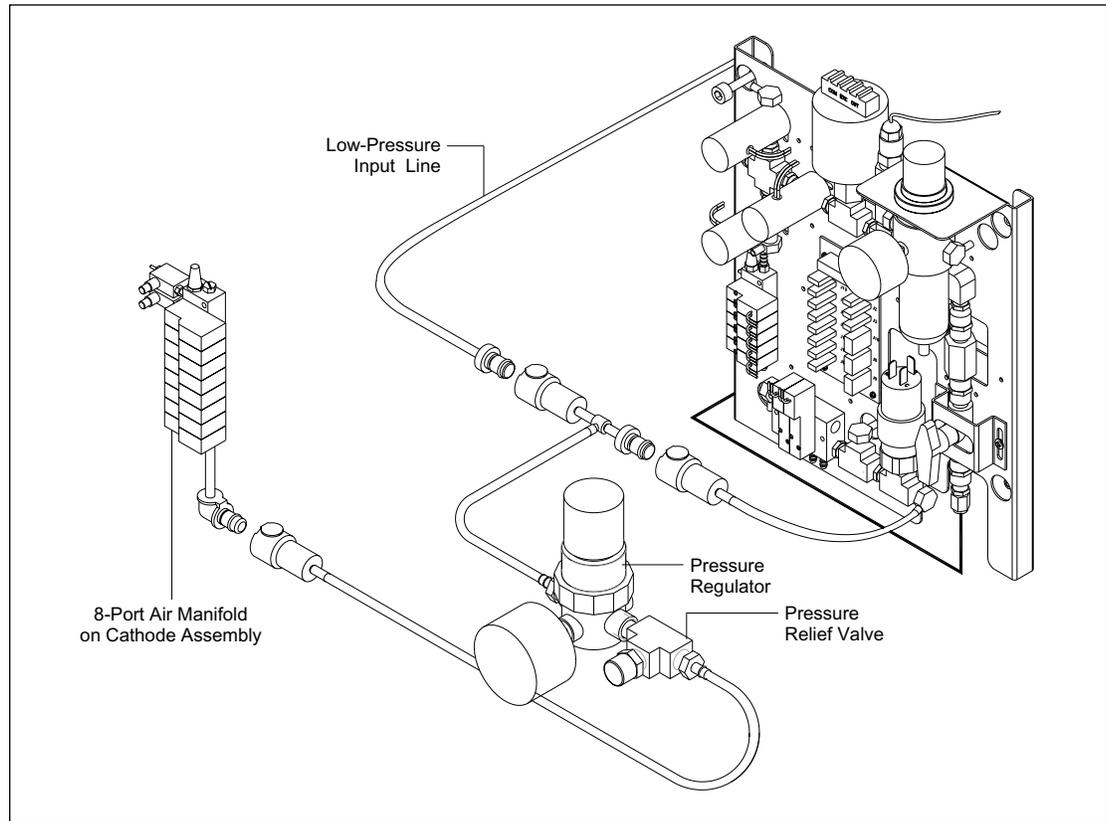
Figure 8-10. New Cathode Pneumatics.
