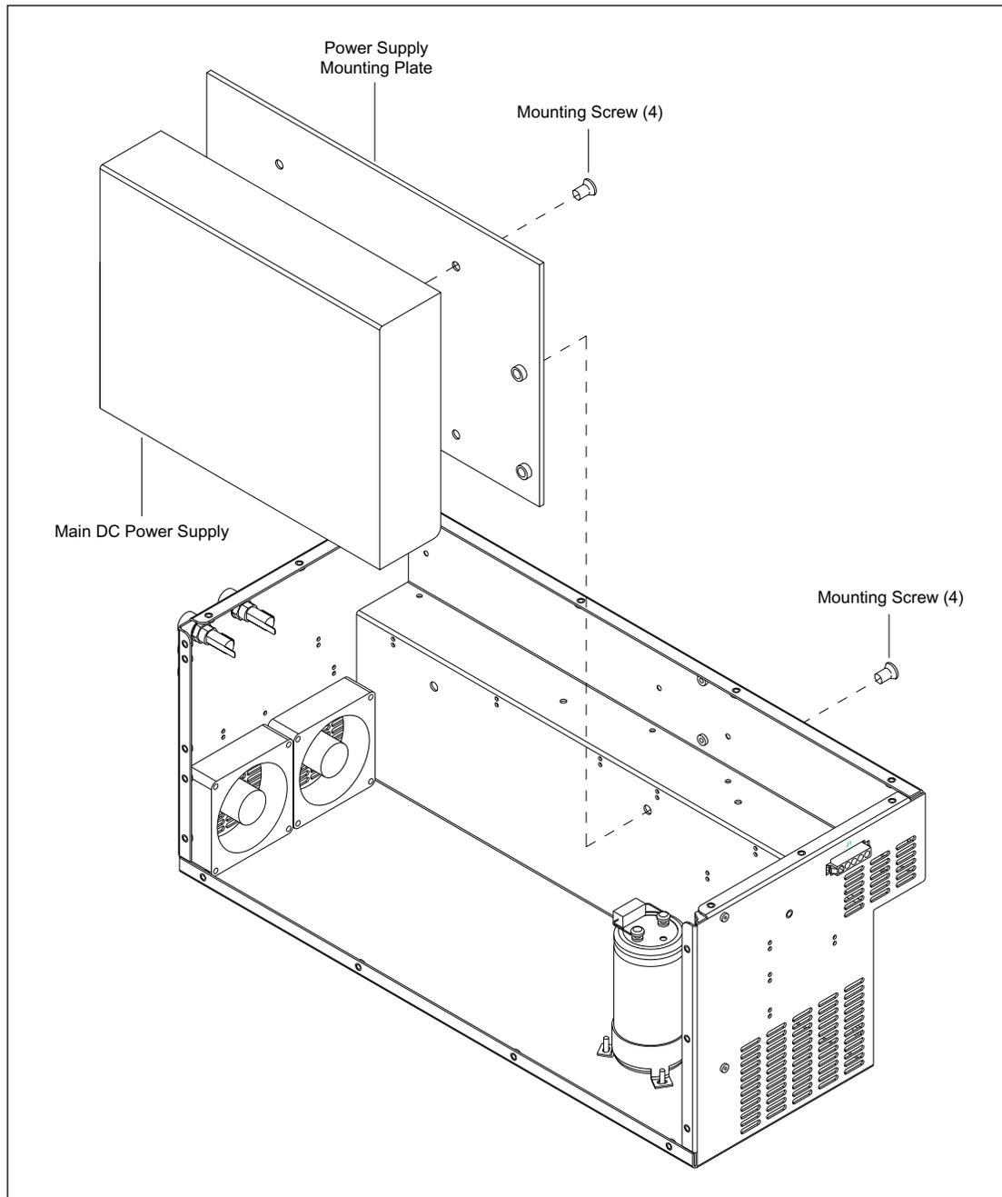
Figure 9-19. Main DC Power Supply Mounting (CE 2001).
