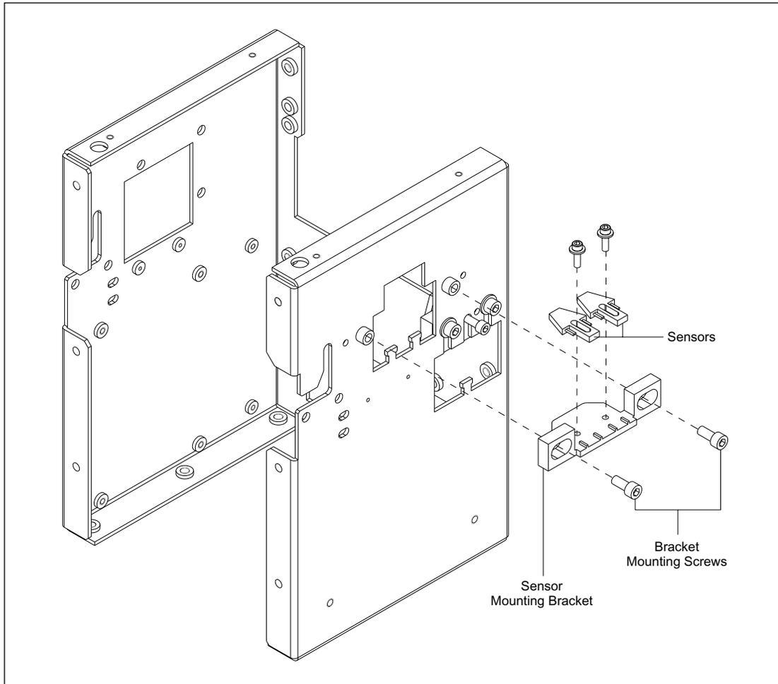
Figure 9-75. Indexer Y-Position Sensor Mounting (MB 2000).
