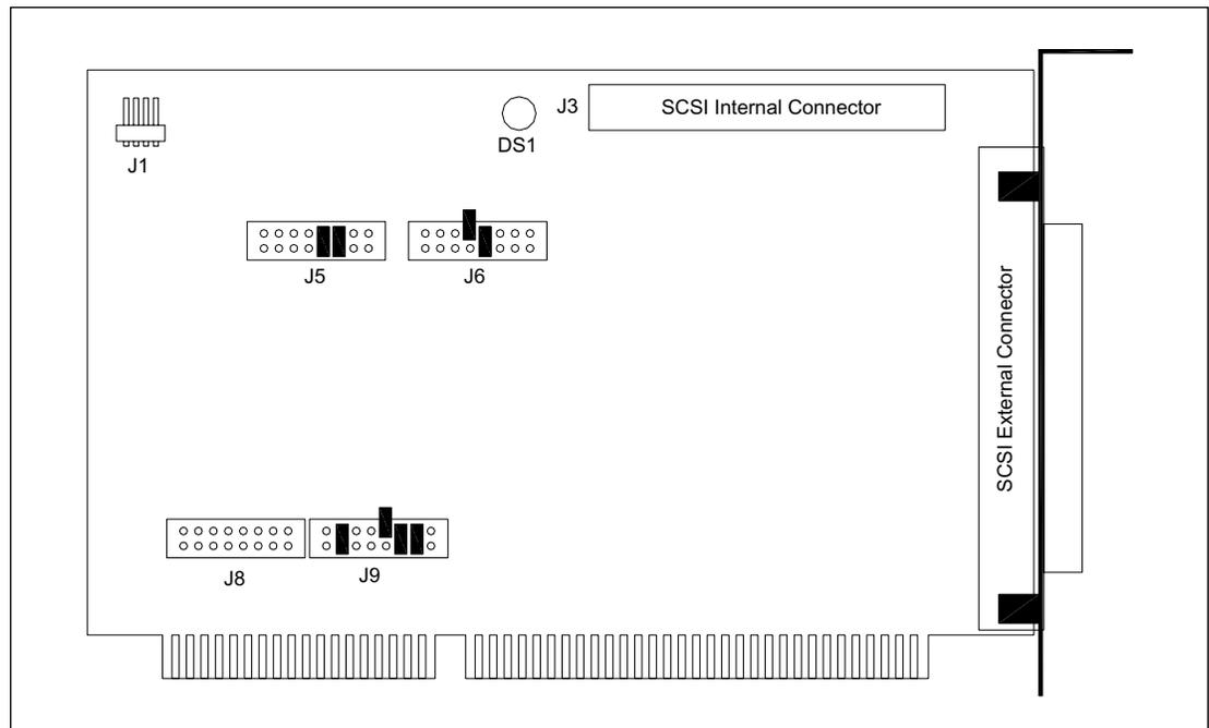
Figure 5-19. SCSI Interface Board Component Layout Diagram.
