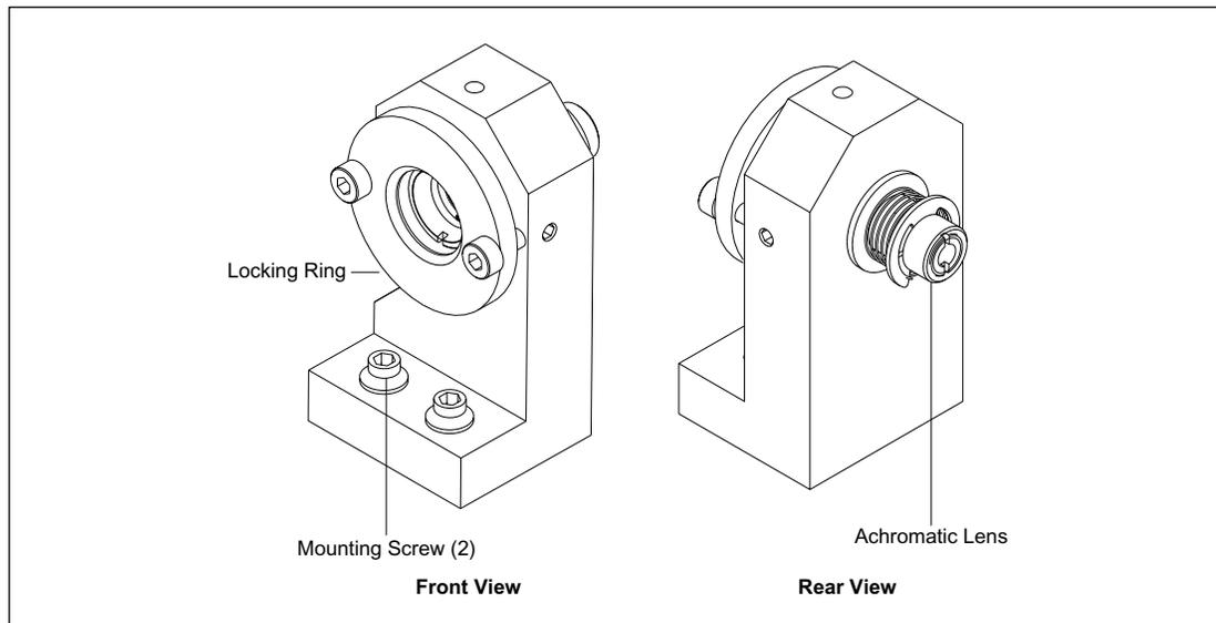
Figure 4-34. Pinhole and Second Achromatic Lens.
