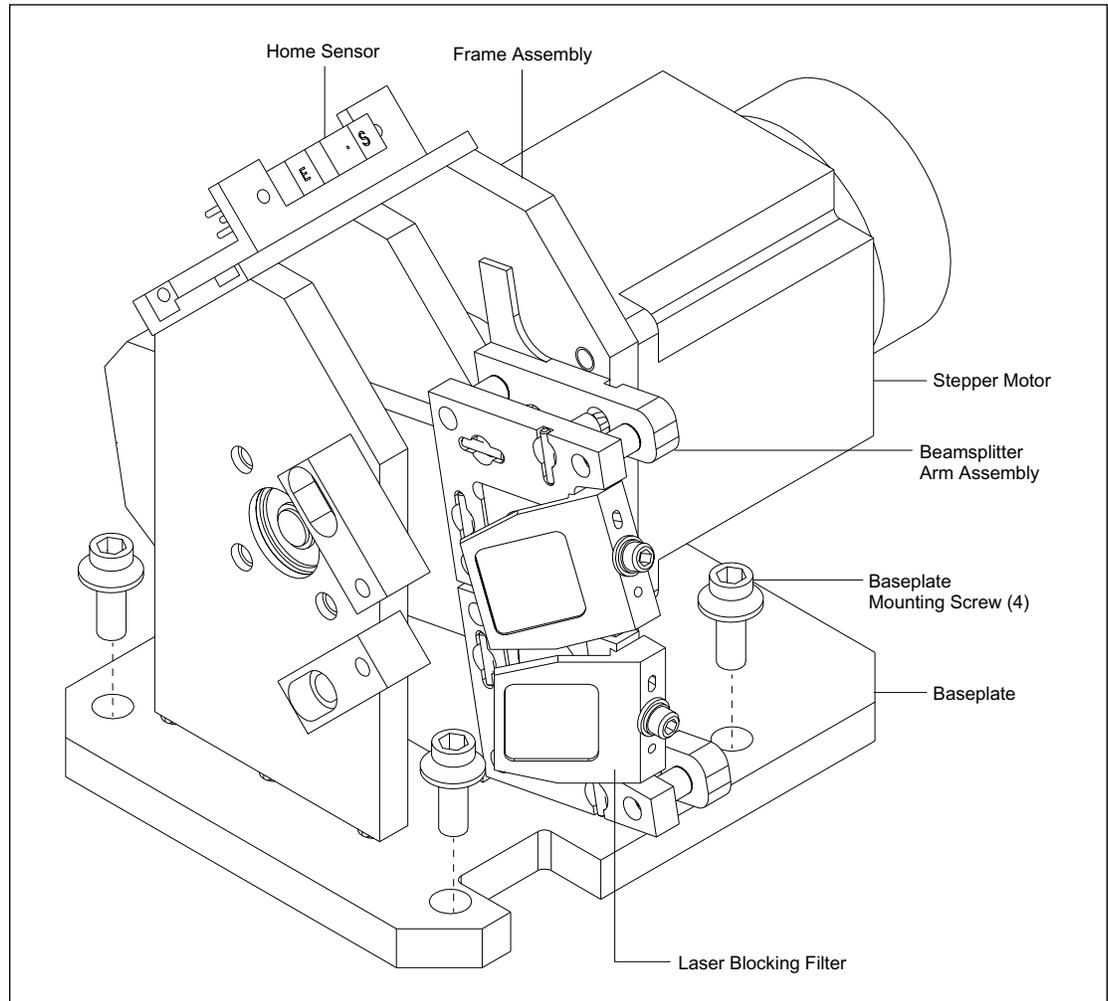
Figure 4-27. Primary Beamsplitter Changer Assembly.
