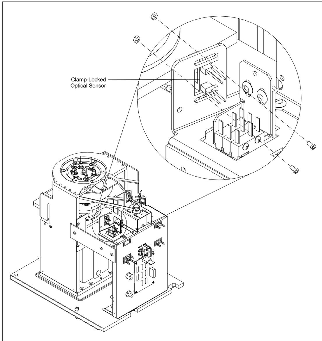
Figure 9-86. Anode Cover Clamp-Locked Optical Sensor Mounting.
