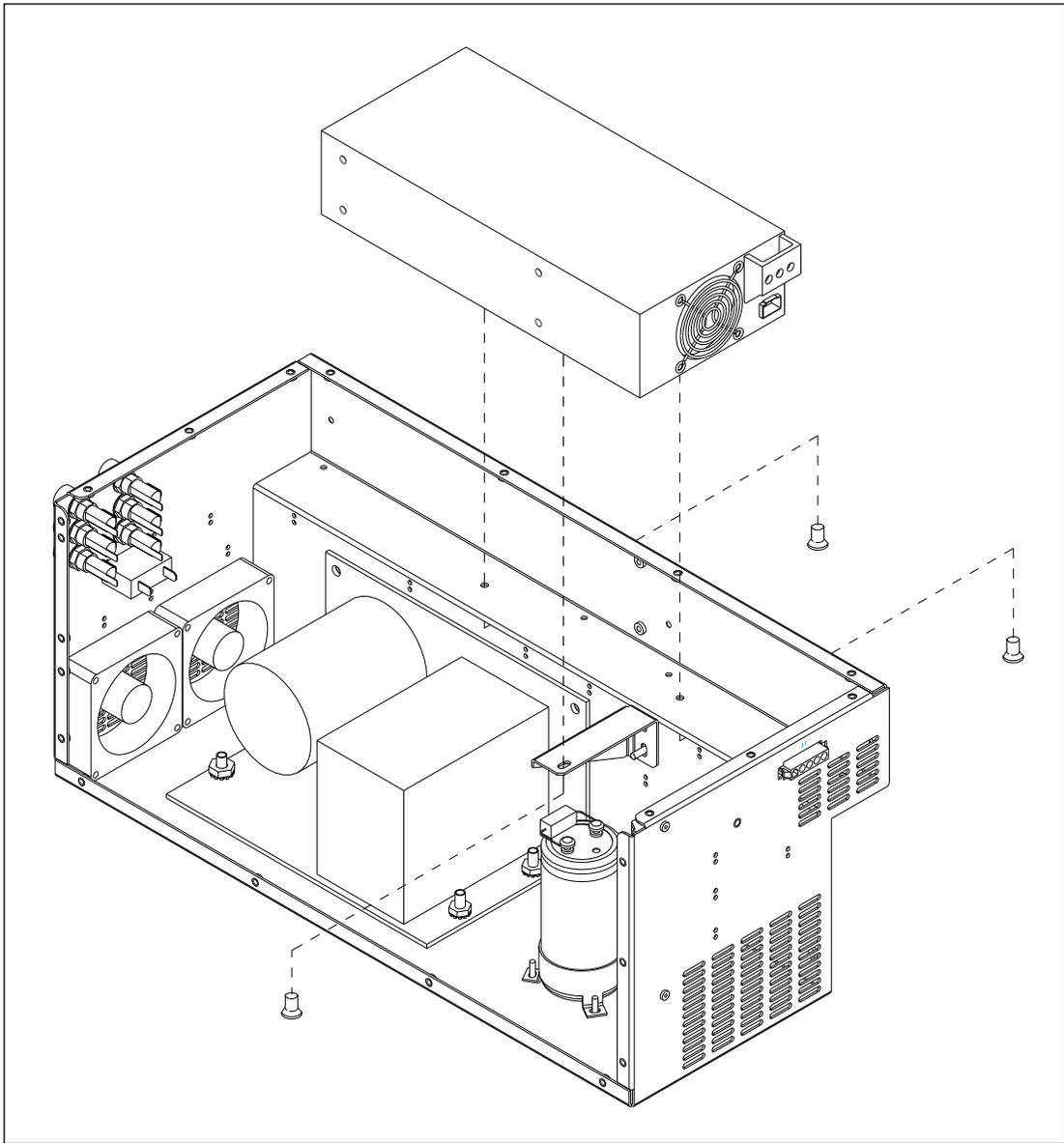
Figure 9-17. Main DC Power Supply Mounting (Two-Supply Model).
