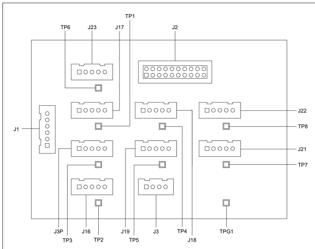
Figure 5-62. Anode Connector Board Component Layout Diagram.
