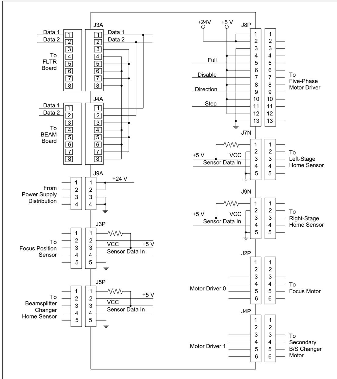
Figure 5-33. SCAN Board Connector Detail Diagram.
