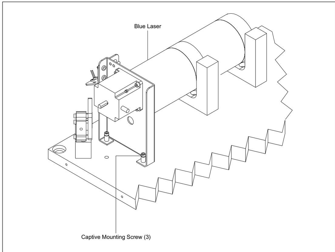
Figure 9-45. Shutter Assembly Mounting.
