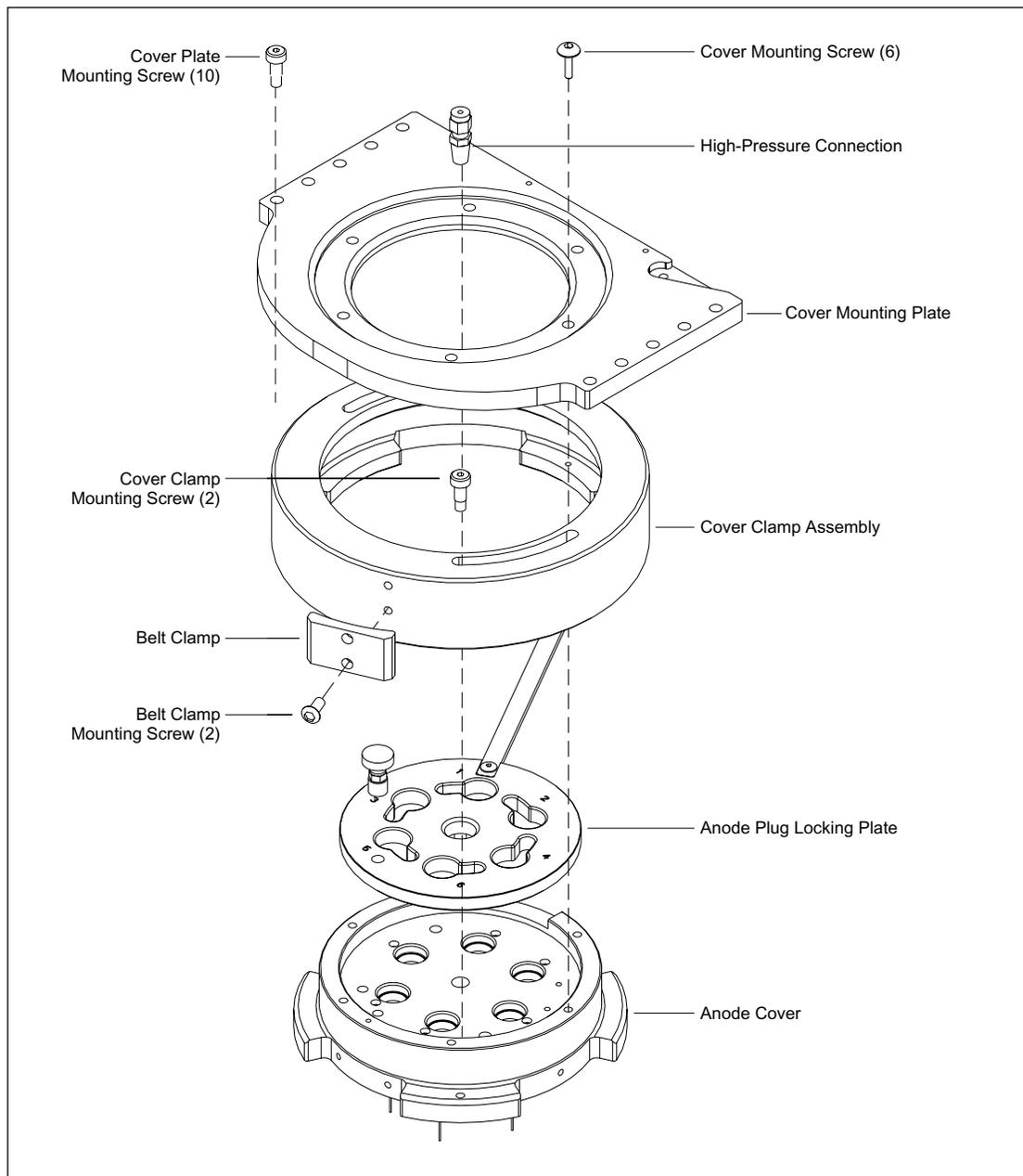
Figure 9-82. Anode Cover Mounting.
