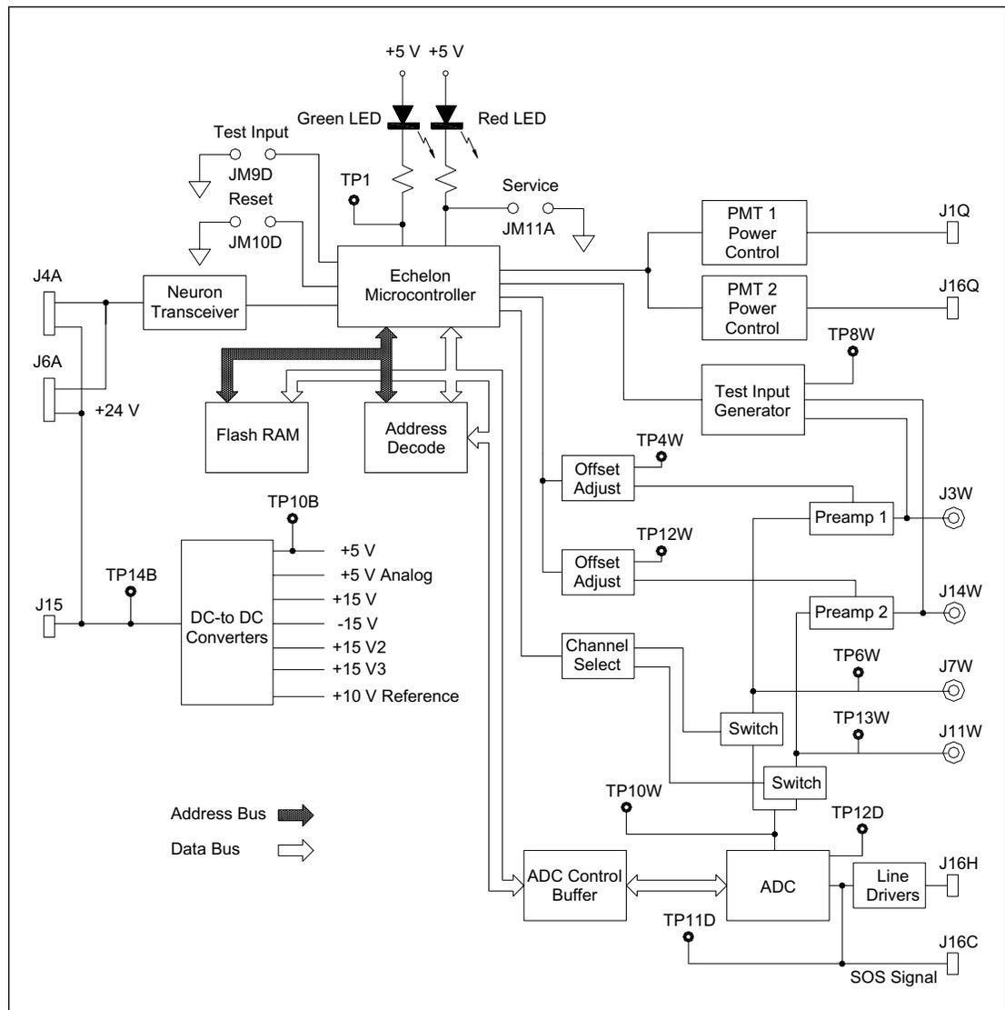
Figure 5-51. ADAQ Board Block Diagram.
