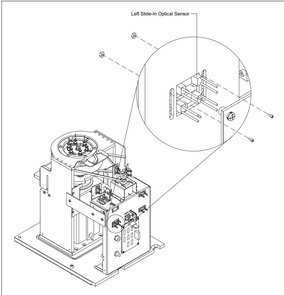
Figure 9-83. Anode Left Slide-In Sensor Mounting.
