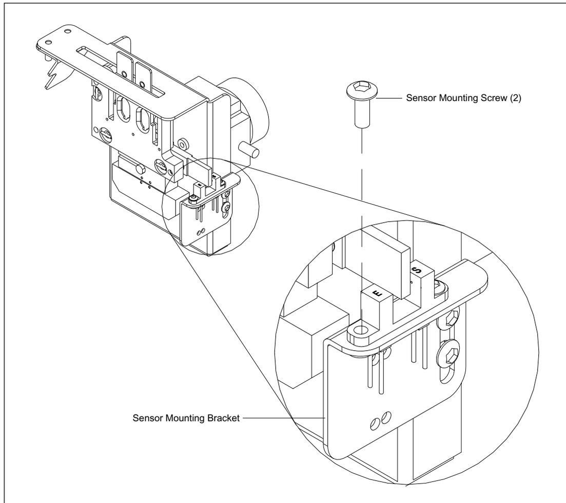
Figure 9-62. Secondary Beamsplitter Changer Home Sensor Mounting.
