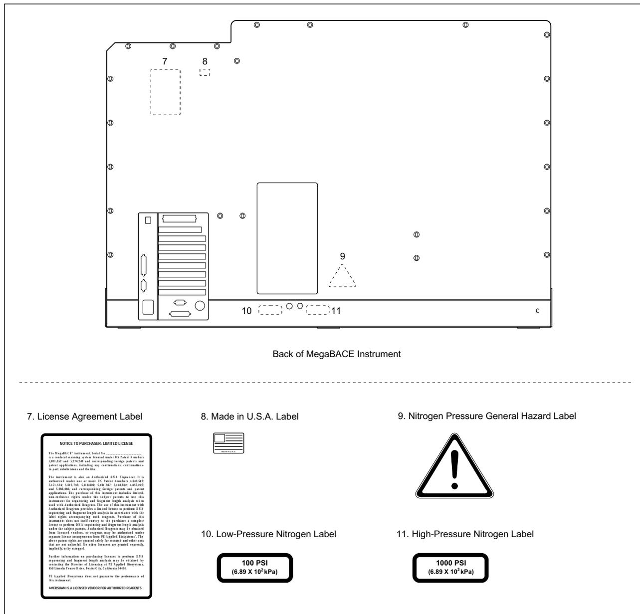
Figure 6-13. Locations of Important Labels on the Instrument (Back View).
