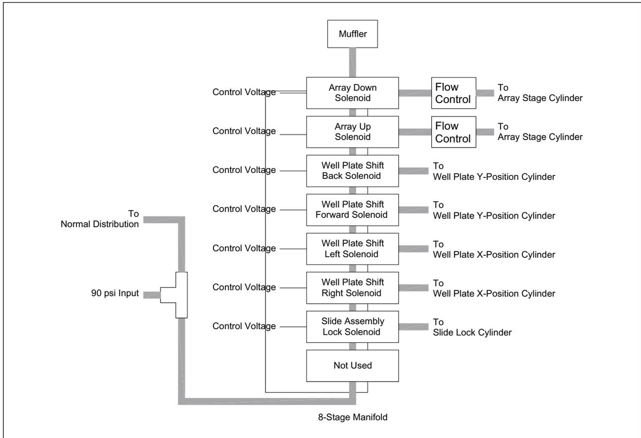
Figure 2-7. MB 2000 Cathode Pneumatics, Simplified Block Diagram.
