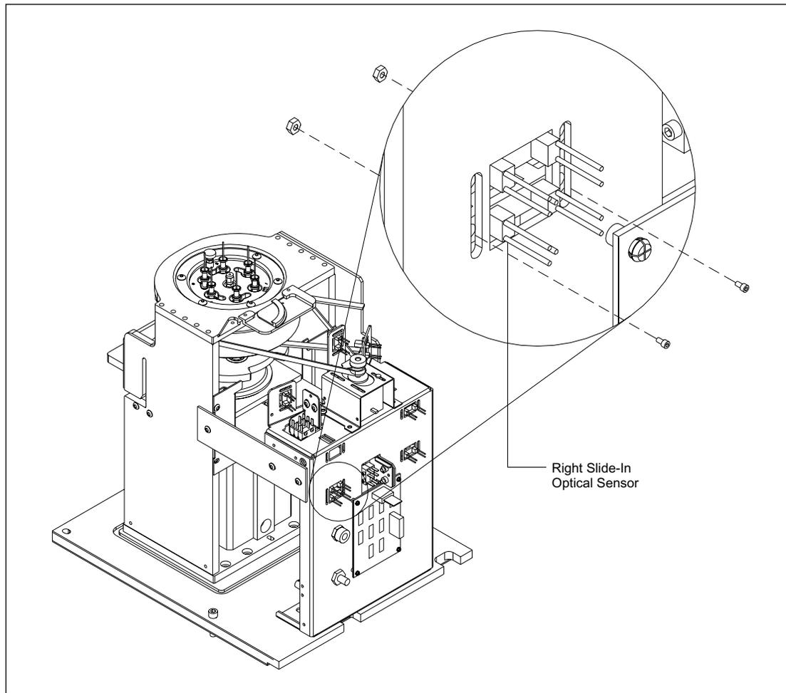
Figure 9-84. Anode Right Slide-In Optical Sensor Mounting.
