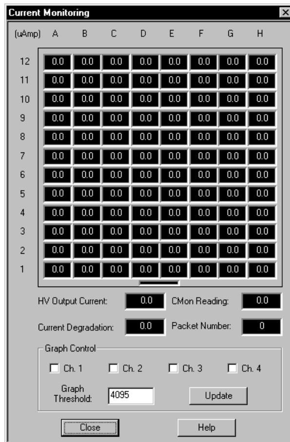
Figure 7-3. Current Monitor and Graph Control Screen.
