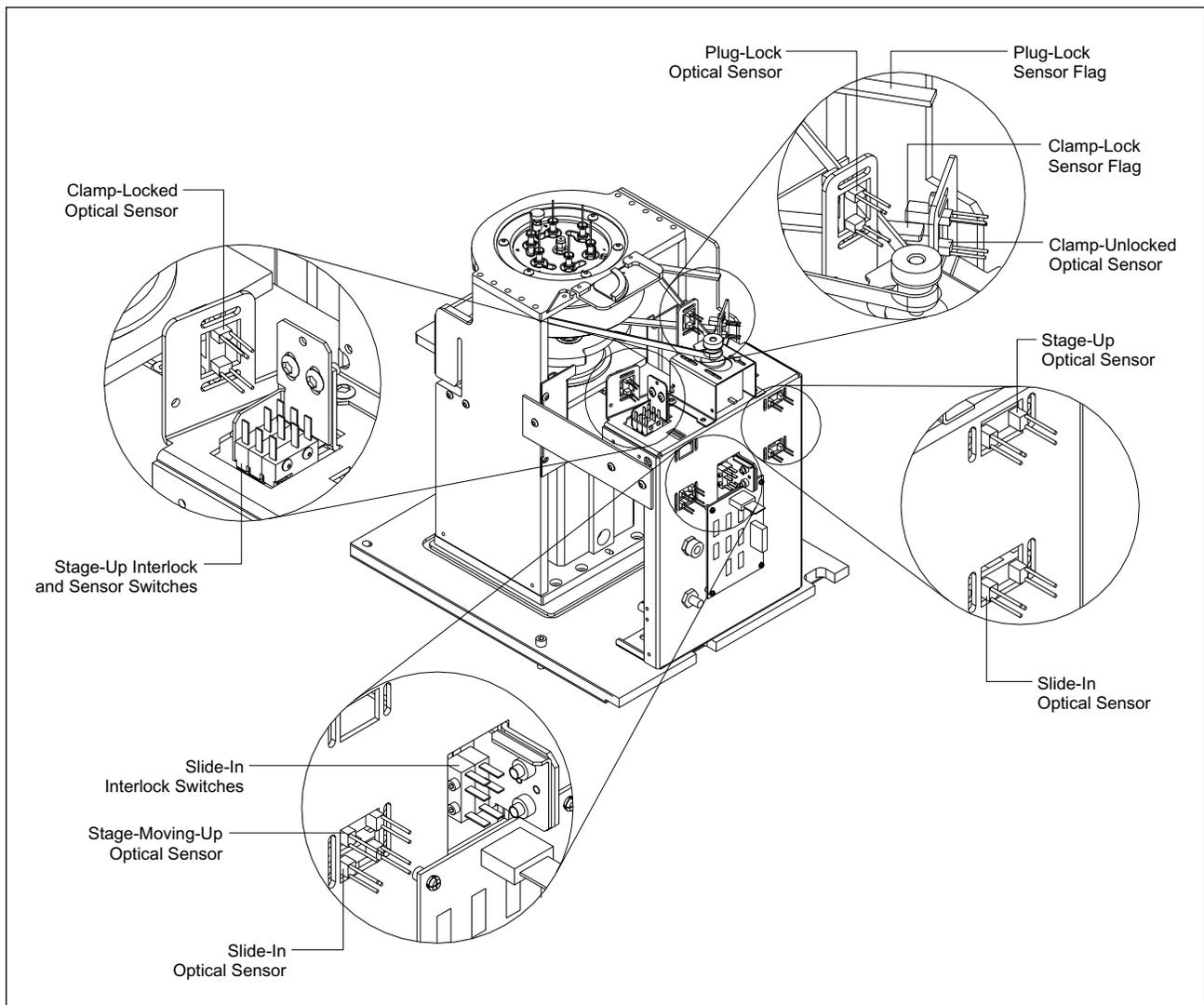
Figure 4-53. Anode Assembly, Switch and Sensor Locations.
