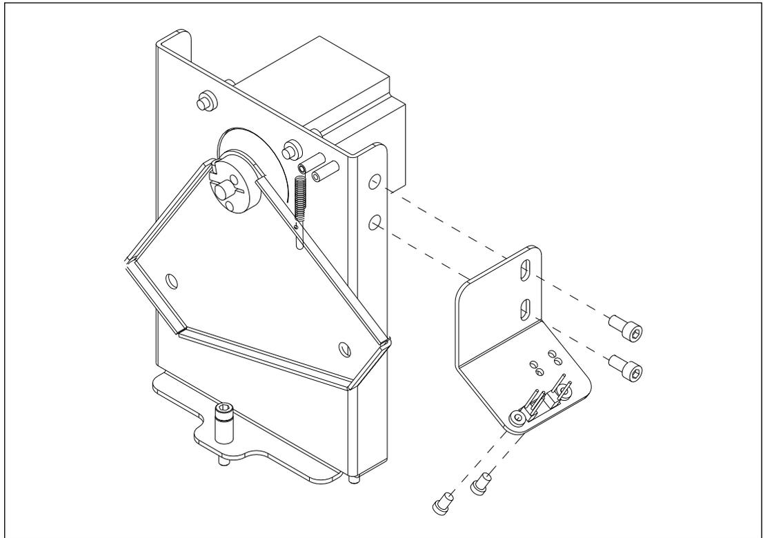
Figure 9-47. Shutter Home Sensor Mounting.
