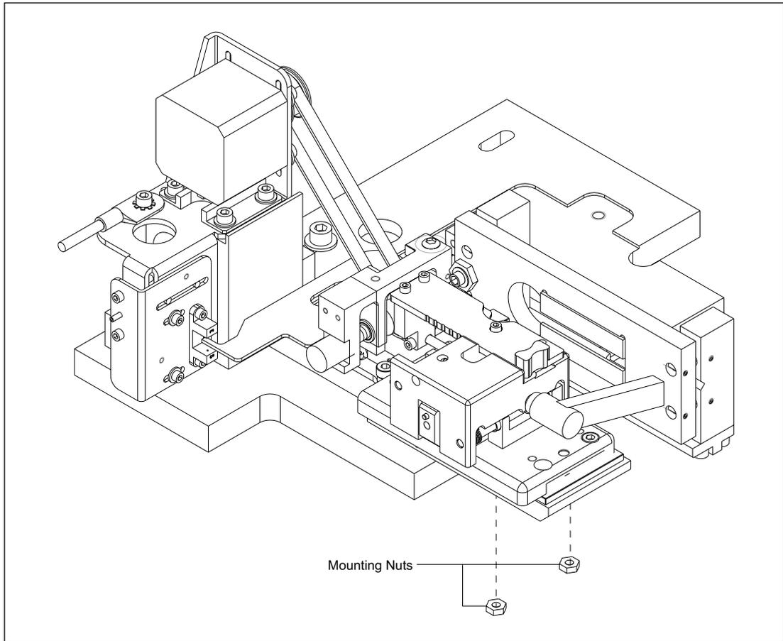
Figure 9-59. Capillary Mount Assembly Mounting.
