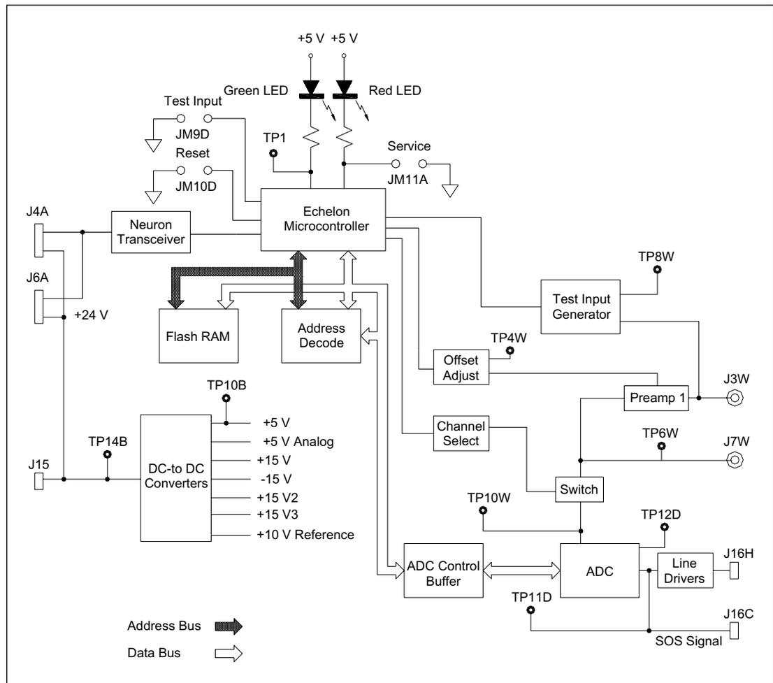
Figure 5-54. PDIO Board Block Diagram.
