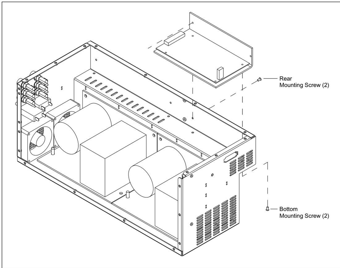
Figure 9-13. Internal Computer Power Supply Mounting.
