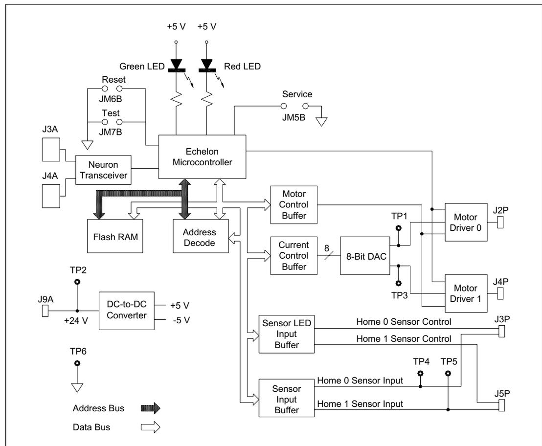
Figure 5-28. FLTR Board Block Diagram.
