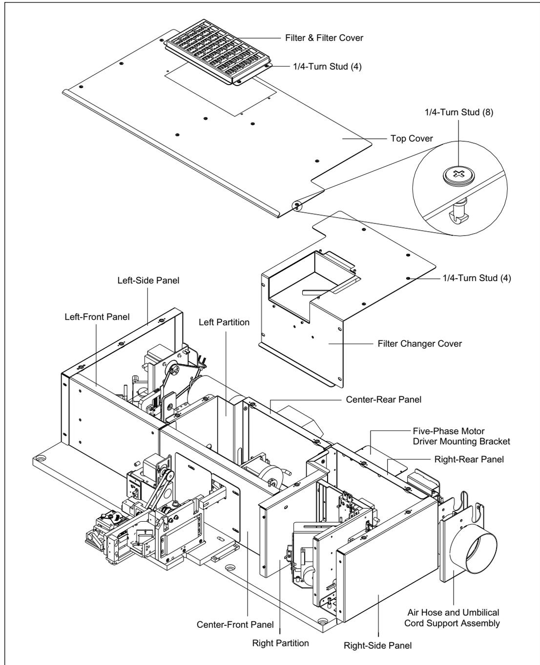
Figure 4-15. Optics Enclosure Assembly.
