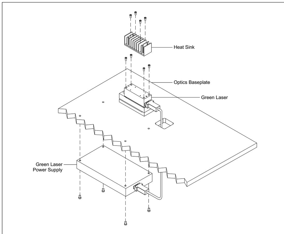
Figure 9-44. Green Laser and Power Supply Mounting.
