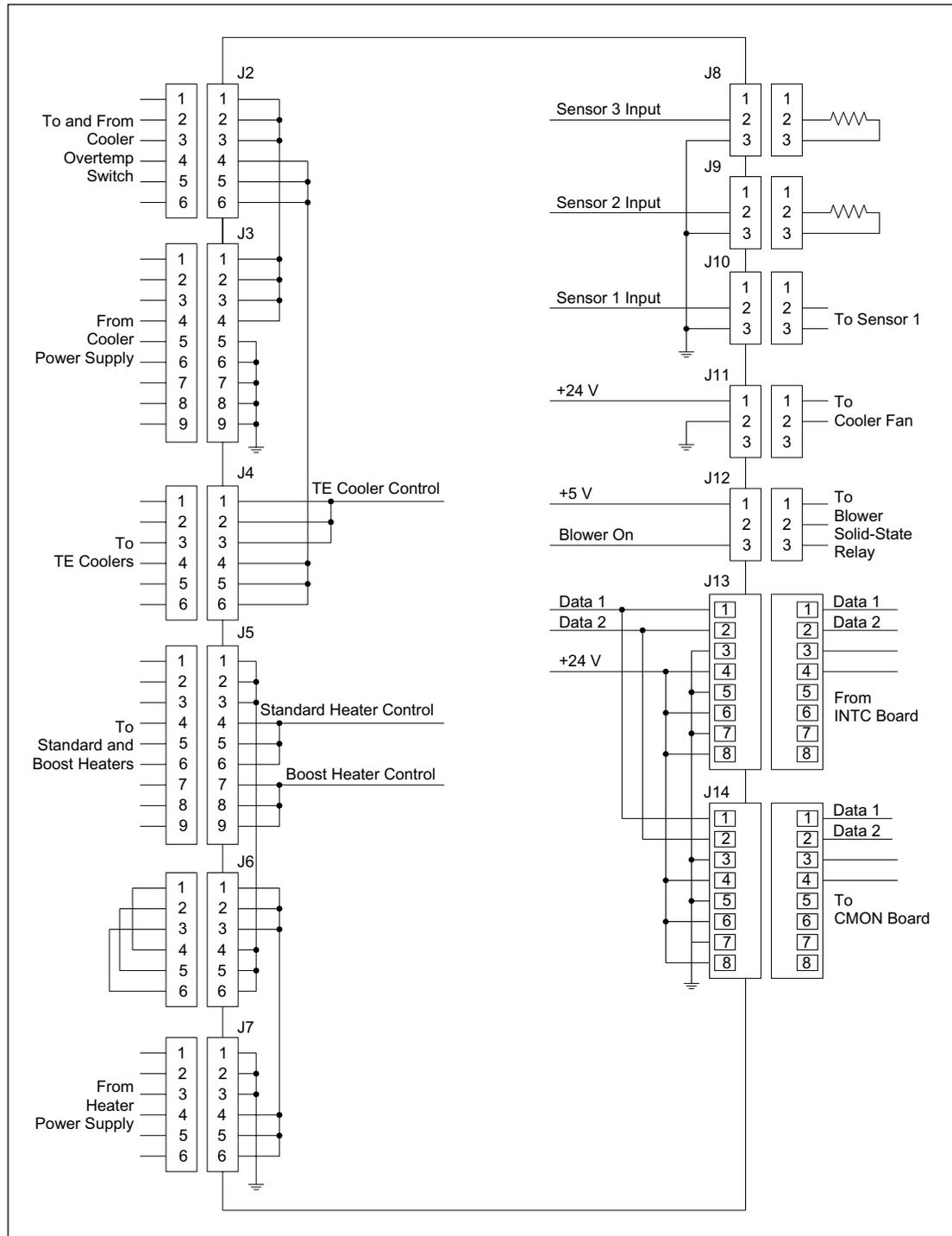
Figure 5-47. TMPR Board Connector Detail Diagram.
