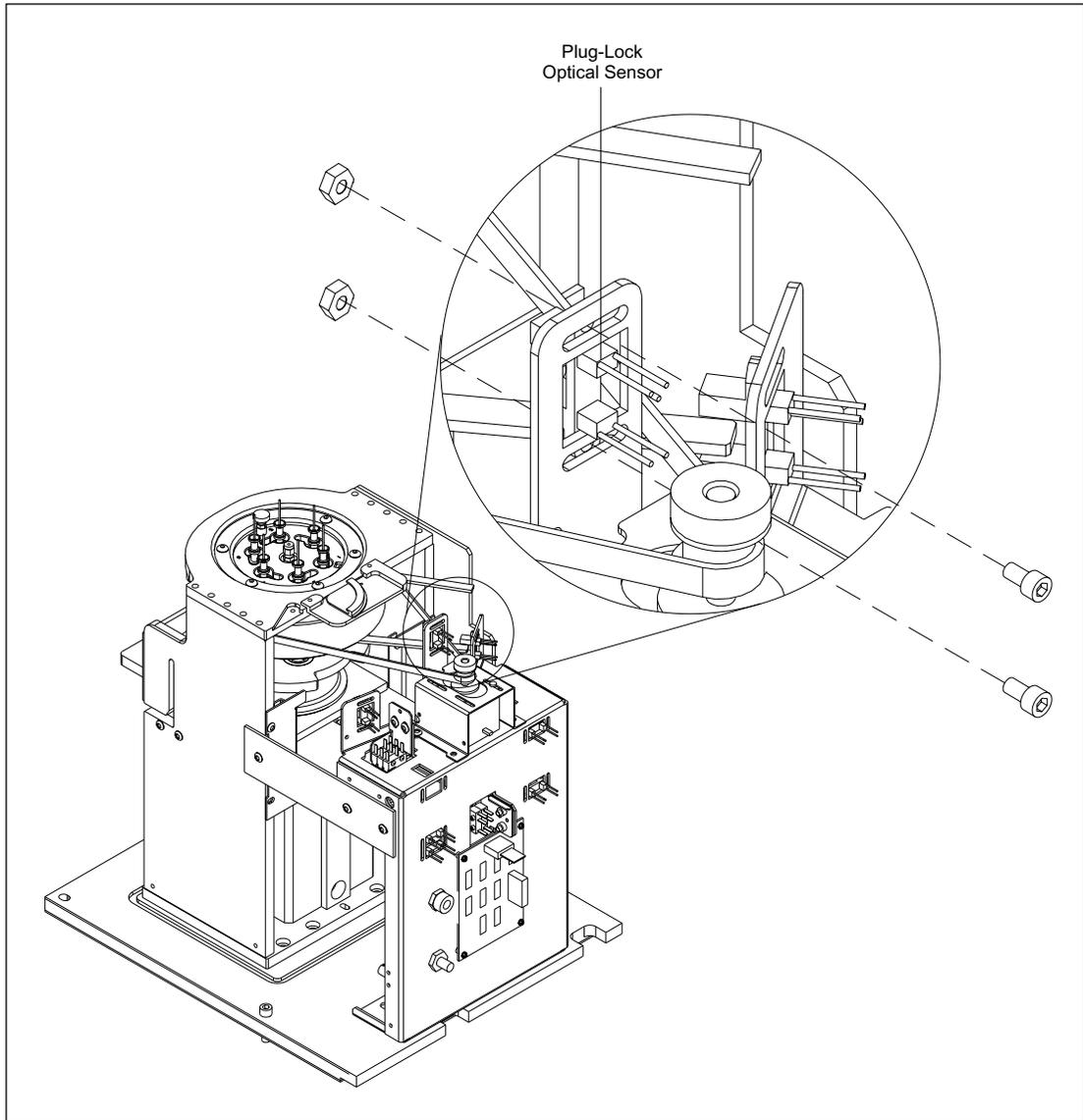
Figure 9-88. Anode Plug-Lock Optical Sensor Mounting.
