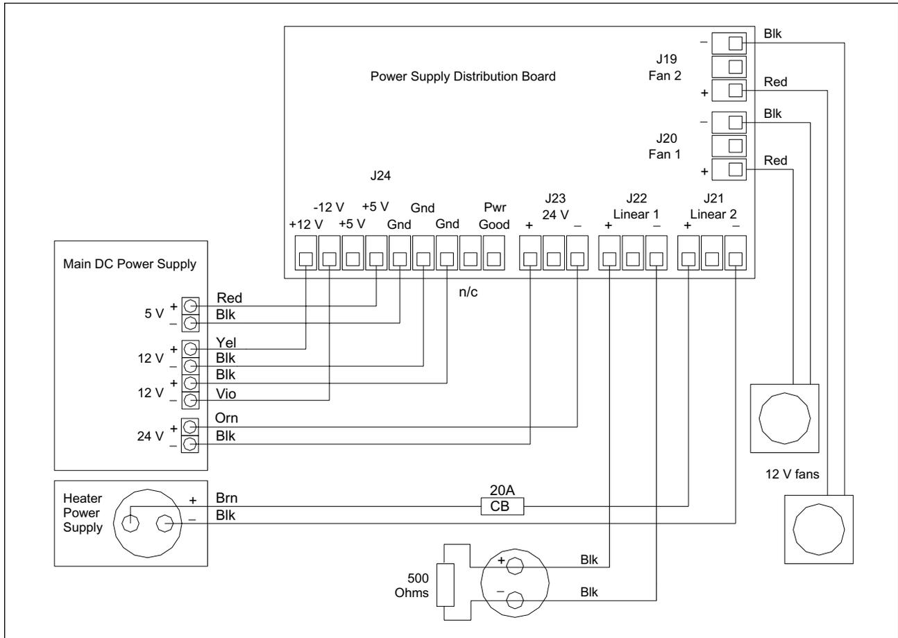
Figure 5-9. Power Supply Box DC Distribution Block Diagram (Two-Supply Model).
