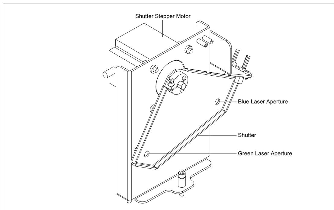
Figure 3-12. Three-Position Shutter.
