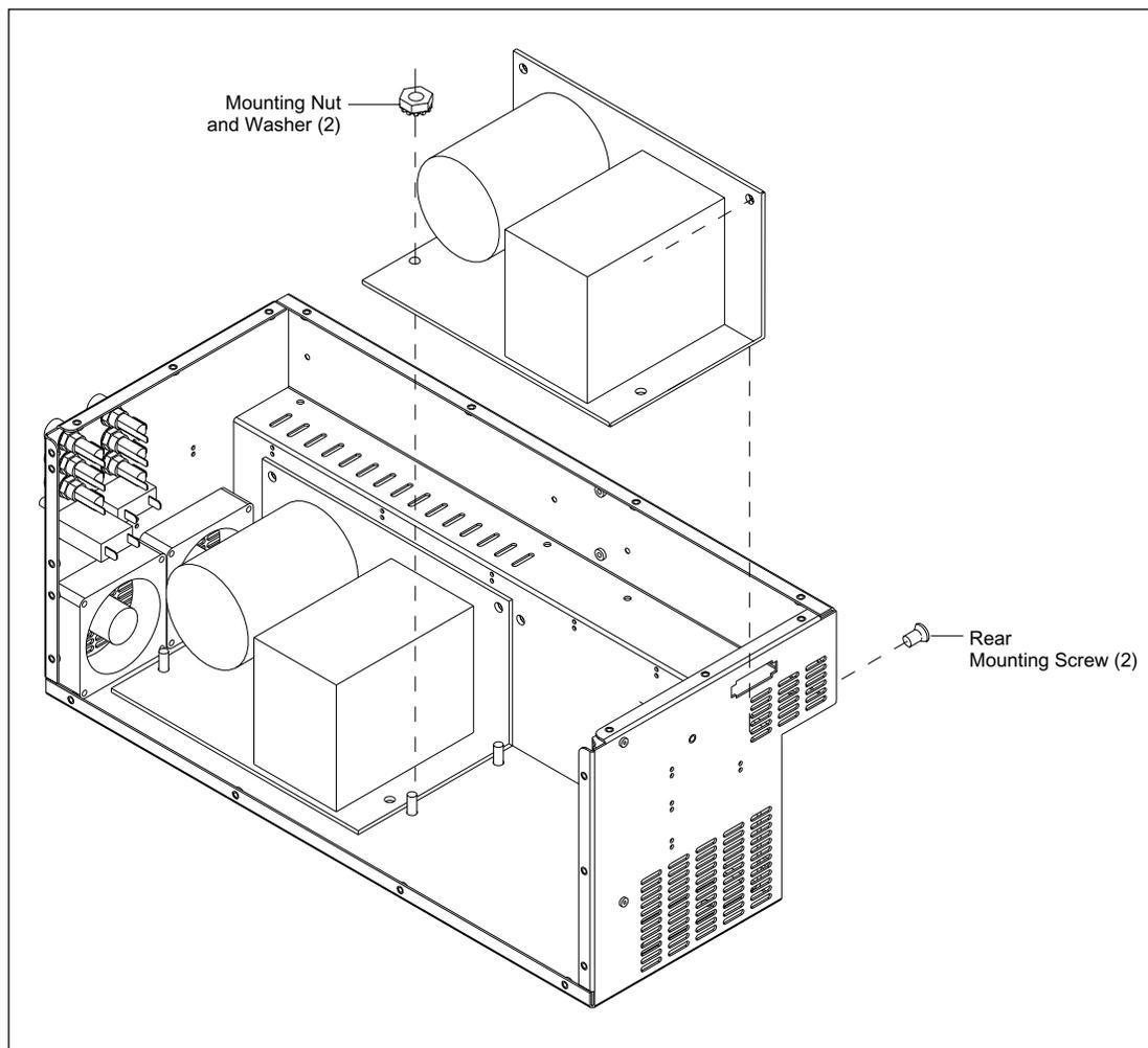
Figure 9-16. Heater Power Supply Mounting (Four-Supply Model).
