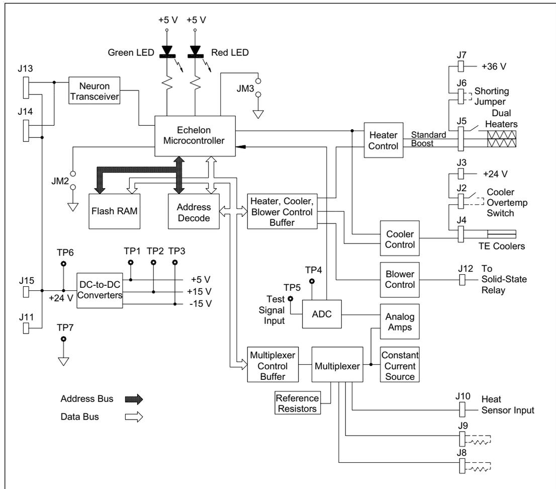
Figure 5-45. TMPR Board Block Diagram.
