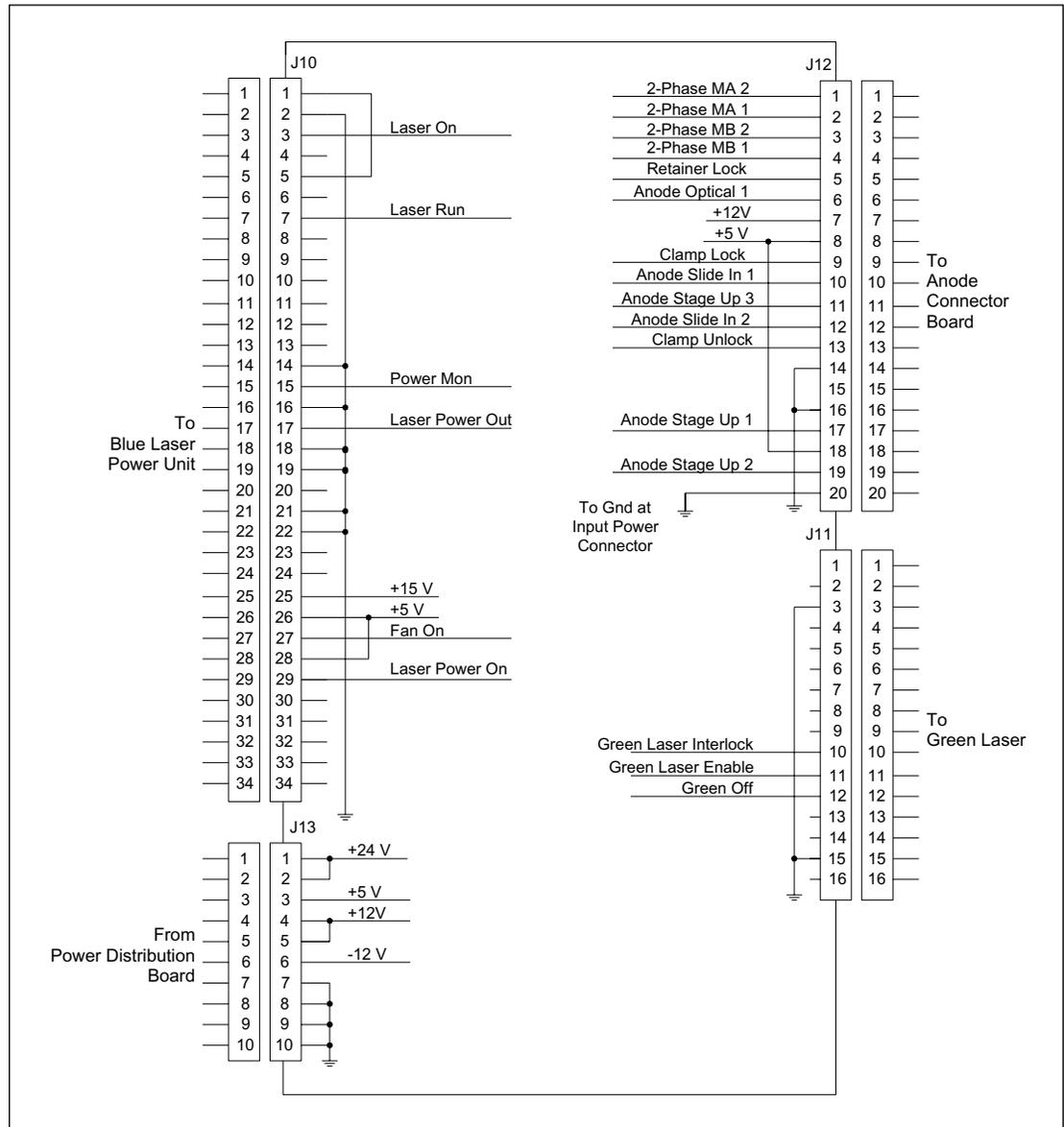
Figure 5-41. INTC Board Connector Detail Diagram (Sheet 3 of 3).
