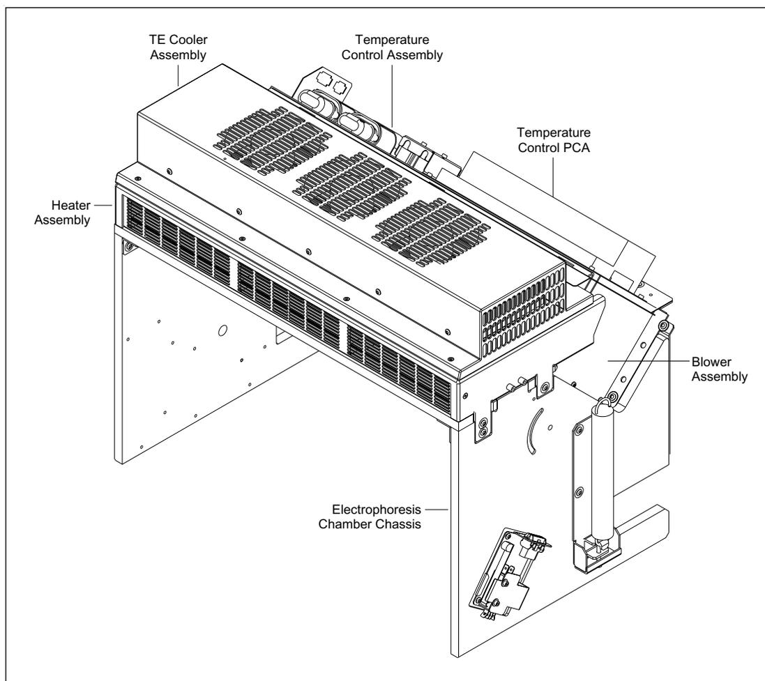
Figure 4-40. Temperature Control System.
