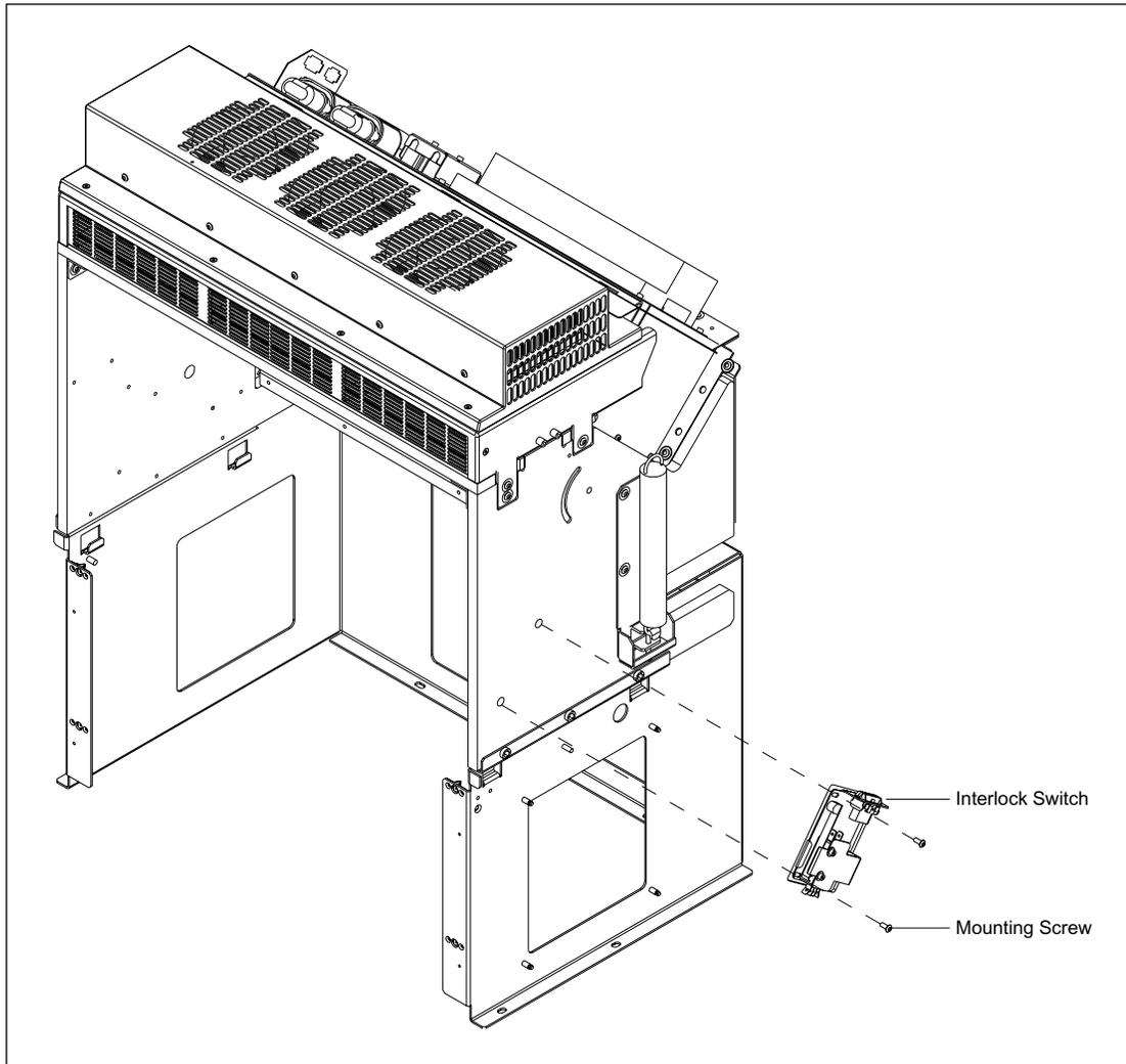
Figure 9-26. Service Door Interlock Switch Mounting.
