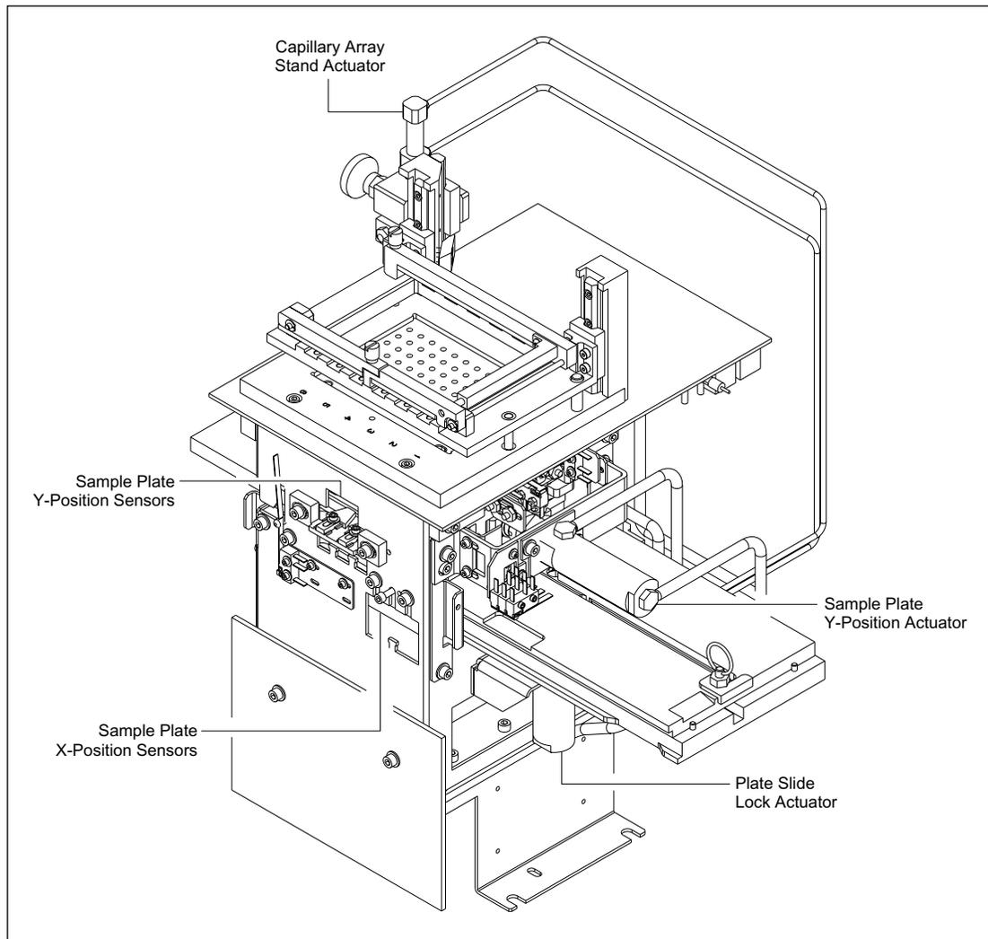
Figure 4-48. Cathode Assembly (MB 2000) (Left Rear).
