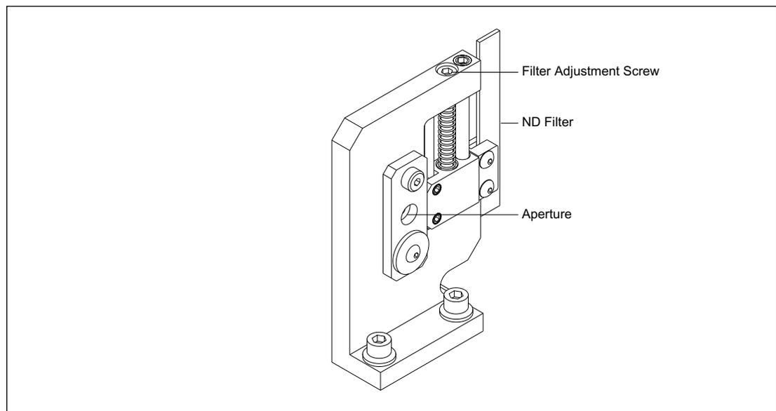
Figure 4-22. Green Laser ND Filter Assembly.
