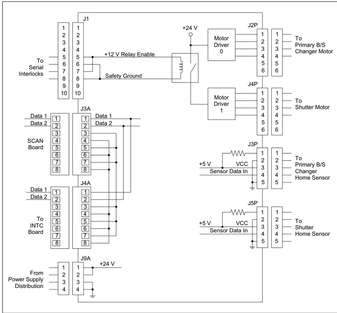
Figure 5-36. BEAM Board Connector Detail Diagram.
