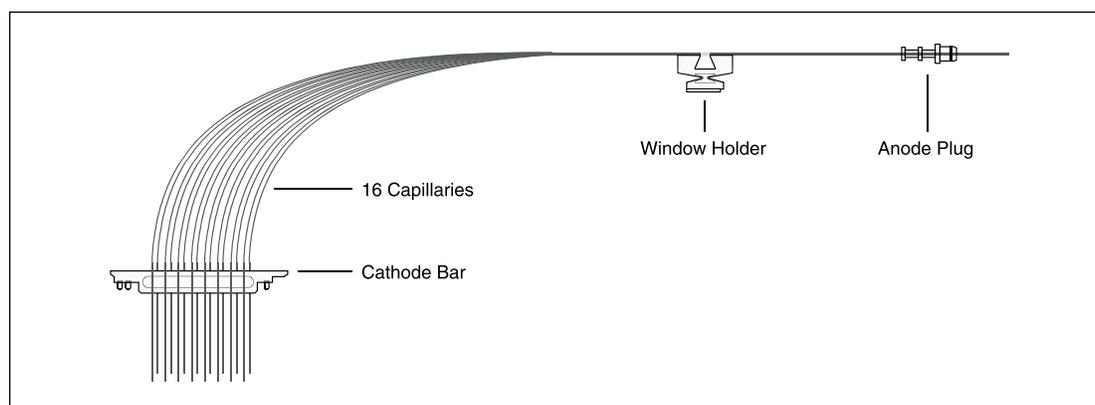
Figure 3-4. Capillary Array Components.
