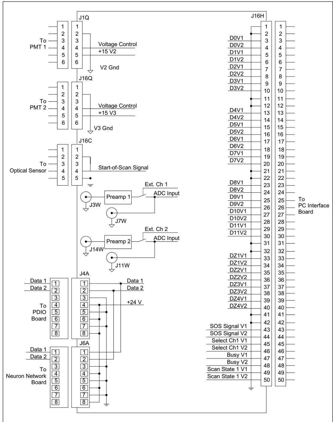
Figure 5-53. ADAQ Board Connector Detail Diagram.
