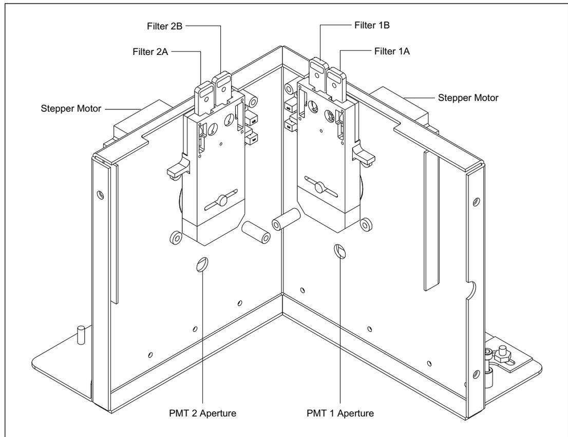
Figure 4-37. Filter Changer Assembly.
