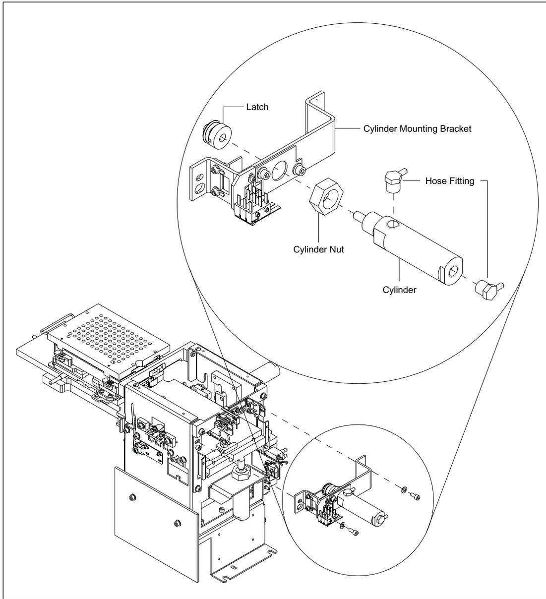
Figure 9-77. Indexer Y-Position Actuator Mounting (MB 2000).
