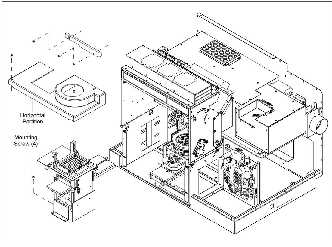
Figure 9-67. Cathode Assembly Mounting.
