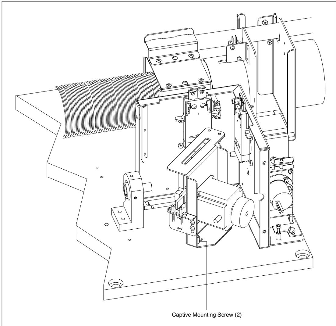
Figure 9-60. Secondary Beamsplitter Assembly Mounting.
