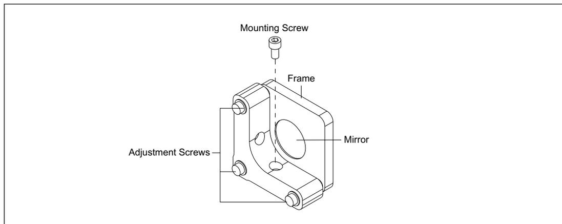
Figure 4-25. Mirror/Beam Combiner Assembly.
