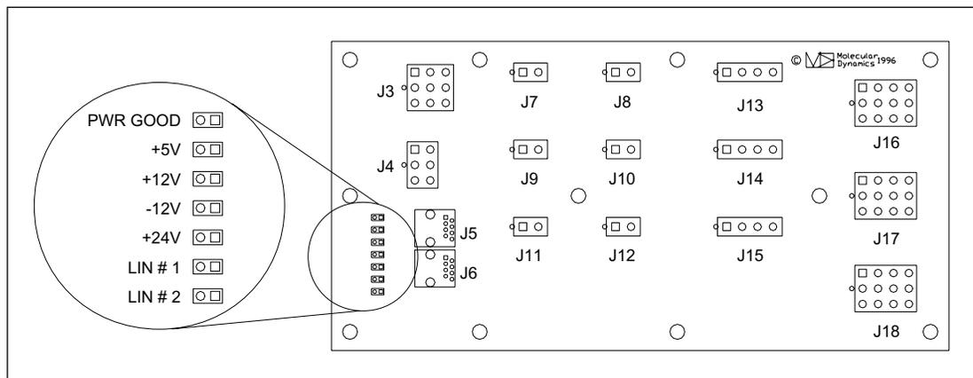
Figure 5-12. Power Supply Distribution Board Output Connections.
