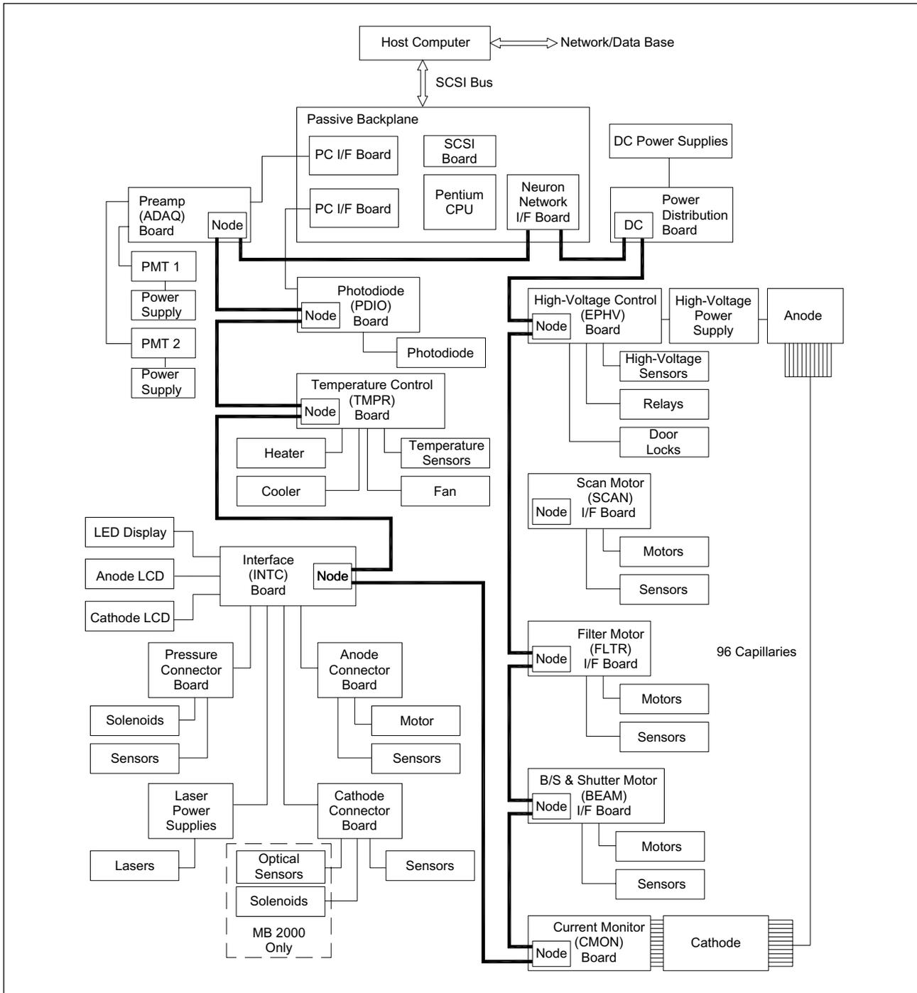
Figure 2-5. Electronics, Simplified Block Diagram.
