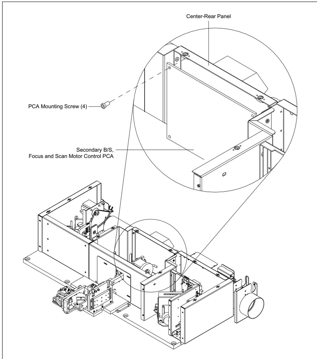
Figure 9-40. SCAN Board Mounting.
