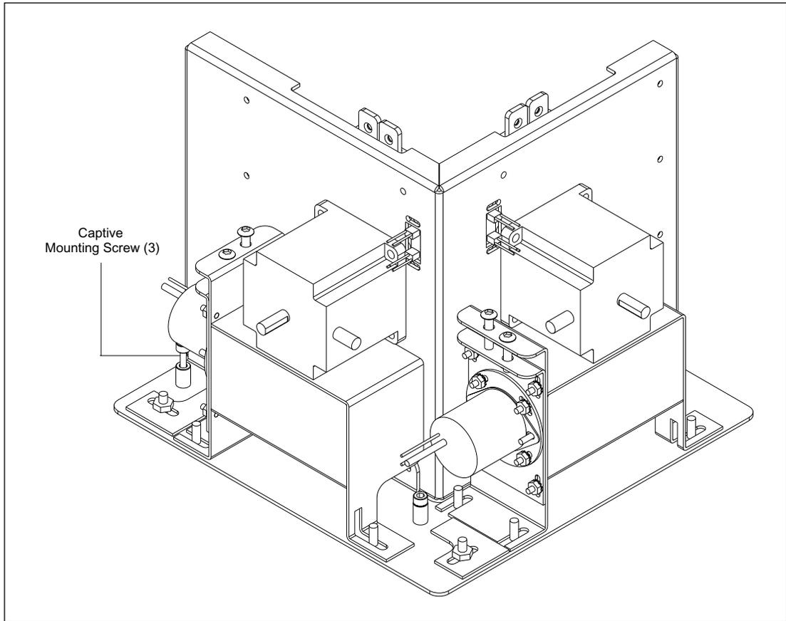
Figure 9-63. Filter Changer Assembly Mounting.
