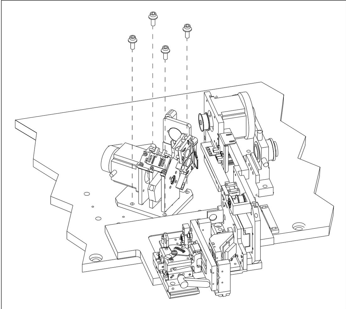
Figure 9-48. Primary Beamsplitter Changer Mounting.
