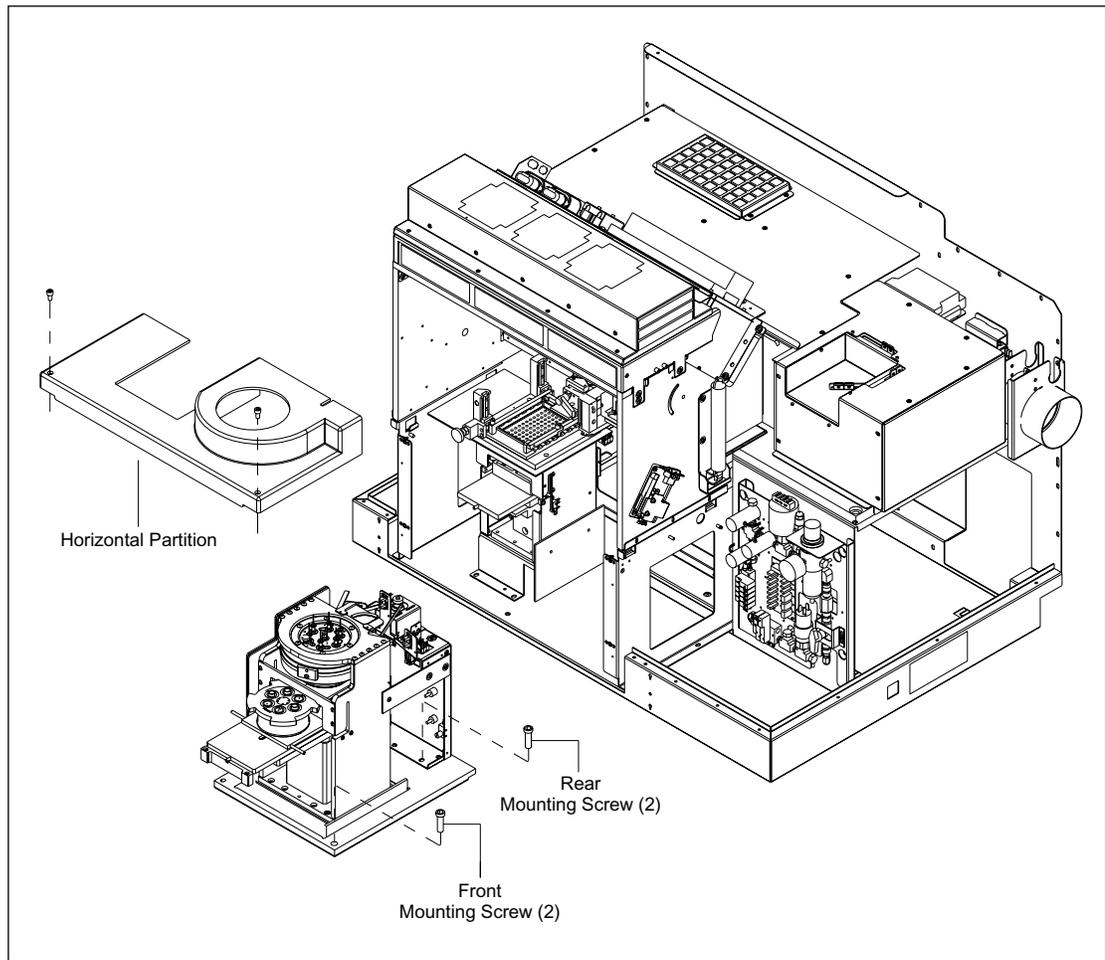
Figure 9-81. Anode Assembly Mounting.
