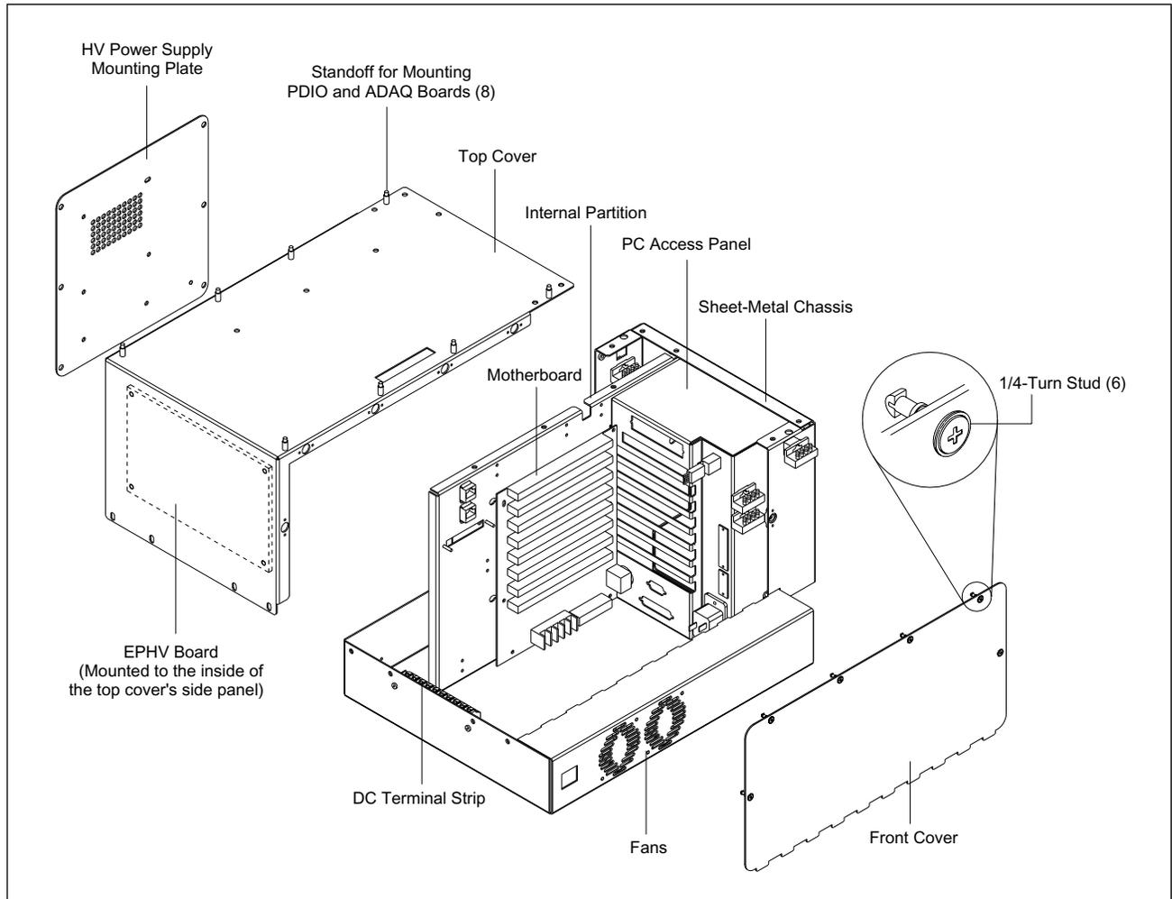
Figure 4-13. Internal Computer Enclosure.
