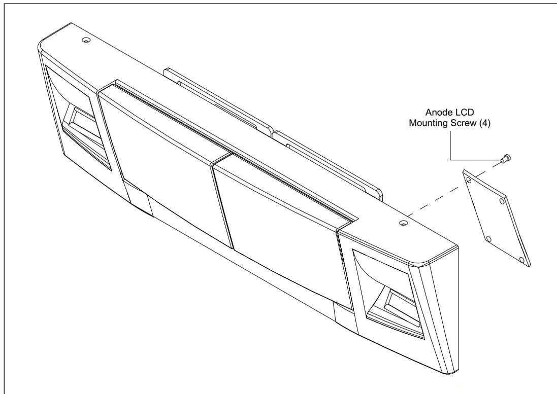
Figure 9-8. Anode LCD Board Mounting.
