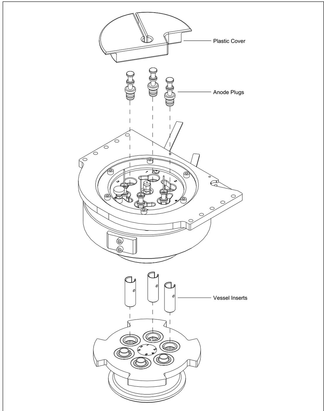
Figure 4-54. Anode Assembly, Simplified View (MB 500).
