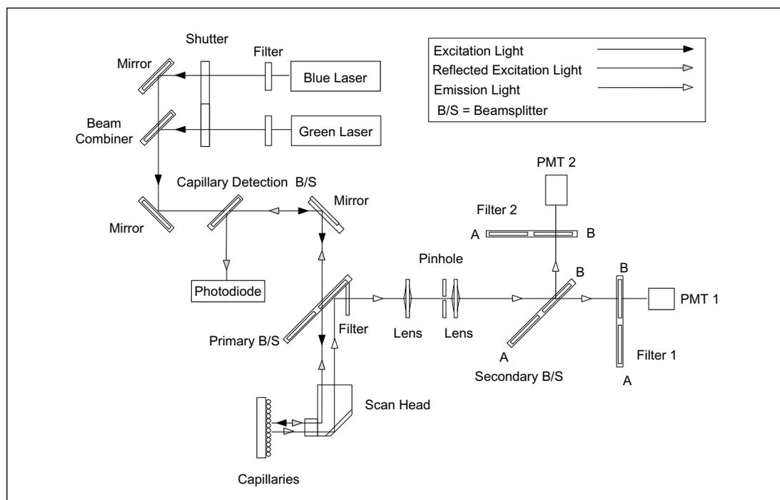
Figure 3-2. Excitation and Emission Paths, Functional Block Diagram.
