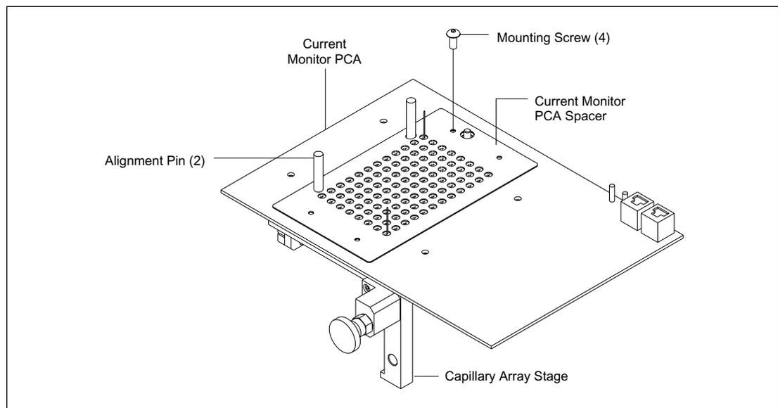
Figure 8-15. Capillary Array Stage.
