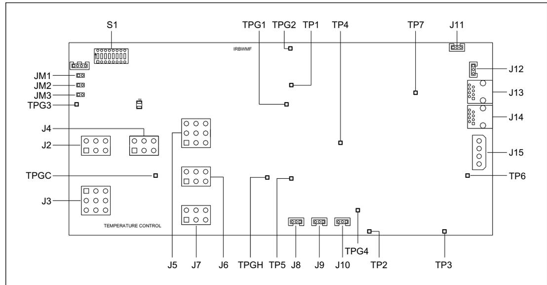
Figure 5-46. TMPR Board Component Layout Diagram.
