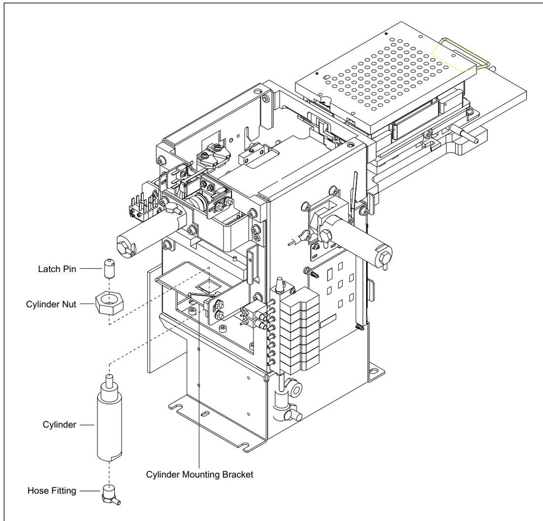
Figure 9-80. Slide Assembly Lock Actuator Mounting (MB 2000).
