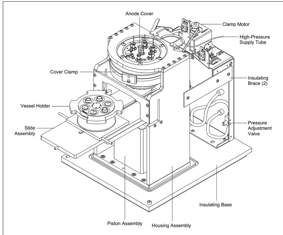
Figure 4-49. Anode Assembly.
