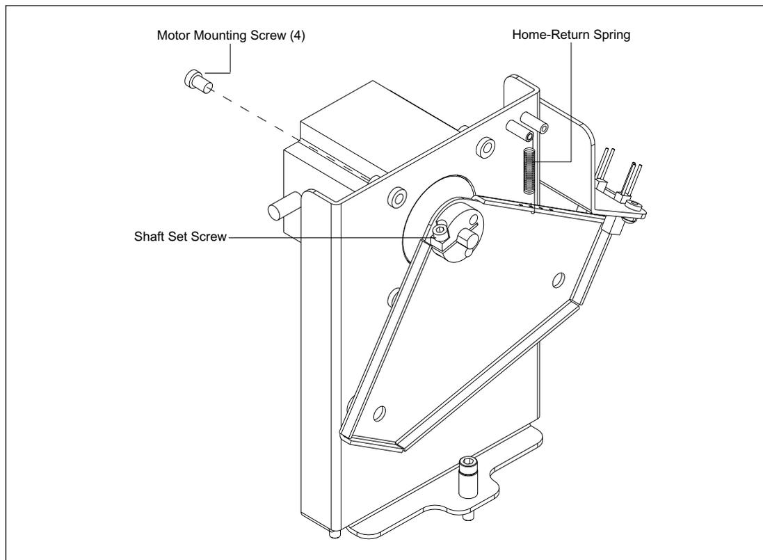
Figure 9-46. Shutter Drive Motor Mounting.
