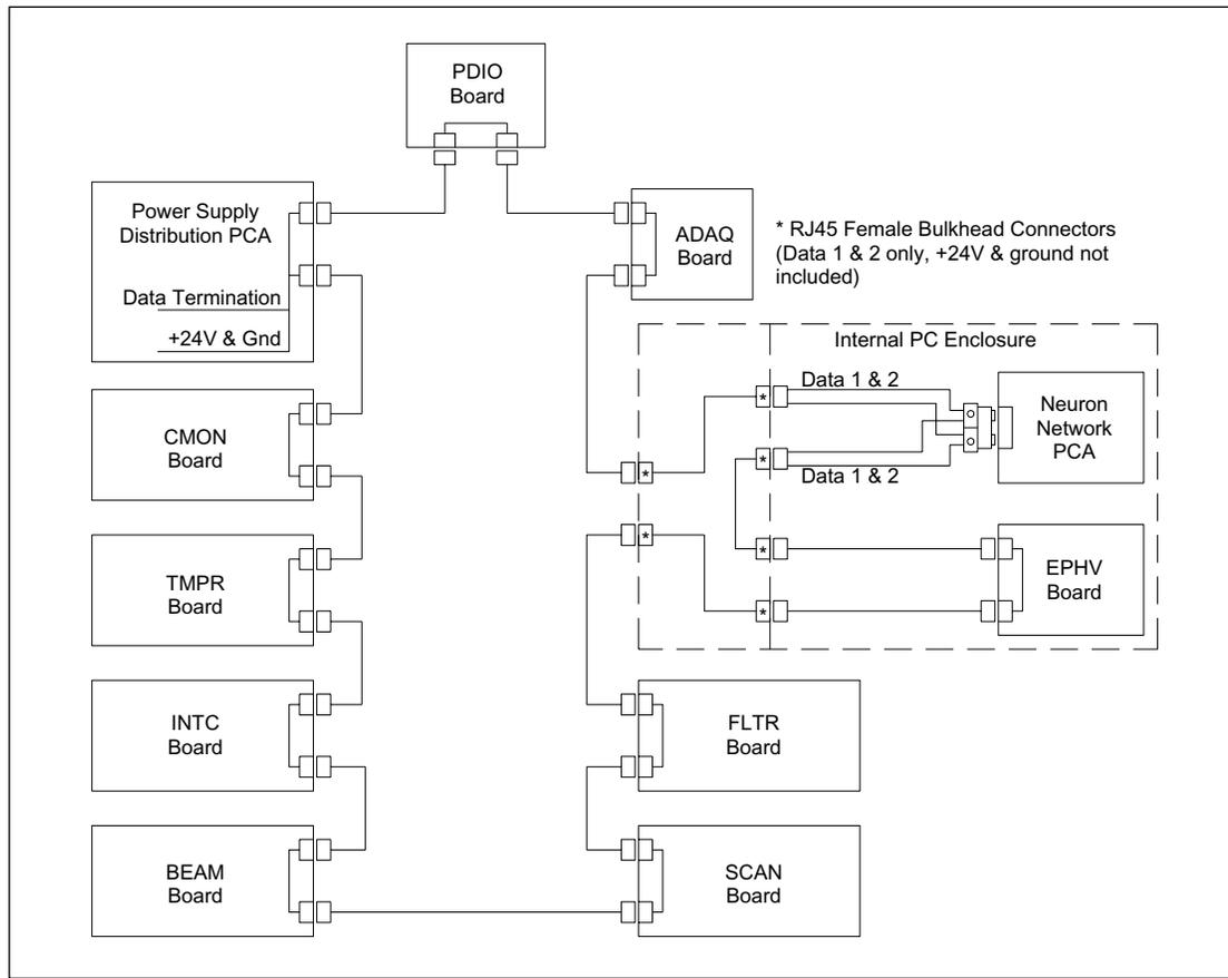
Figure 5-14. Neuron Network Signal and DC Distribution Block Diagram.
