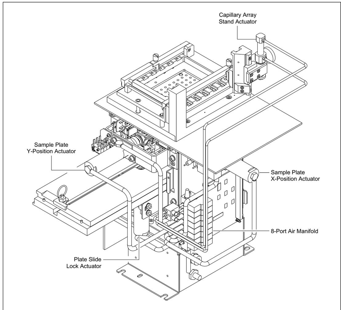
Figure 4-47. Cathode Assembly (MB 2000) (Right Rear).
