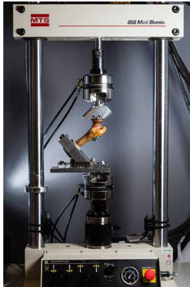
Photograph of a human cadaveric femur with a standardised osteotomy fixated with the Swemac Pinloc®.
